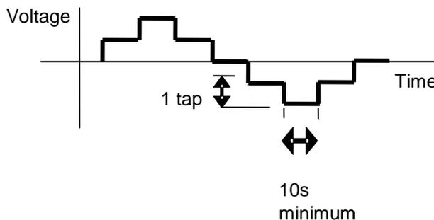
OC5.A.3.5 Figure 1 – Transformer tap sequence for voltage control tests
