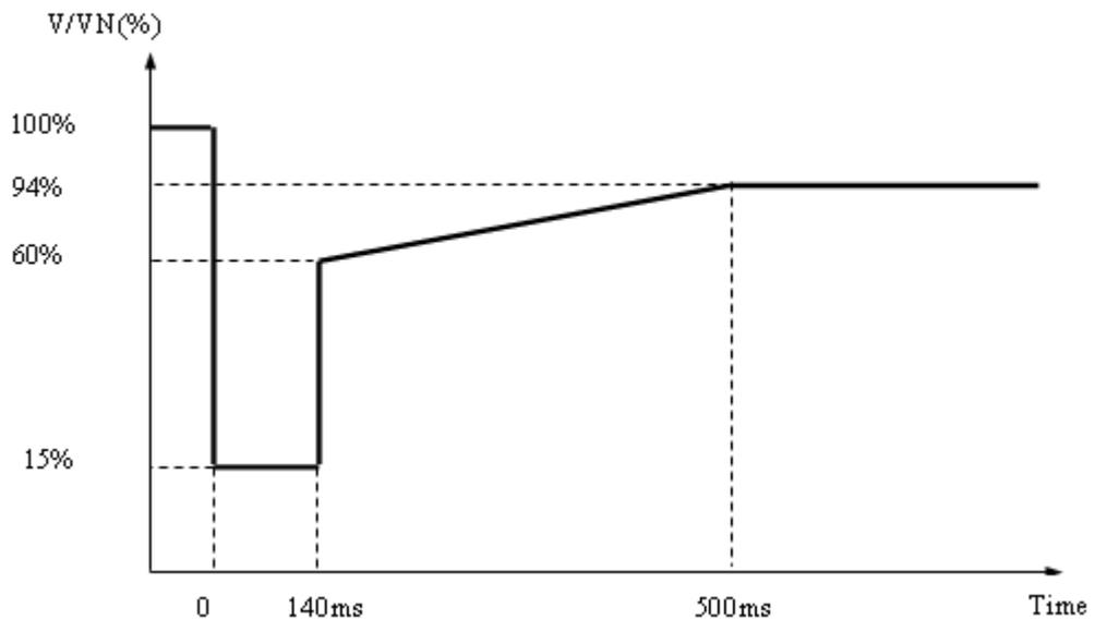
$V/V_N$  is the ratio of the voltage at the **LV side of the Offshore Platform** to the nominal voltage of the LV side of the **Offshore Platform**.
