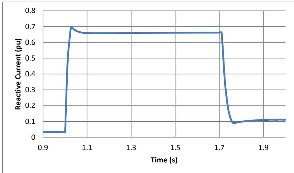
Figure ECC4.5 Reactive Current Injected for a 50% voltage dip for a period of 710ms
