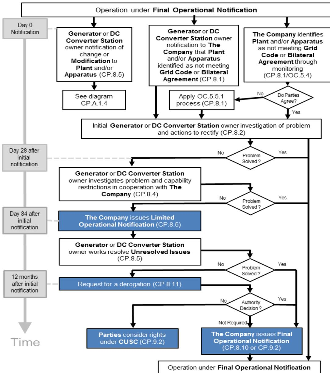
This diagram illustrates the process in the CP and includes references in brackets to specific Grid Code clauses. For the avoidance of doubt this process does not apply to **Embedded Medium Power Stations** not subject to a **Bilateral Agreement** and **Embedded DC Converter Stations** not subject to a **Bilateral Agreement**.
