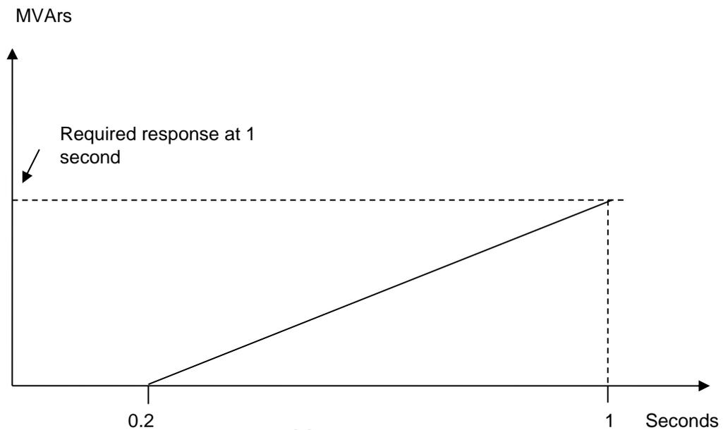
CC.A.7.2.3.2 An **Onshore Non-Synchronous Generating Unit, Onshore DC Converter, OTSDUW Plant and Apparatus** or **Onshore Power Park Module** installed on or after 1 December 2017 shall be capable of;
