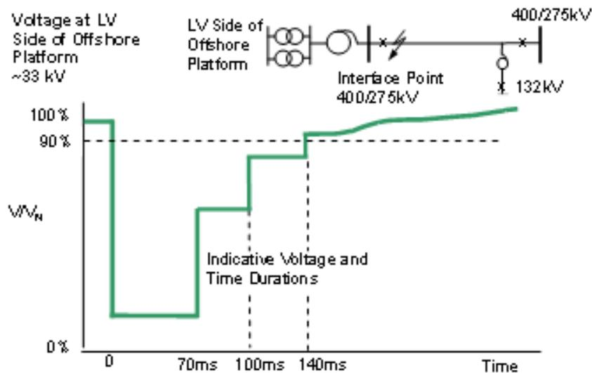
Typical fault cleared in 140ms:- 3 ended circuit
