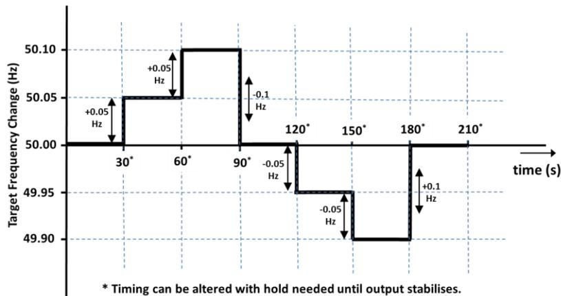
OC5.A.3.6. Figure 3 – Target Frequency setting changes
