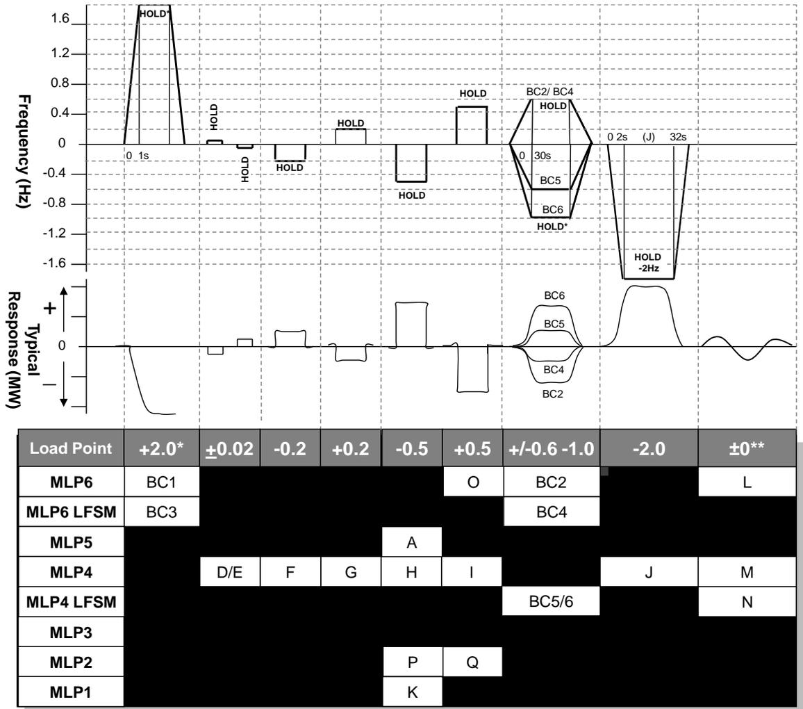
ECP.A.6.6. Figure 2 – Frequency Response Capability LFSM-O, LFSM-U, FSM Step Response tests
