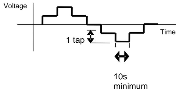
ECP.A.7.4 Figure 1 – Transformer tap sequence for voltage control tests
