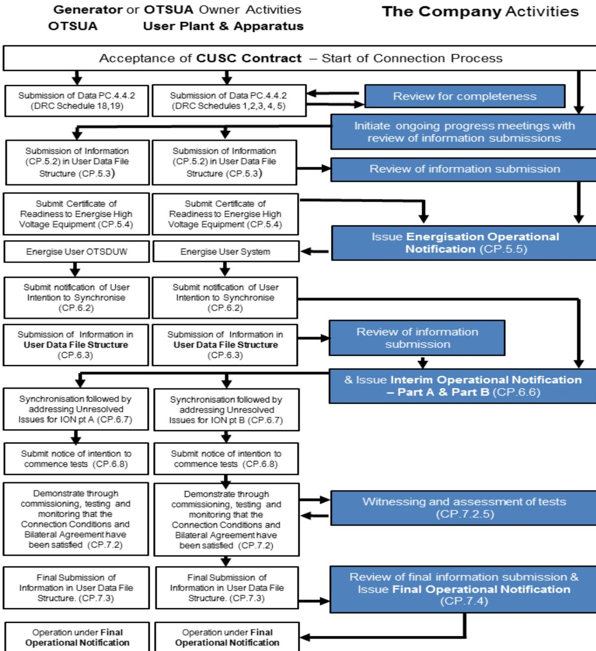
This diagram illustrates the process in the **CP** and includes references in brackets to specific Grid Code clauses.
