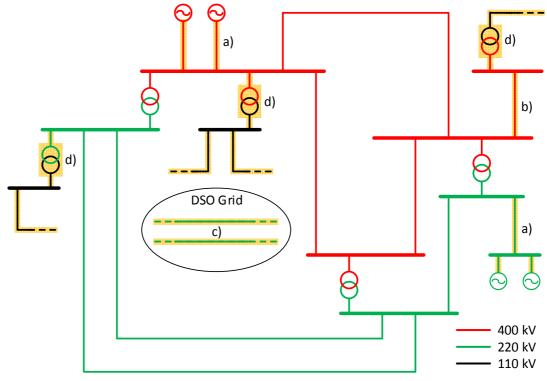
Figure 2: Elements (highlighted in yellow) which can be discarded from the set of Channel XNEs
