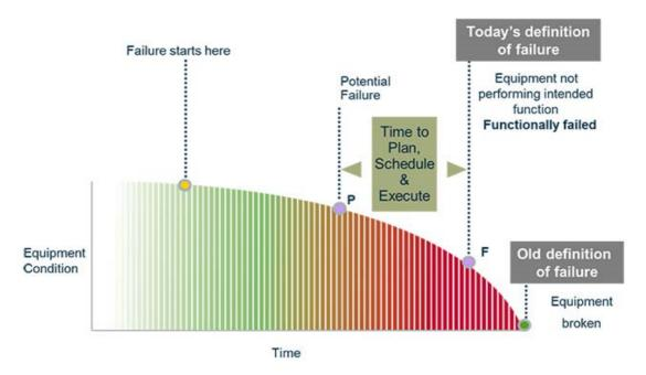
Figure 97 - Equipment condition and relationship to failure over time
