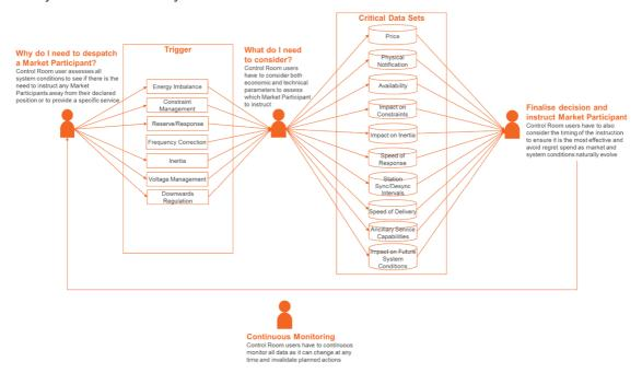
Figure 19 – High-level decision process for control centre engineers
