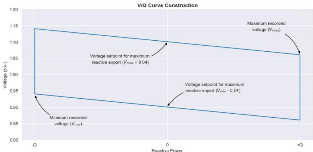
Figure 20: An example V/Q curve
