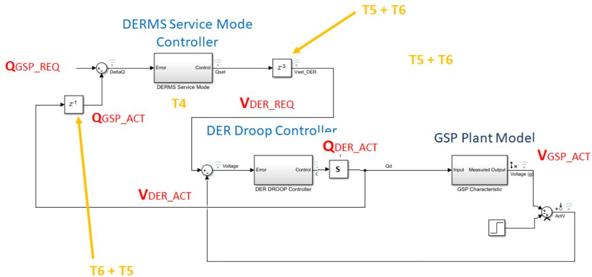
Figure 15: DERMS Q service mode control system view (2/2).
