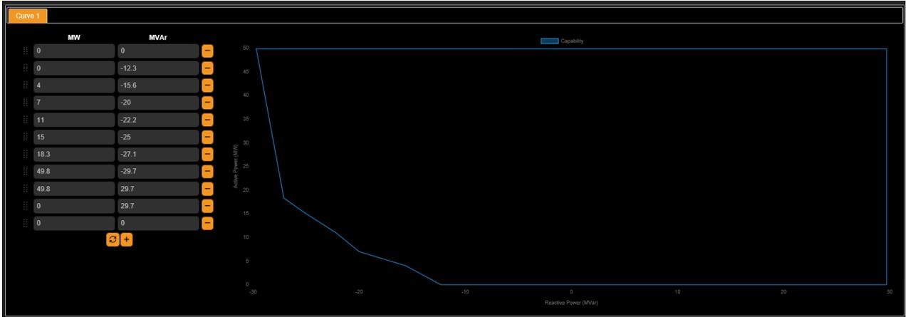
Figure 40: Simplistic DER PQ technical capability curve
