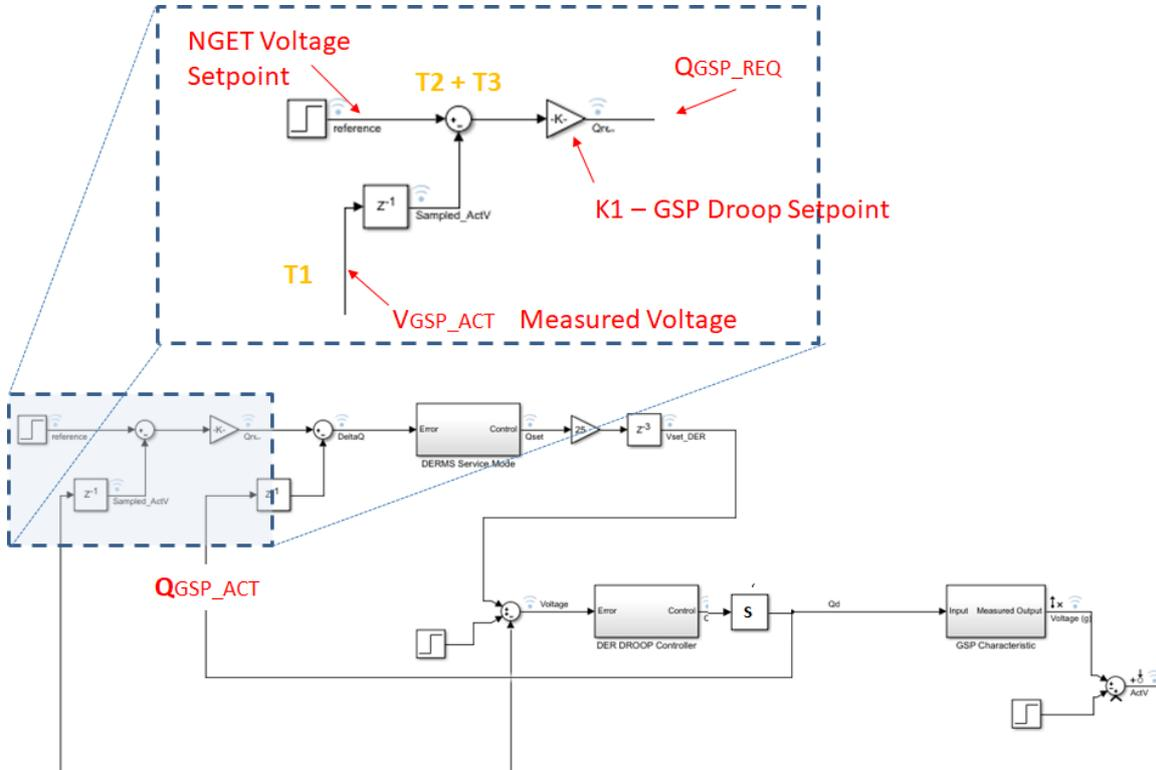
Figure 14: DERMS Q service mode control system (view 1/2).
