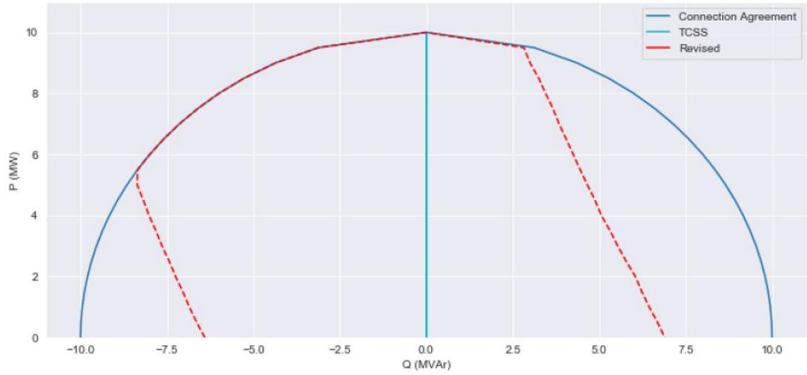
Figure 21: An example PQ capability curve
