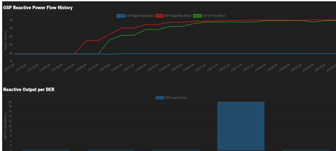
Figure 16: Example of stable testing result. One DER available: Q actual tracks (green) Q requested (red) for the following instruction: voltage set point of 405kV, dead-band = 2kV, 4% drop.
