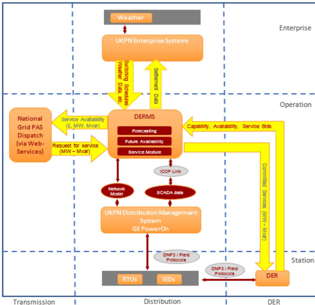
Figure 5: Solution data flow diagram
