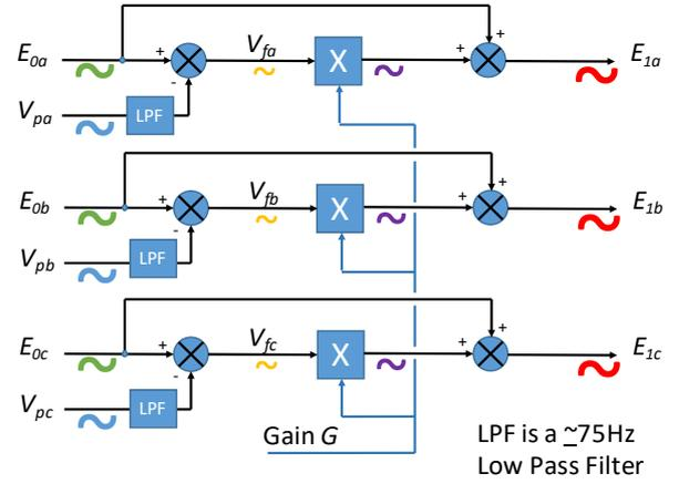
Fig. 6. Convertor and EMT Implementation of Impedance Reduction Algorithm
