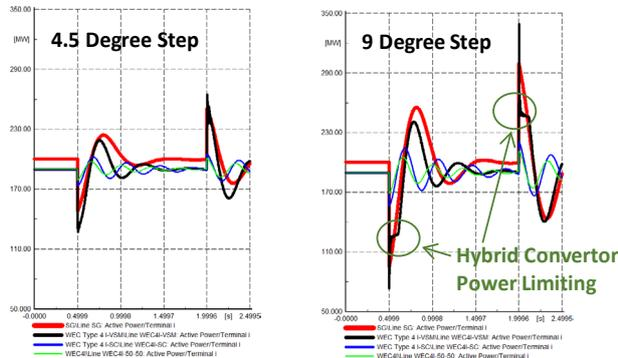
Fig. 8. Vector Shift Results with X Reduction Algorithm gain set to 1 (X reduction on and impedance halved)
