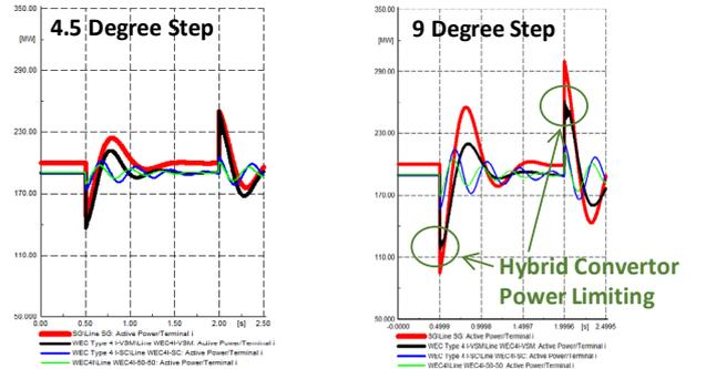
Fig. 7. Vector Shift Results with X Reduction Algorithm gain set to 0 (X Reduction switched off)
