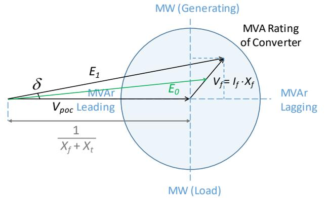
Fig. 4. Vector Diagram for modified relationship between Voltages
