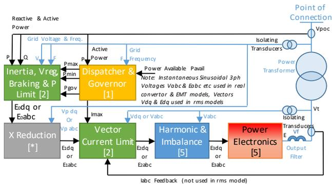
Fig. 1. Simplified Block Diagram of potential VSM Implementation
