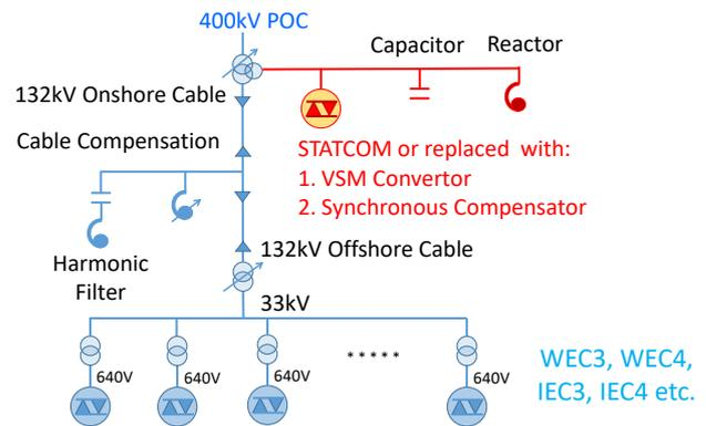
Fig. 2. Single Line Diagram (SLD) of a model for a typical OFTO
