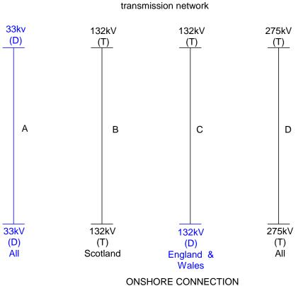
ONSHORE CONNECTION 132/275/400kV circuits are part of GB Transmission network in Scotland Only 275/400 circuits are part of GB Transmission network in England & Wales
