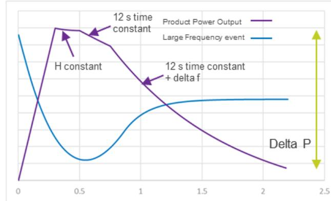
Swing equation relationship to determine additional active power to allow  $df/dt$  of upto 1 Hz/s
