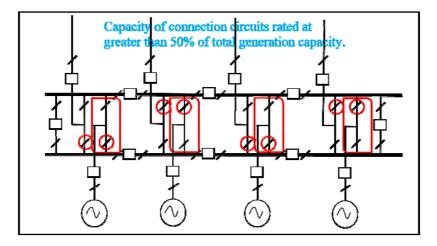
Figure 10: Alternative Method 9 - Firm Connection, 4 circuits, multmesh arrangement
