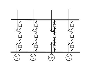
A.6.7.11 Firm connection, 4 circuits, Multi-mesh arrangement
