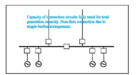
Figure 5: Method 5, Non-firm, two fully rated circuits
