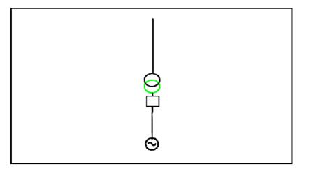
The simplest connection method is considered appropriate for smaller developments and enables a direct transmission connection while retaining a sub-transmission connection voltage.
