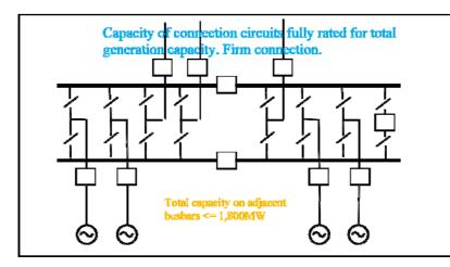
Other alternative configurations are possible such as an additional bus-coupler on the left hand side with the replacement of the bus-section circuit breaker on the reserve busbar by disconnectors. This provides similar functionality but improved operational flexibility.
