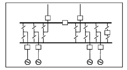
Connection method 7 is an incremental development of method 6 with the addition of a single bus section circuit breaker. This method also provides a 'firm' connection for the associated generation with additional resilience. The arrangements can be summarised:
