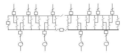
A.7.7.4 Eight circuit marshalling Substation, Wrap-Around busbar
