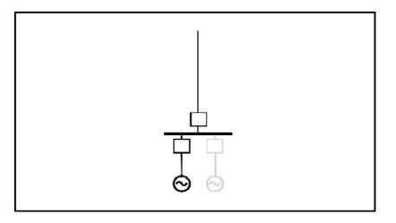
This connection method is considered appropriate for larger developments or groups of developments and enables a direct transmission connection at a transmission voltage.
