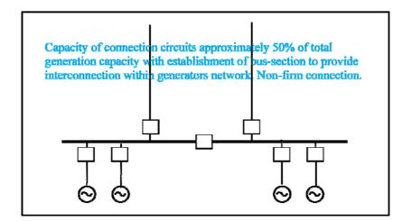
Figure 4: Method 4 - Non-firm, two circuits of reduced capacity
