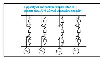
Figure 9: Method 9 – Firm connection, 4 circuits, 1½ switch layout
