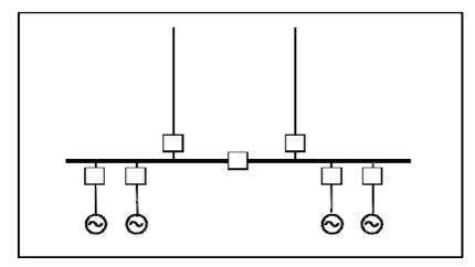
Connection method 5 is an incremental development of method 4 which provides system access to the entire group generation capacity during single circuit outages. The arrangements can be summarised:
