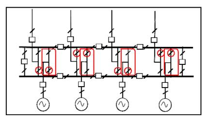
Connection method 9 is the most secure of the connection arrangements together with the addition of a fourth circuit.
