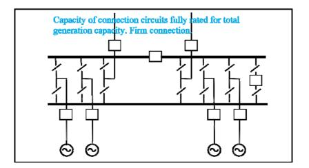
Figure 7: Method 7 - Firm connection, 2 circuits, three section double busbar
