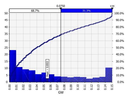
For interest, Figure 19 shows the *approximate* probability distribution for the output of this onshore Scottish windfarm for 150MW, 400MW and 800MW capacities. To derive a mean constrained off volume, we *could* 'sumproduct' the appropriate windfarm outputs and their associated probabilities from this table. Instead, we elect to use @Risk to do this for us with greater accuracy.
