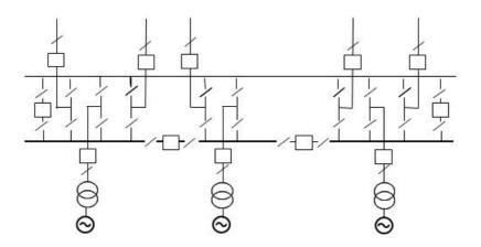
A.6.7.9 Firm connection, 3 circuits, four section double busbar
