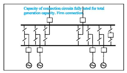
Figure 6: Method 6 - Firm connection, 2 circuits, two section double busbar
