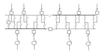
A.7.7.2 Six circuit marshalling Substation, double B'bar with physical split
