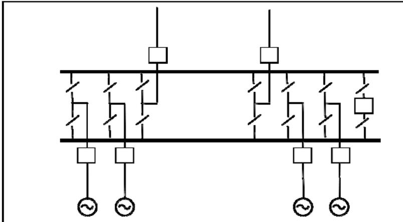
Connection method 6 is the simplest application of a double busbar switchgear layout providing a 'firm' connection for the associated generation. The arrangements can be summarised:
