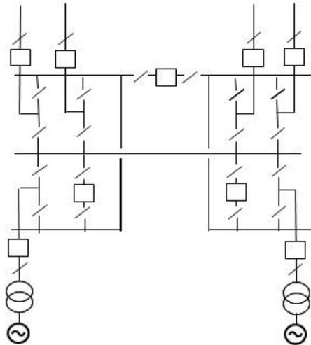
A.6.7.3 Firm connection, Two section wrap-around busbar, main b'bar central
