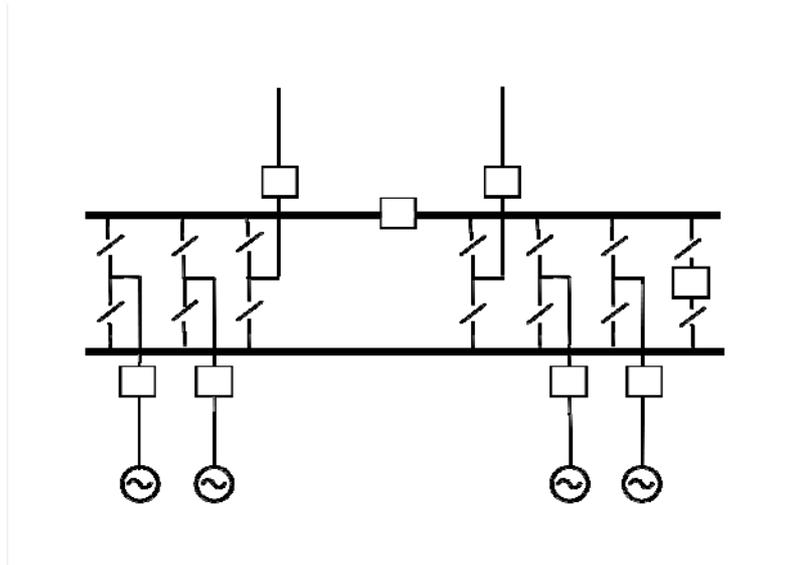
A.6.7.5 Firm connection, three section wrap-around busbar, main b'bar outside
