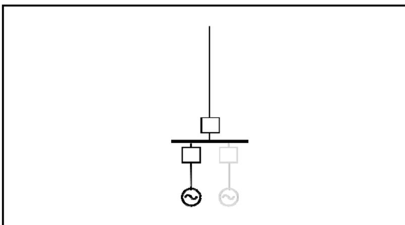
This connection method is considered appropriate for larger developments or groups of developments and enables a direct transmission connection at a transmission voltage.
