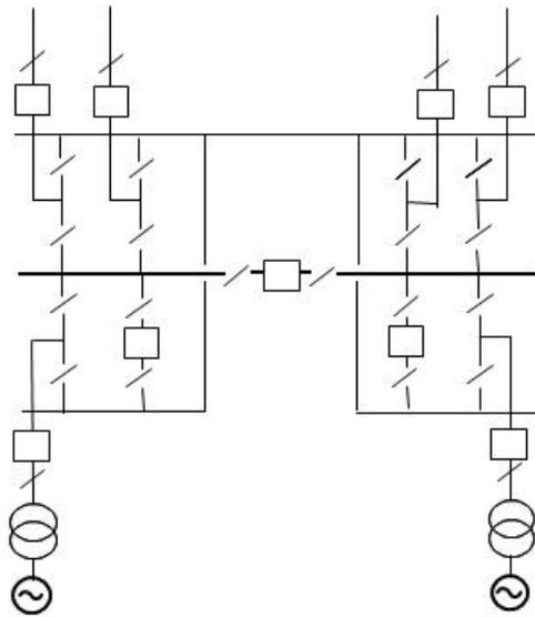
A.6.7.4 Firm connection, 2 circuits, three section double busbar
