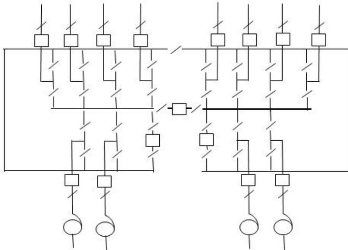
**A.7.7.5 Eight circuit marshalling Substation, double b'bar & physical split**
