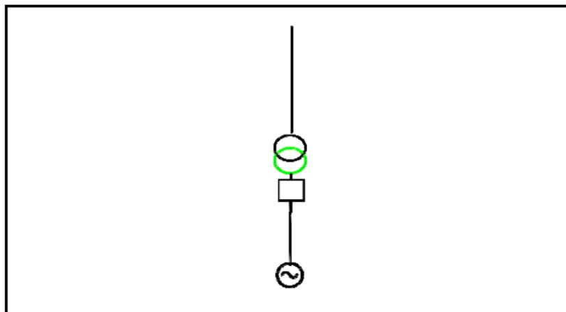
Figure 1: Method 1 - Single Circuit Radial, Sub-Transmission. Connection Voltage
