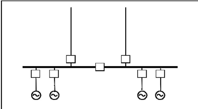
Connection method 5 is an incremental development of method 4 which provides system access to the entire group generation capacity during single circuit outages. The arrangements can be summarised:
