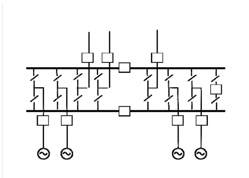
A.6.7.10 Firm connection, 4 circuits, 1½ switch layout busbar
