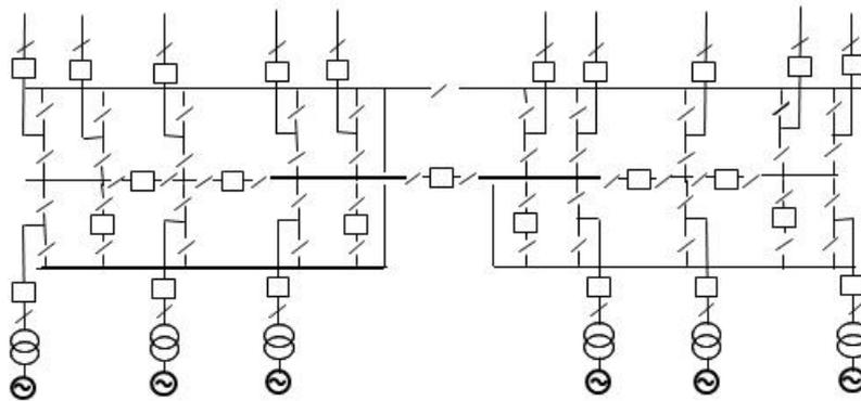
A.6.7.14 Firm connection, four section Double Busbar
