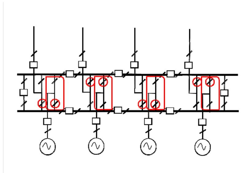
A.6.7.12 Firm connection, four section Wrap-Round Busbar, Outside Main
