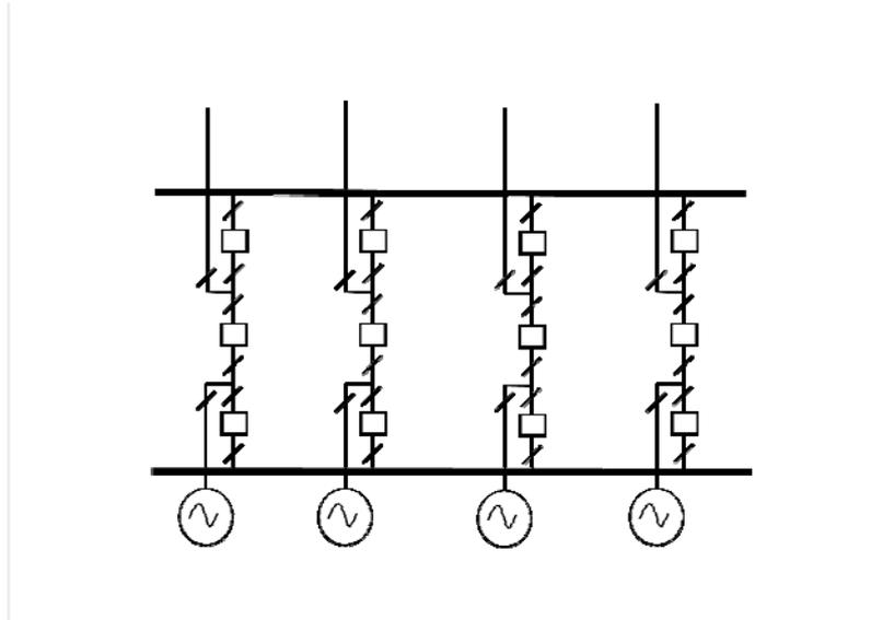
A.6.7.11 Firm connection, 4 circuits, Multi-mesh arrangement
