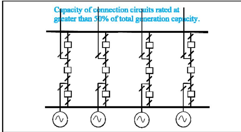
Figure 9: Method 9 – Firm connection, 4 circuits, 1/2 switch layout
