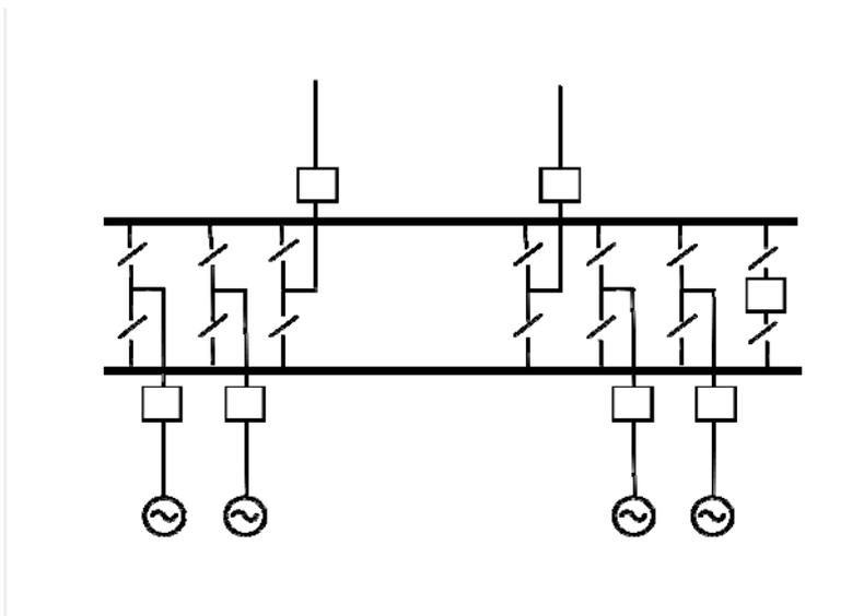
A.6.7.2 Firm connection, Two section wrap-around busbar, main b'bar outside
