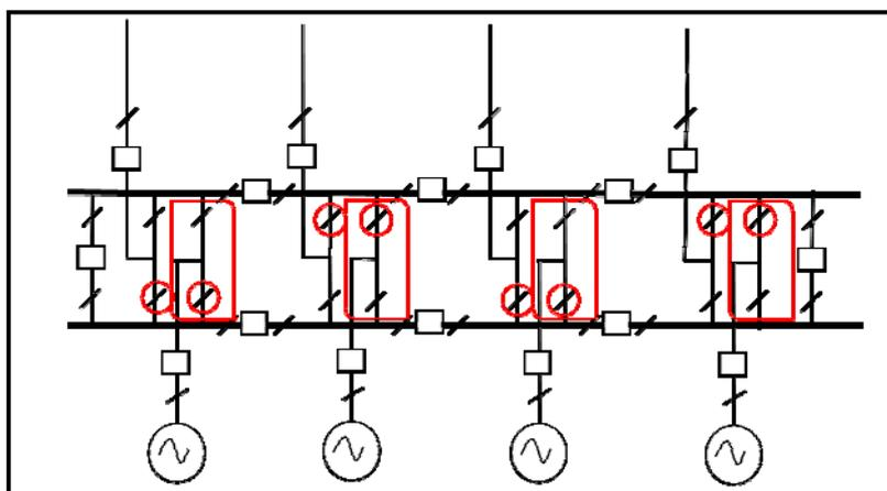
Connection method 9 is the most secure of the connection arrangements together with the addition of a fourth circuit.
