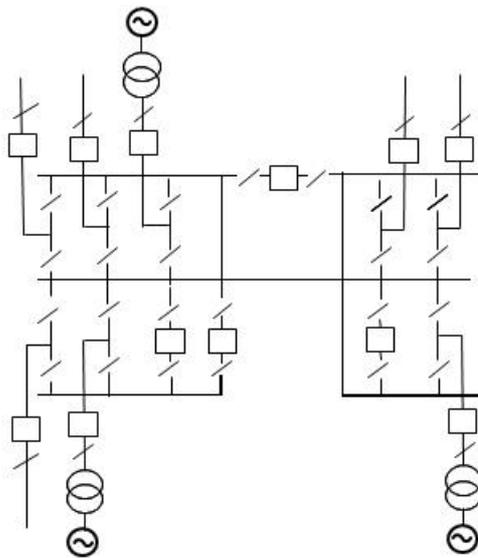
A.6.7.6 Firm connection, three section wrap-around busbar, (B/B end-wrap)
