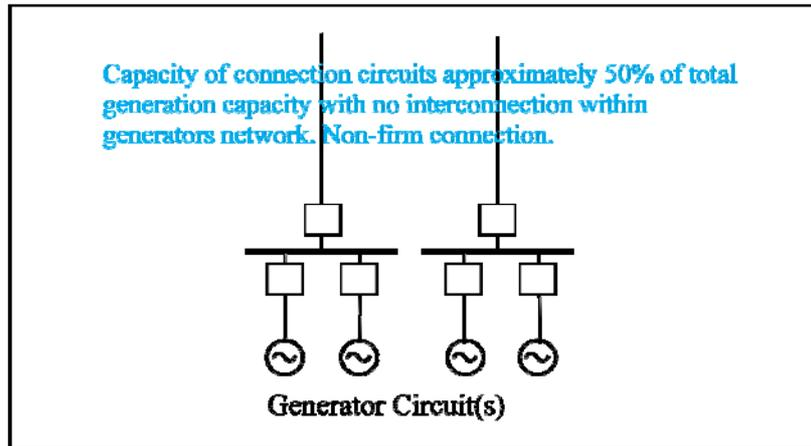
Figure 3: Method 3 – Non-firm, two single circuits, no interconnection
