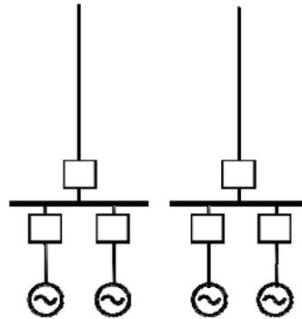
A.4.3.4 Non-firm, two circuits of reduced capacity
