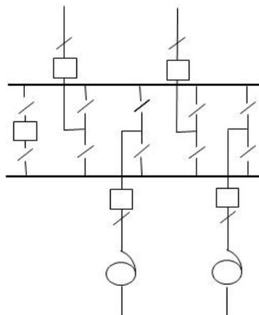
**A.8.7 Three section double busbar arrangement**
