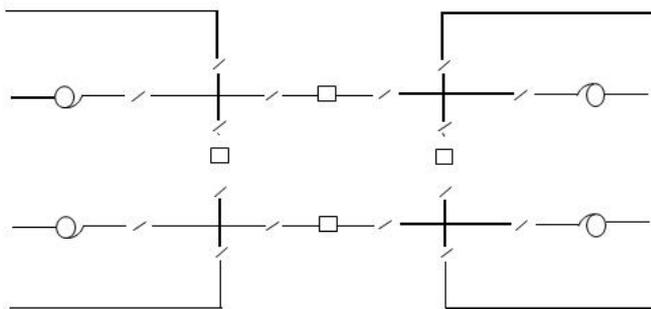
**A.8.5 Two section double busbar arrangement**
