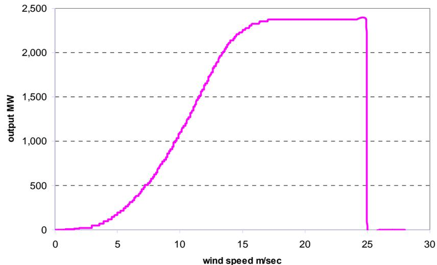
Figure 16 shows the generic windfarm power curve that we have used in this assessment. It is in fact a trace for a 2.4GW windfarm, but we scale this down appropriately.
