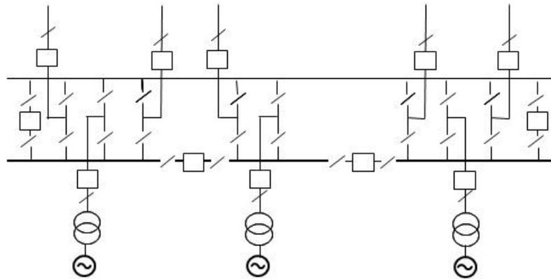
A.6.7.9 Firm connection, 3 circuits, four section double busbar
