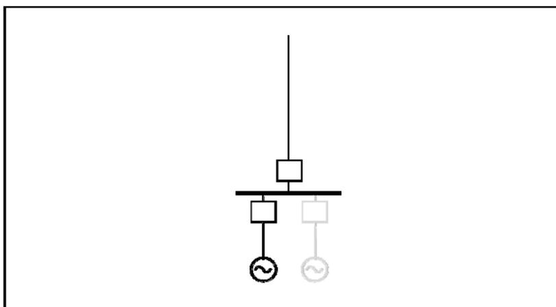
Figure 2: Method 2 - Single Circuit Radial, Transmission Connection Voltage
