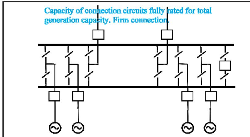
Figure 6: Method 6 - Firm connection, 2 circuits, two section double busbar
