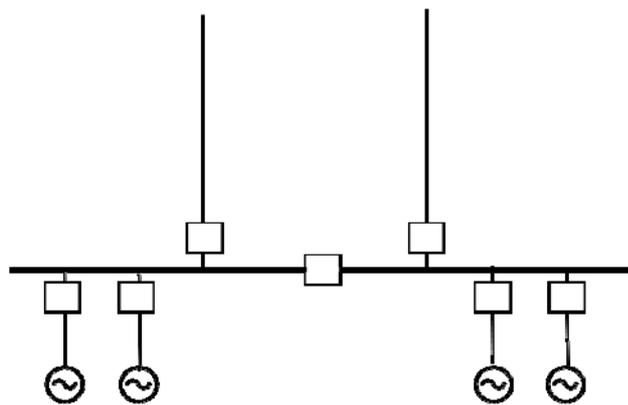
A.4.3.5 Non-firm, two fully rated circuits
