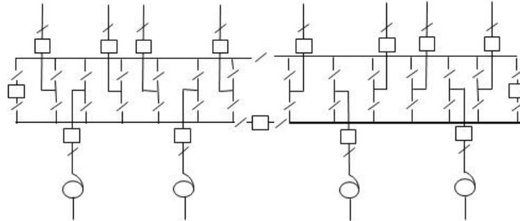
**A.7.7.4 Eight circuit marshalling Substation, Wrap-Around busbar**
