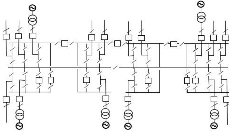
A.6.7.13 Firm connection, four section Wrap-Round Busbar, Central Main
