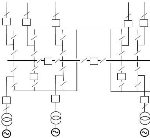
A.6.7.8 Firm connection, three section wrap-around busbar, main b'bar central
