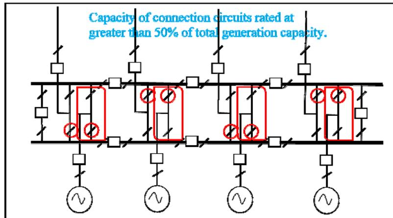
Figure 10: Alternative Method 9 - Firm Connection, 4 circuits, multi-mesh arrangement
