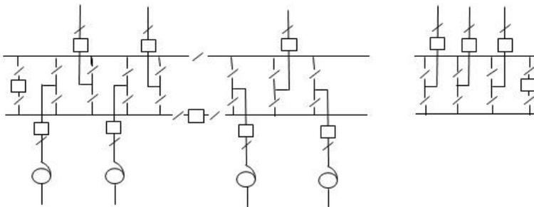
**A.7.7.3 Eight circuit marshalling Substation, Double busbar arrangement**
