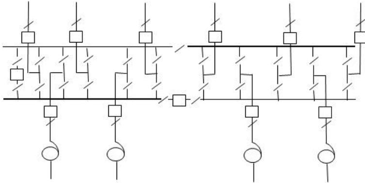
**A.7.7.2 Six circuit marshalling Substation, double B'bar with physical split**
