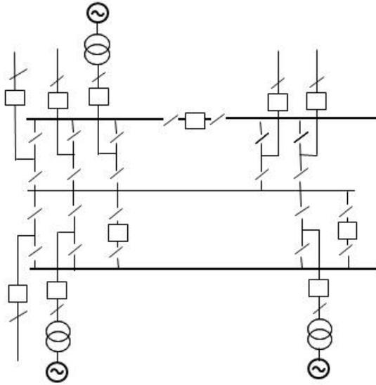
A.6.7.7 Firm connection, three section wrap-around busbar, main b'bar central
