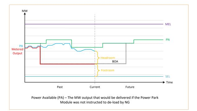
Figure 5: PA behaviour during Frequency Response
