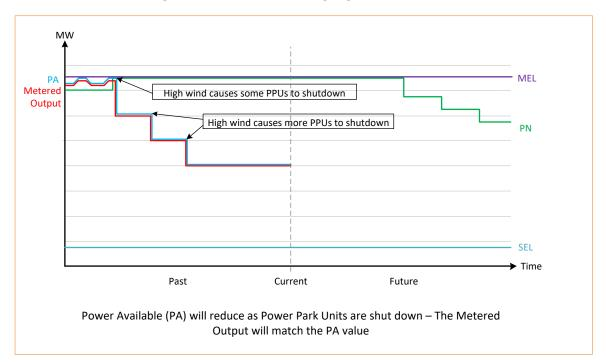
Figure 7: PA Behaviour during High Wind Shutdown
