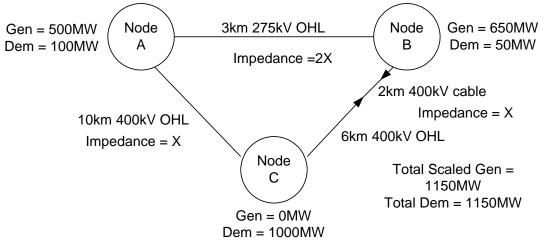
Step 2:Net export from Node B to Node C is 1000MW; route BC has impedance X and route BA-AC has impedance 3X; hence 750MW would flow down BC and 250MW along BA-AC
