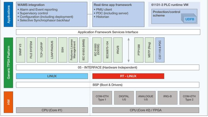
Figure 62: Software and applications used by the PhasorController
