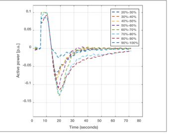
Figure 20b: 5s duration park level IR for D7 wind farm turbine with 20% to 100% of rated power; mean profile
