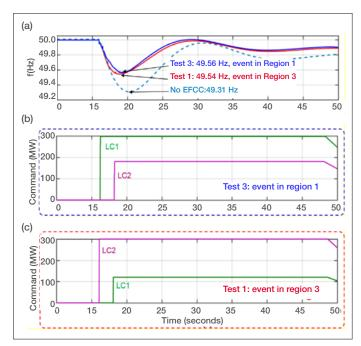
Figure 25: Example test results for evaluating the performance of the EFCC scheme
