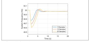
Figure 23: Comparison of system frequency containment with different samples for RoCoF calculation
