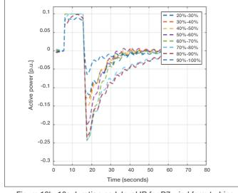
Figure 19b: 10s duration park level IR for D7 wind farm turbine with 20% to 100% of rated power; mean profile
