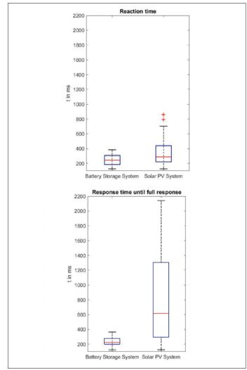
Figure 36: Reaction and response time analysis of the individual hybrid resources battery and solar PV system logged during the hardware in the loop test series.
