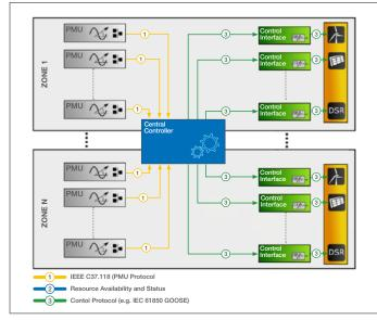
Figure 44: Centralised control scheme design approach
