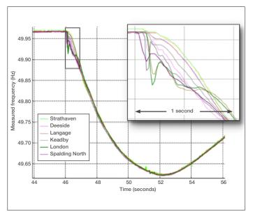
Figure 48: System frequency divergence immediately after an event
