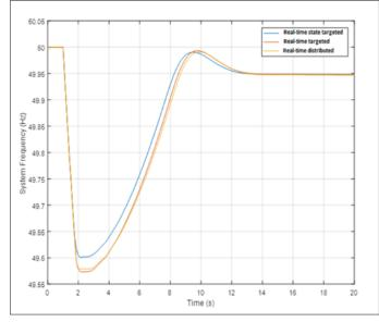
Figure 22: Comparison of the three control methods for 1560 MW generation loss in the south west zone in 2020/21
