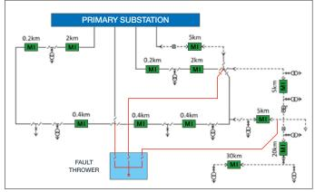
Figure 13: Single line diagram of the PNDC network
