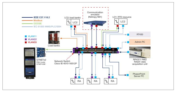
Figure 51: Physical connection of the various devices required for the tests at PNDC.
