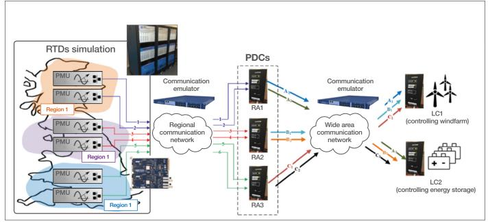
Figure 15: Test setup for evaluating the communication performance impact on the operation of the MCS
