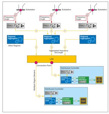
Figure 60: A PMU communication and data flow for the MCS
