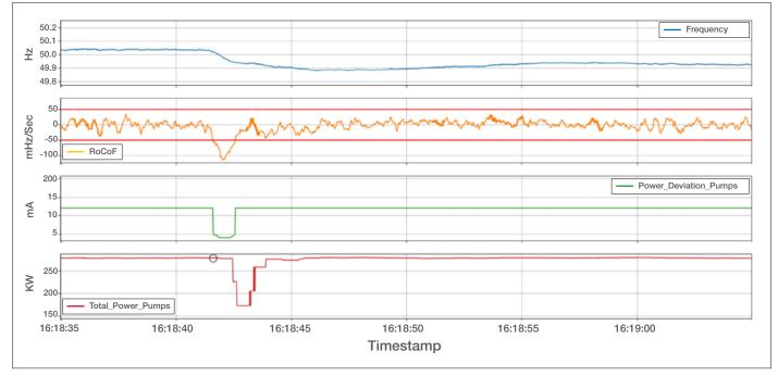
Figure 32(a): Negative RoCoF event at the waste water pumping station
