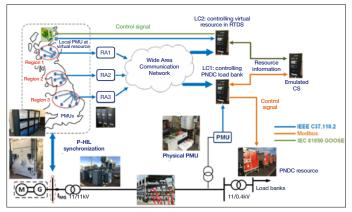
Figure 14: P-HiL testbed for testing the MCS wide area operational mode
