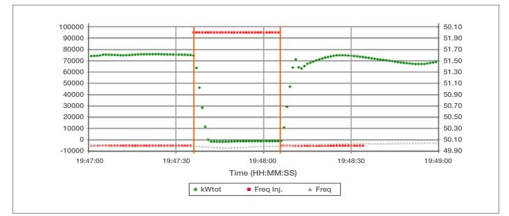
Figure 38: Burbo Bank ramp rate limit (test 9)
