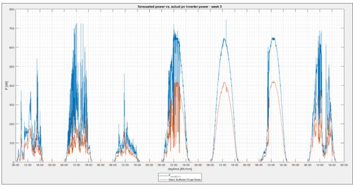
Figure 34: Real power output (blue graph) vs. forecasted power output (orange graph) for irradiance data during one week in April 2018 at the Rainbows solar PV farm
