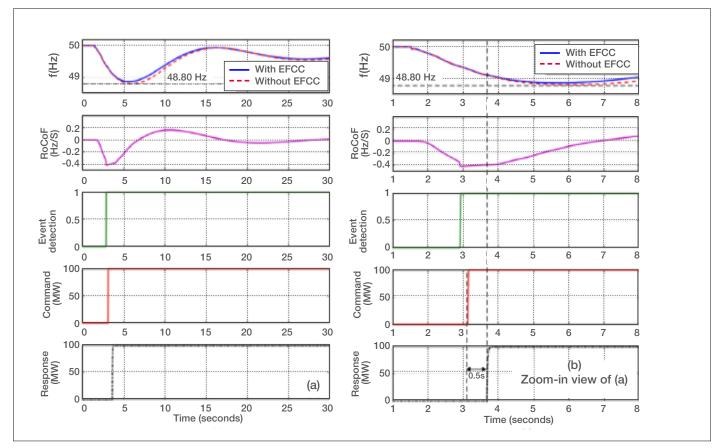
Figure 27: Test results for both frequency and RoCoF thresholds that are enabled in resource allocation block - 82 GVAs
