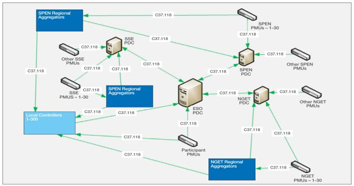
Figure 41: PMU and PhasorController C37.118 data streams across the network
