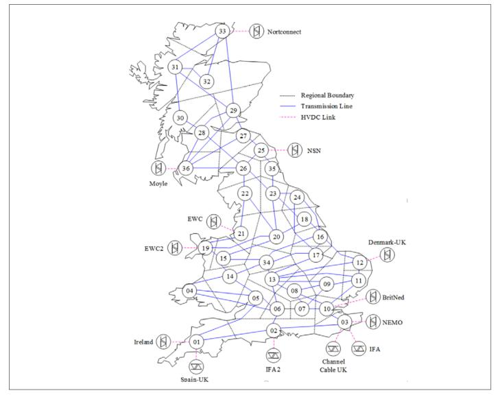
Figure 58: 36-bus model of the Great Britain electricity transmission system
