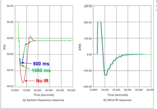
Figure 39: SGRE wind response (5s mean profile, 20-30% loading of rated power, 2 GVA)
