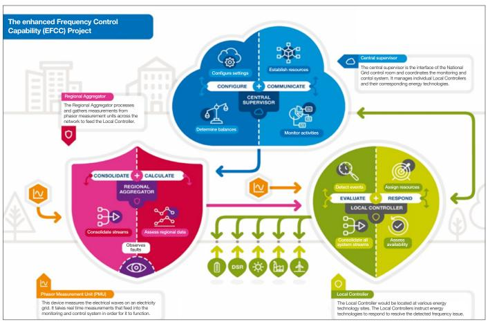
Figure 8: Monitoring and control system
