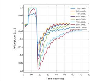
Figure 19a: 10s duration park level IR for D7 wind farm turbine with 20% to 100% of rated power; conservative profile
