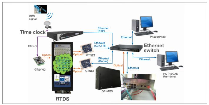
Figure 50: Physical connection of the various devices required for the tests at UoM.
