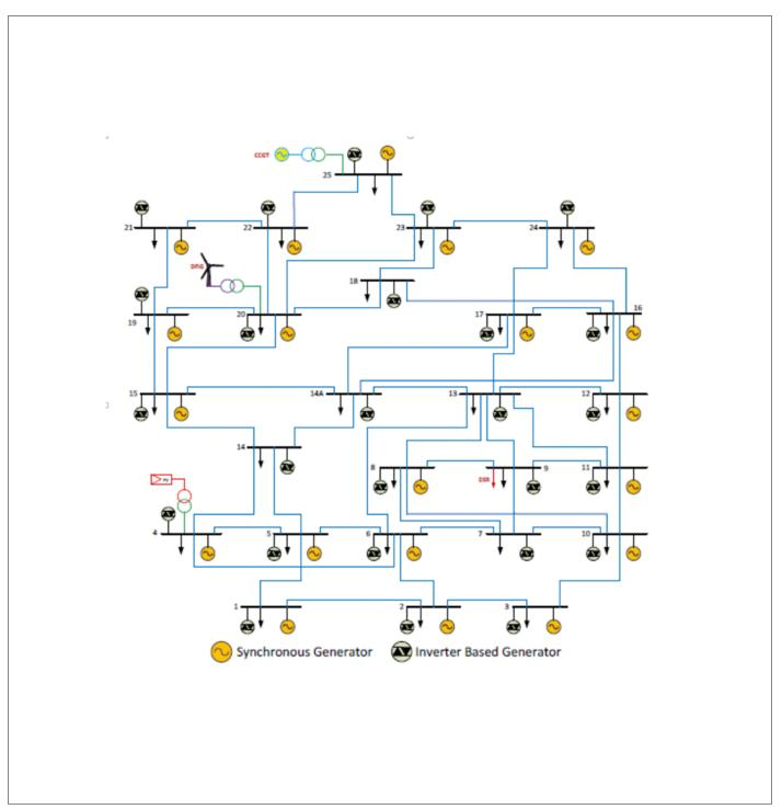
Figure 59: Diagram of 26-bus model of the GB electricity transmission system
