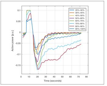
Figure 20a: 5s duration park level IR for D7 wind farm turbine with 20% to 100% of rated power; conservative profile
