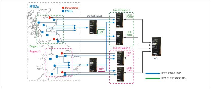
Figure 12: The test setup with the MCS controllers, PMUs and representative service providers
