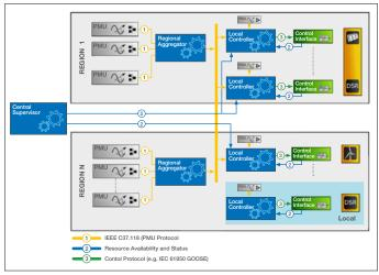
Figure 45: Decentralised control scheme design approach
