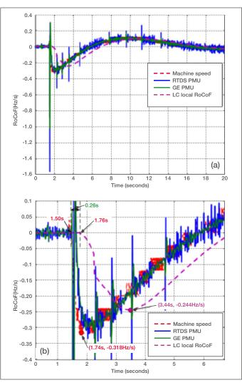
Figure 26: RoCoF measurements for 1GW generation loss (Region 3)
