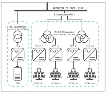
Figure 17: Schematic of the solar PV+Storage Hybrid System with 3.7MW Rainbows solar PV farm and 1MW/1MWh Energy Buffer Unit (EBU) 1000 in Willersey, UK
