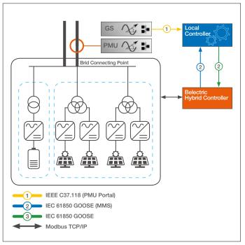
Figure 52: Communication setup with PMU simulator
