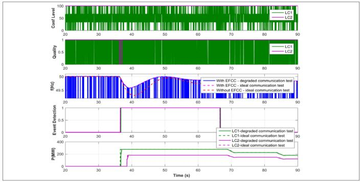
Figure 30: Example test results for evaluating the impact of communication jitters on the performance of the EFCC scheme
