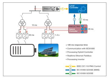
Figure 18: Communication overview and communication protocols used between the different systems control and components
