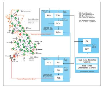
Figure 3: Real-time targeted control, real-time distributed control and real-time state targeted control techniques
