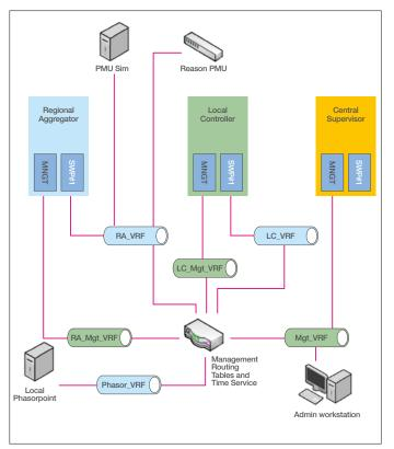
Figure 53: High level network test environment
