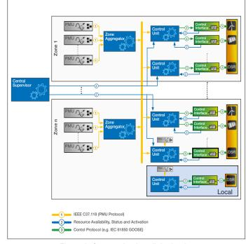
Figure 9: Communications links for the monitoring and control system
