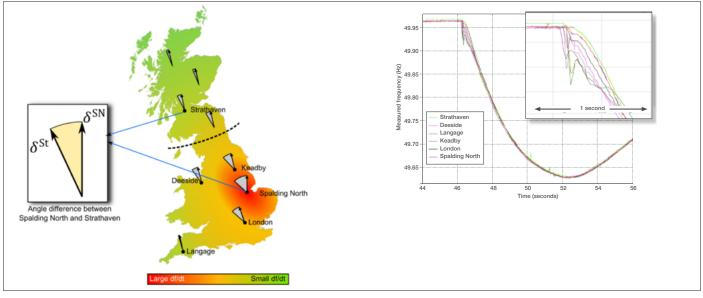
Figure 5: Phase angle behaviour after loss of generator
