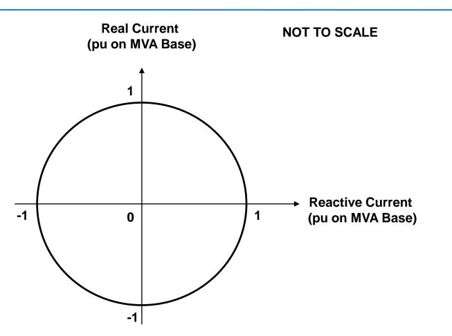
NOTE:- 1 pu current is the rated current of the Power Park Module or HVDC Equipment when operating at full MW output and full leading or Lagging MVAr capability (eg for a 100MW Power Park Module Rated Current would be obtained when the Power Park Module is supplying 100MW and 0.95 Power Factor lead or 0.95 Power Factor lag at the Connection Point)
