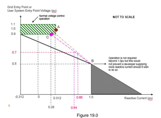
In terms of time frames and reactive current injection the minimum performance requirement that would be expected is shown in Figures 20 and 21. There is no real difference between these two figures other than in respect of the fault clearance time. In this example the green hashed area is showing the effect of the pre-fault operating condition of the Power Park Module.
