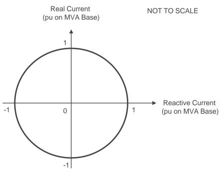
NOTE:- 1 pu current is the rated current of the Power Park Module or HVDC Equipment when operating at full MW output and full leading or Lagging MVAr capability (eg for a 100MW Power Park Module Rated Current would be obtained when the Power Park Module is supplying 100MW and 0.95 Power Factor lead or 0.95 Power Factor lag at the Connection Point). Note this is the rating of the converter. When I<sub>R</sub> is less than 1.0 pu any residual reactive current should be supplied as Active Current
