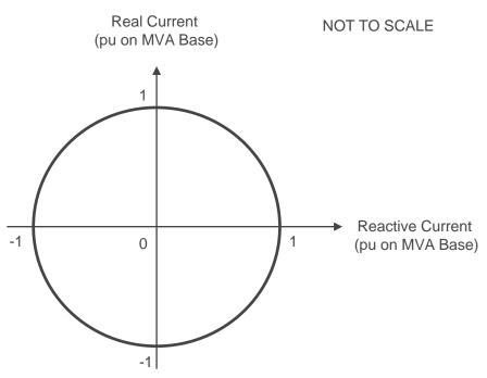
NOTE:- 1 pu current is the rated current of the Power Park Module or HVDC Equipment when operating at full MW output and full leading or Lagging MVAr capability (eg for a 100MW Power Park Module Rated Current would be obtained when the Power Park Module is supplying 100MW and 0.95 Power Factor lead or 0.95 Power Factor lag at the Connection Point)
