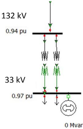
Figure 28 DSO solves the undervoltage problem in Bolney using tap changing transformers
