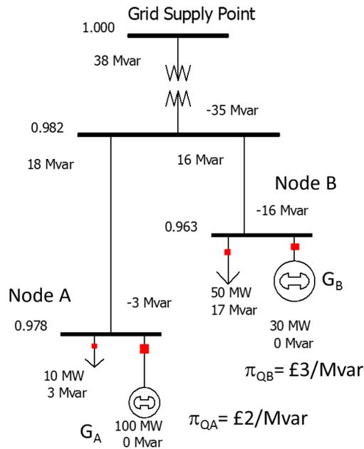
**Figure 2 A distribution system with DER**
