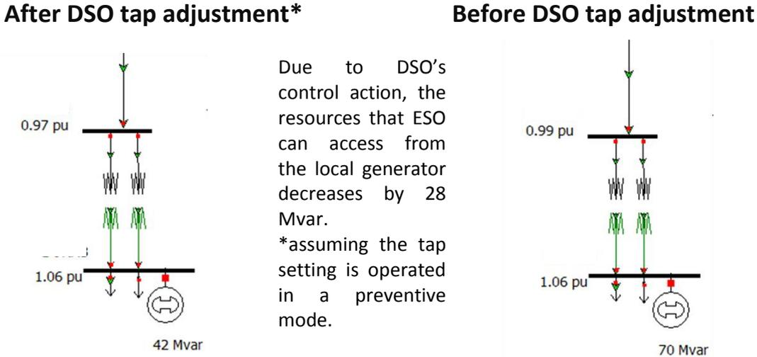
**Figure 29 Impact of different settings of transformers on the maximum reactive capability that can be delivered by the local generator**
