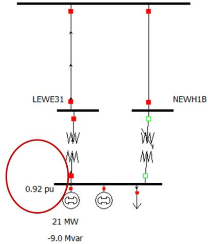
Figure 7 An undervoltage problem caused by non-coordinated DSO-ESO control actions
