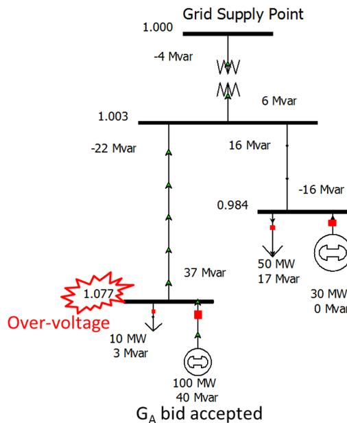
**Figure 3 An overvoltage problem caused by no ESO-DSO coordination**
