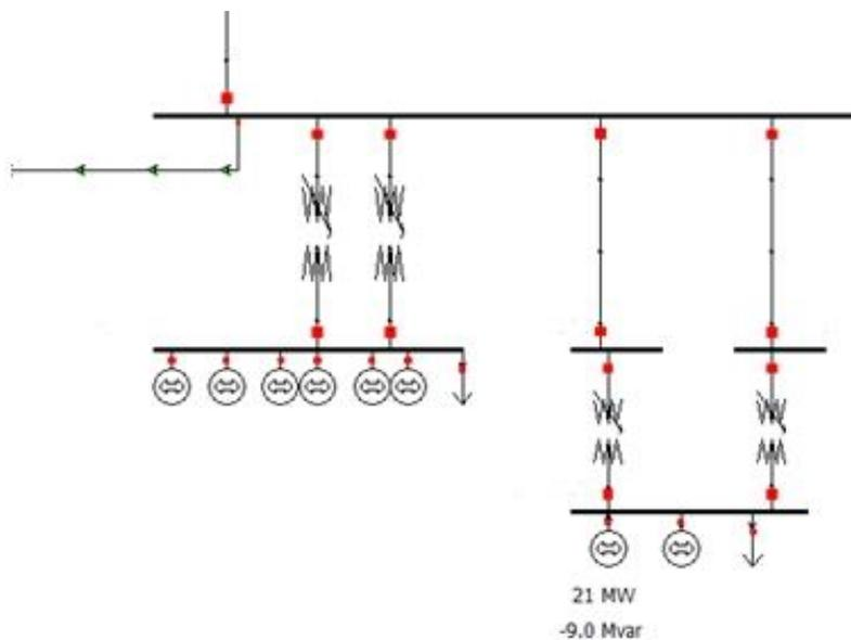
Figure 17 A power Potential unit in Ninfield VPP is used to correct the overvoltage problem at Ninfield 400 kV
