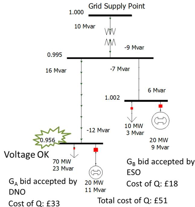
**Figure 14 Step 2 of DSO-ESO incremental approach: ESO uses the DSO solution and adds more reactive supports to meet its requirement**
