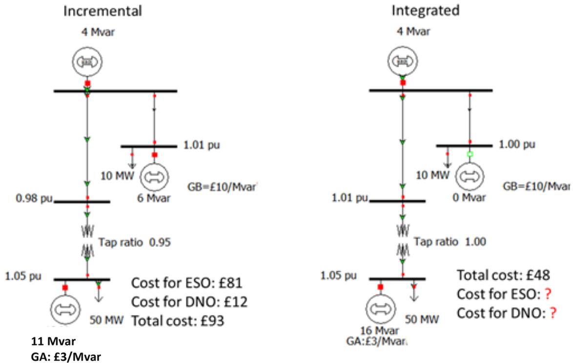
Figure 24 Comparison between the incremental and integrated solution with no smart (preventive) control
