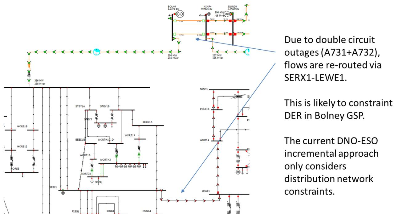
**Figure 31 Impact of transmission outages on the distribution system**
