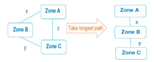
Parallel zones – parallel zones will be amalgamated with the incremental km immediately beyond the amalgamated zones being the greater of those existing prior to the amalgamation. An illustrative example is shown below with a, b, c, and d representing the initial incremental km between zones, and x and y representing the final incremental km following zonal amalgamation.
