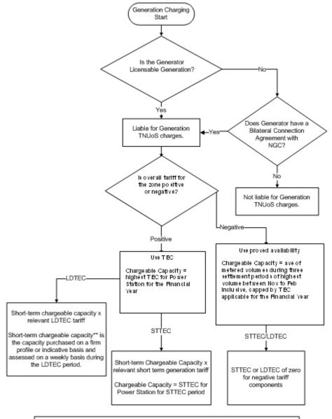
Ave = average BMU = BM Unit STTEC = Short-Term Transmission Entry Capacity
