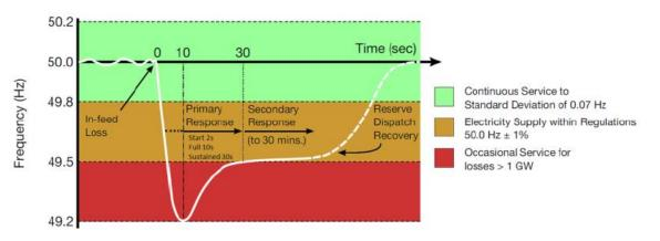
Figure 2 System Frequency Limits
