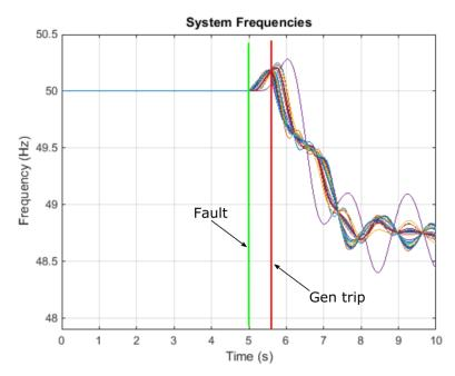
Figure 8: Fault followed by generator trip
