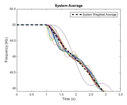
Figure 7: Plot showing frequencies measured at generator buses and the system aggregated frequency based on the centre of inertia technique
