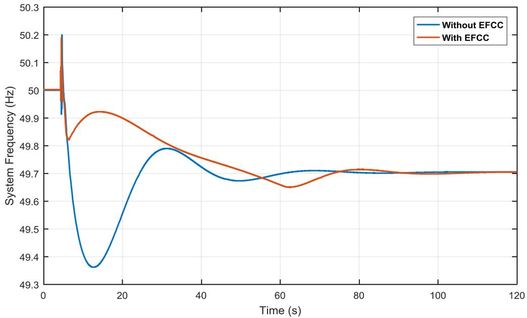
Figure 4-36 System frequency of generator tripping (Asyn at bus 5) after fault at bus 5 in zone 1
