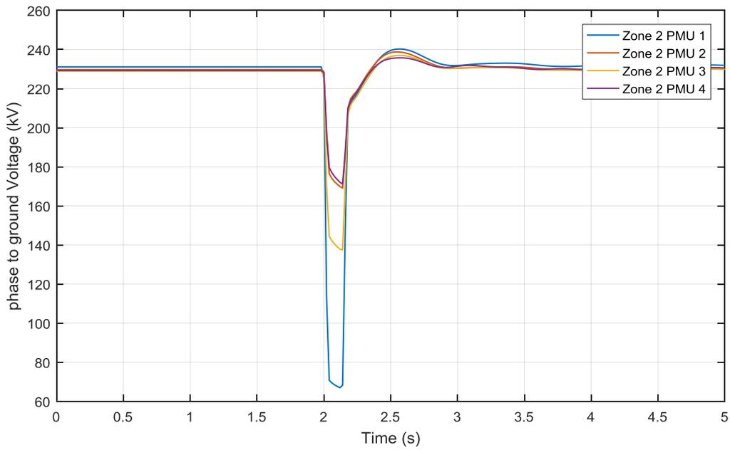
Figure 4-29 Zone 2 PMU voltages of 140 ms three phase ground fault at Bus 16 Zone 2
