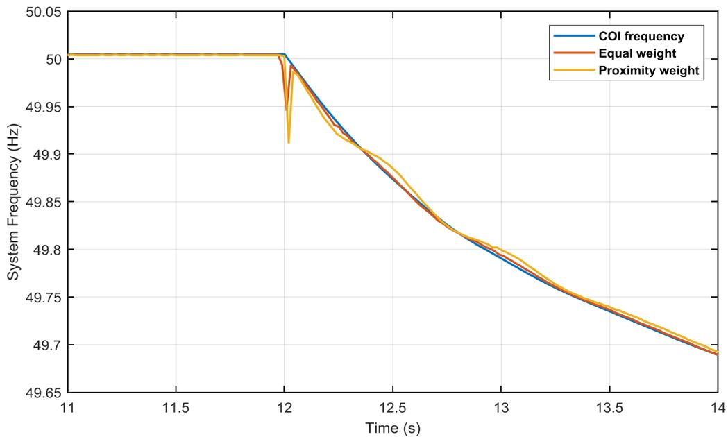
Figure 4-39 System frequency of different PMU weight configuration
