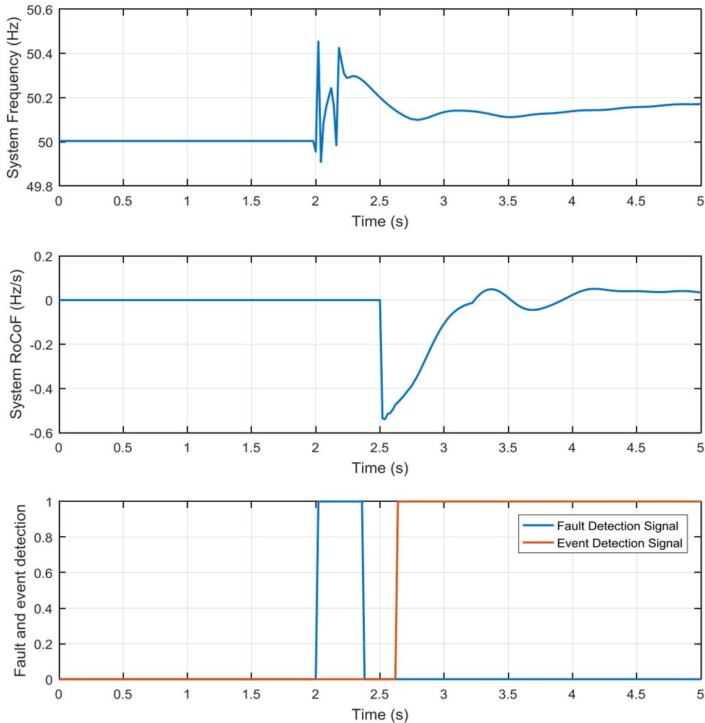
Figure 4-27 Simulation result of 140 ms three phase ground fault at Bus 16 Zone 2
