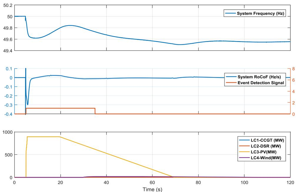
Figure 4-10 Simulation results of 1500 MW load increase at bus 9 zone 1
