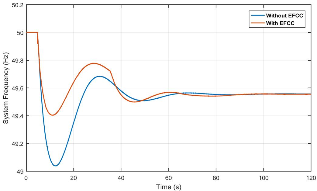
Figure 4-11 System frequency of 1000 MW load increase at bus 9 zone 1 with limited resources
