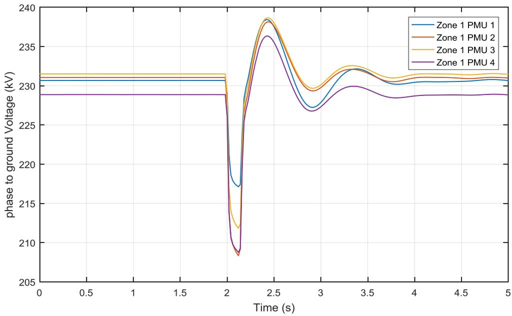
Figure 4-19 Zone 1 PMU voltages of 140 ms Single line ground fault at Bus 16 Zone 2
