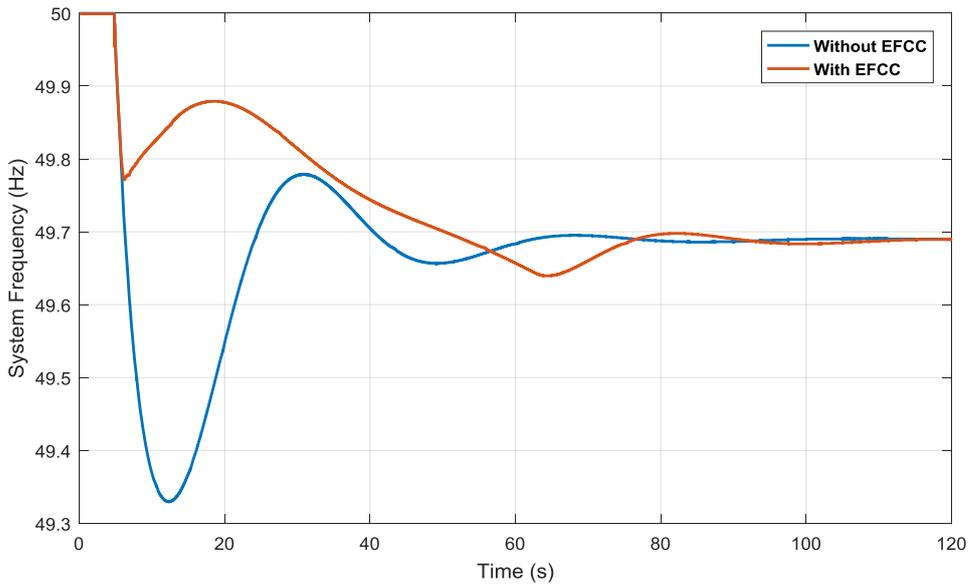
Figure 4-7 System frequency of 1000 MW load increase at bus 21 zone
