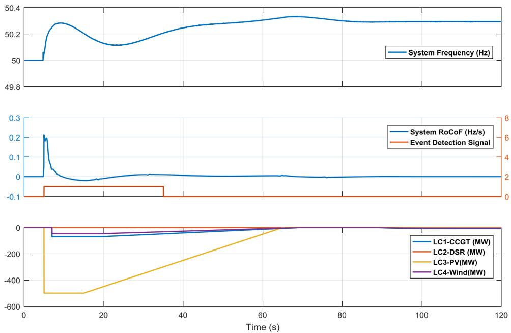
Figure 4-14 Simulation result of 1000 MW load increase at bus 9 zone 1 with limited resources
