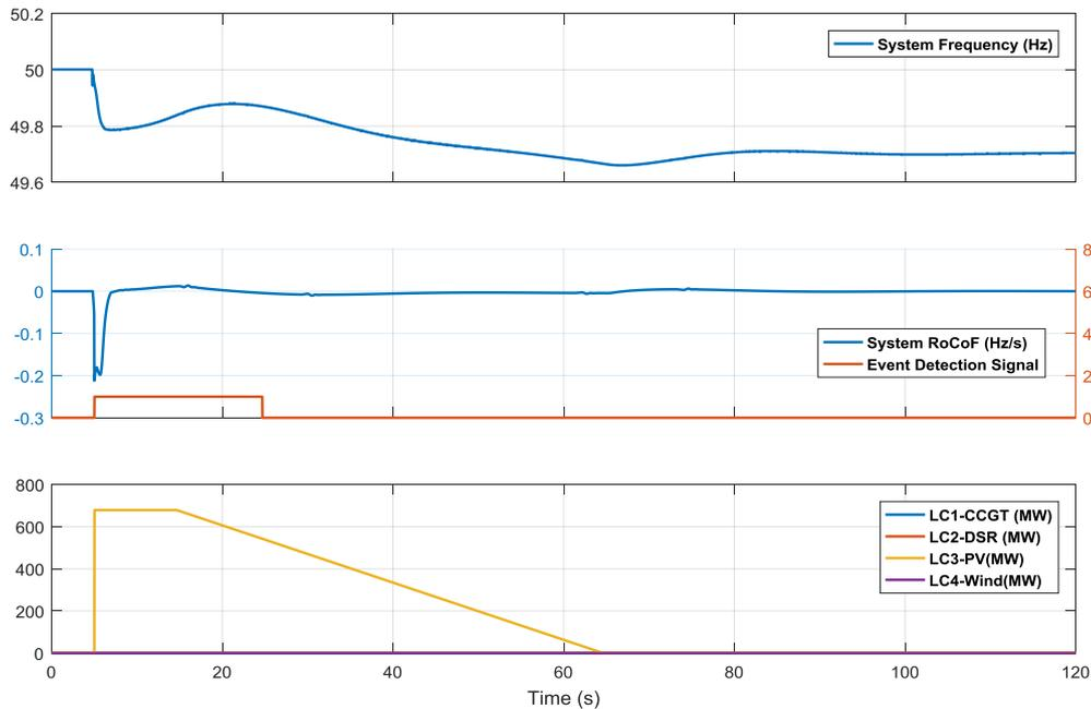
Figure 4-2 Simulation results of 1000 MW load increase at bus 9 zone 1
