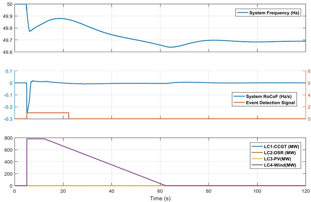
Figure 4-8 Simulation results of 1000 MW load increase with limited resources at bus 21 zone 2
