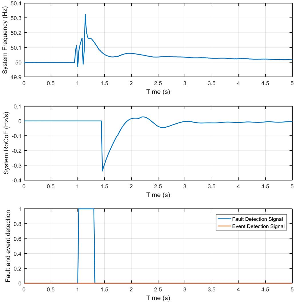
Figure 4-35 Simulation results of line 13-17 tripping after fault at bus 13
