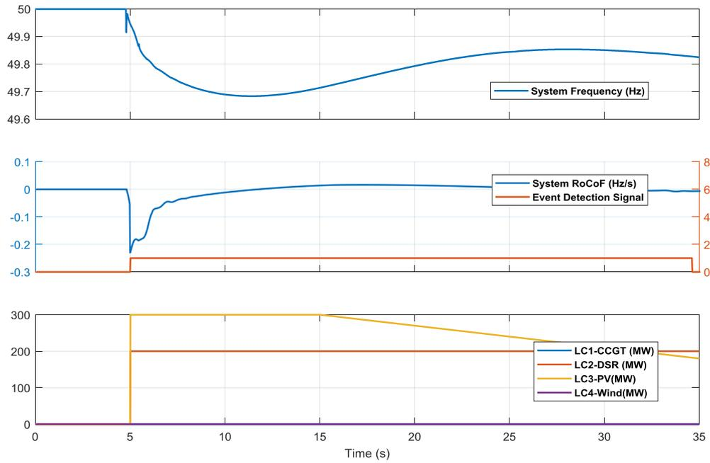
Figure 4-6 Simulation results of 1000 MW load increase at bus 9 zone 1 with limited resources
