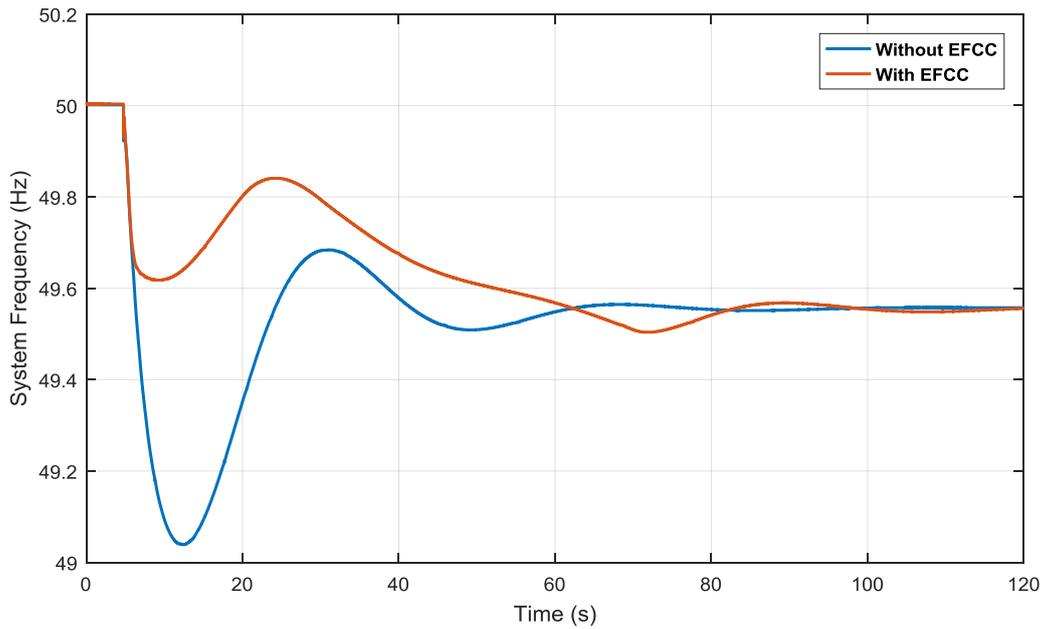
Figure 4-9 System frequency of 1500 MW load increase event at bus 9 zone 1
