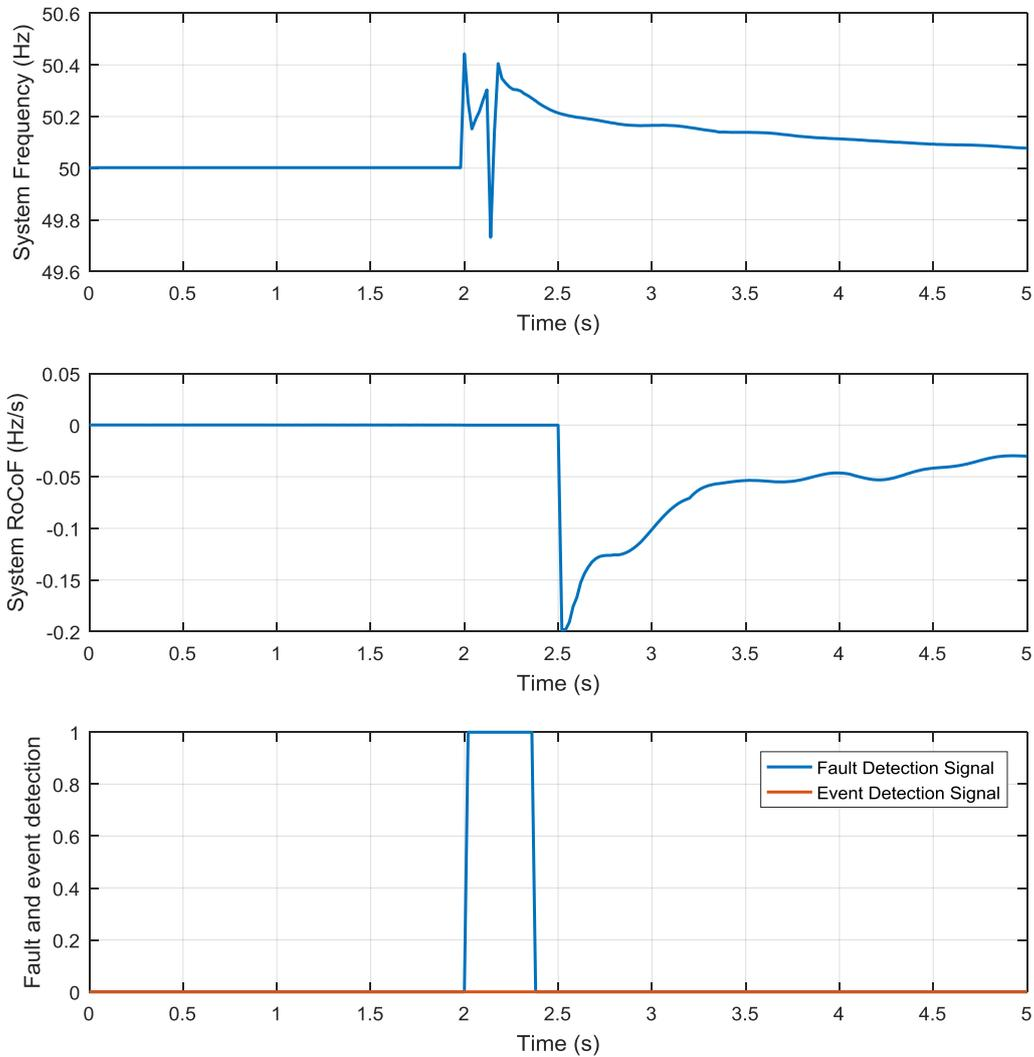
Figure 4-24 Simulation result of 140 ms three phase ground fault at Bus 3 Zone 1
