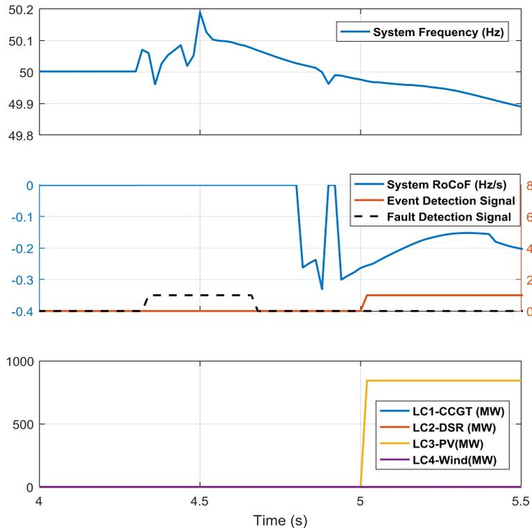
Figure 4-38 System frequency of generator tripping (Asyn at bus 5) after fault at bus 5
