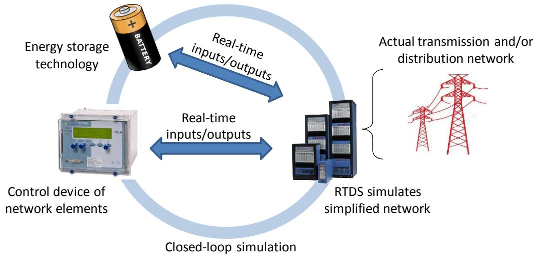
**Figure 2-1** Block diagram of the Manchester RTDS
