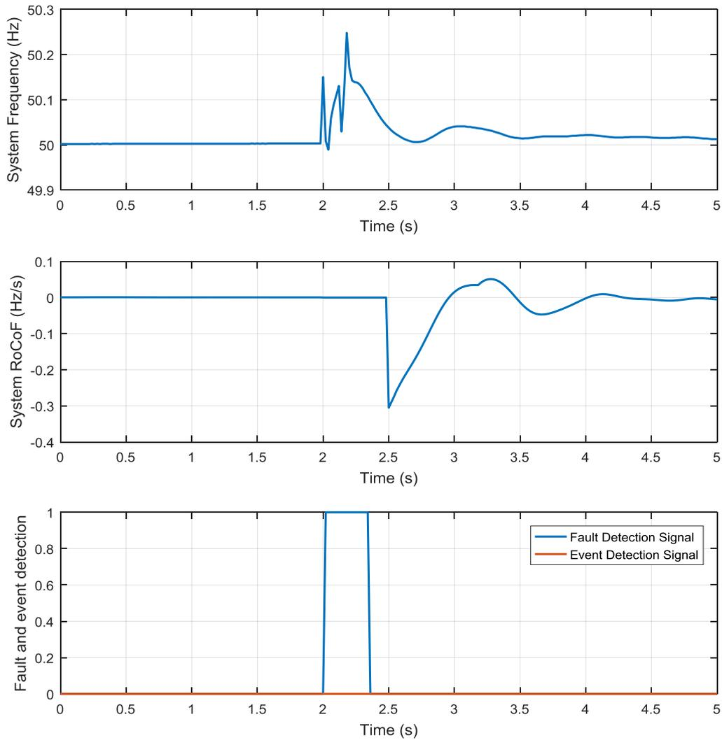
Figure 4-18 Simulation result of 140 ms Single line ground fault at Bus 16 Zone 2
