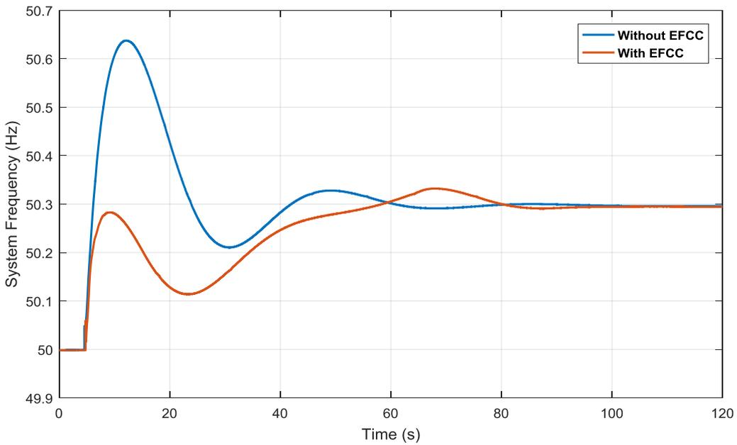
Figure 4-13 System frequency of 1000 MW load increase at bus 9 zone 1 with limited resources
