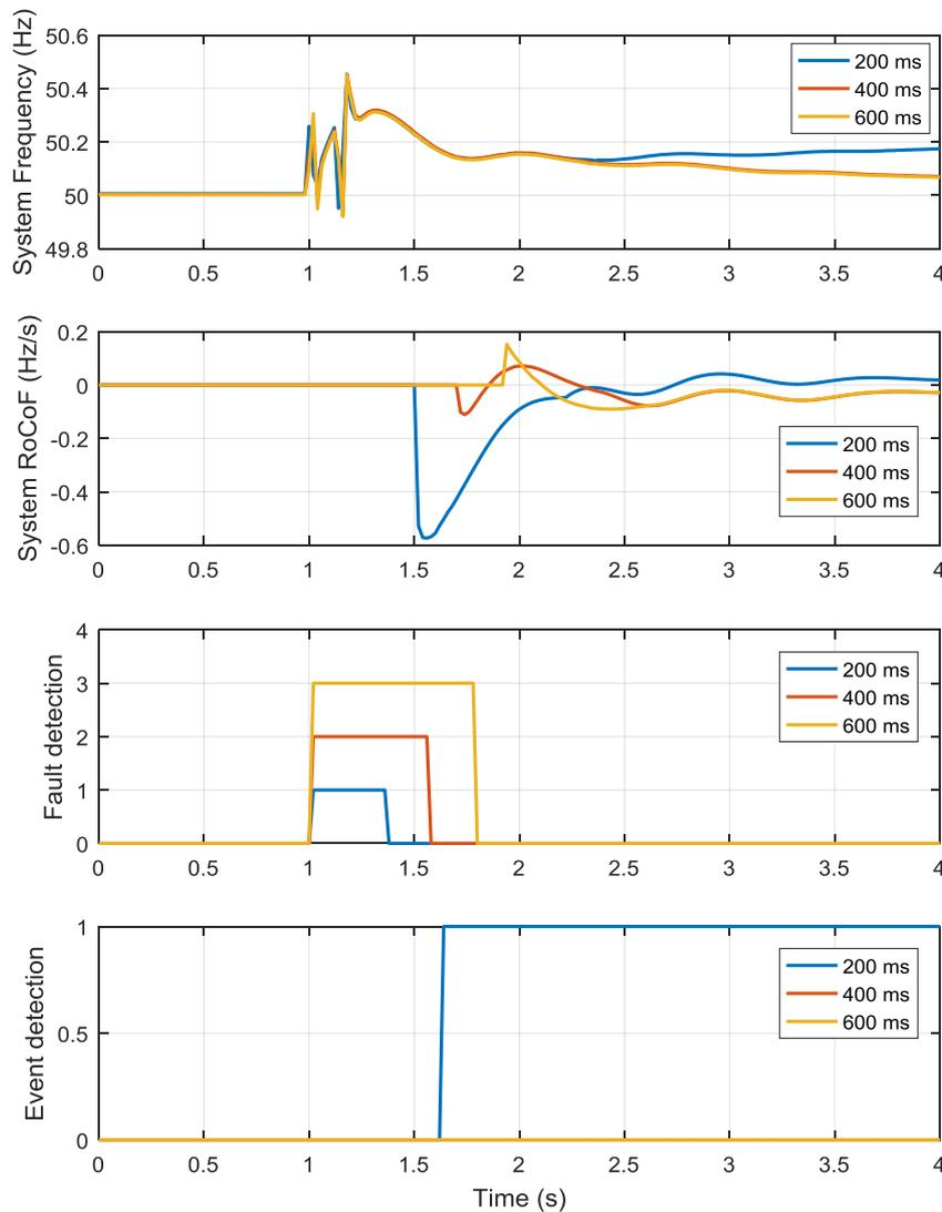
Figure 4-42 Sensitivity analysis of fault off hypnosis time after a three-phase fault at bus 5
