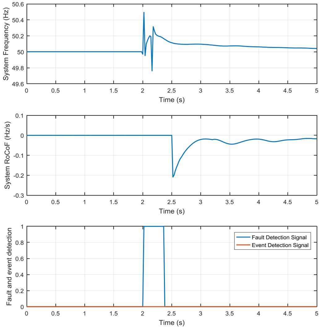
Figure 4-21 Simulation result of 140 ms two phase ground fault at Bus 3 Zone 1
