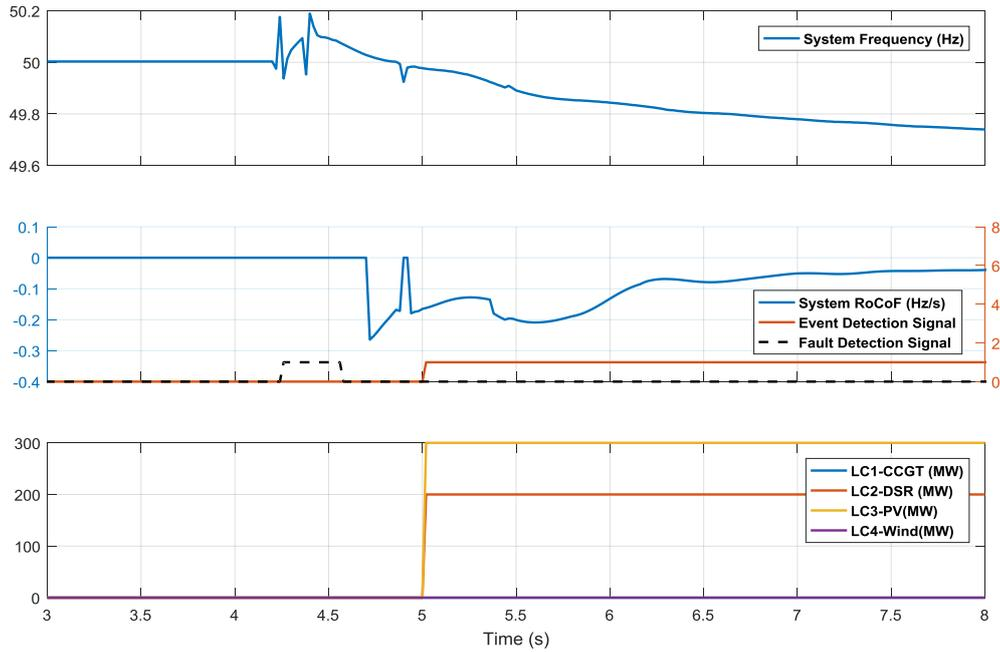
Figure 4-32 Simulation results (Zoomed) of load increase after fault at bus 8
