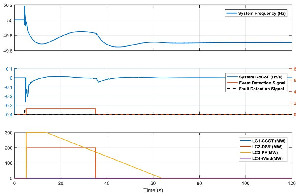
Figure 4-31 Simulation results (Zoomed) of load increase after fault at bus 8
