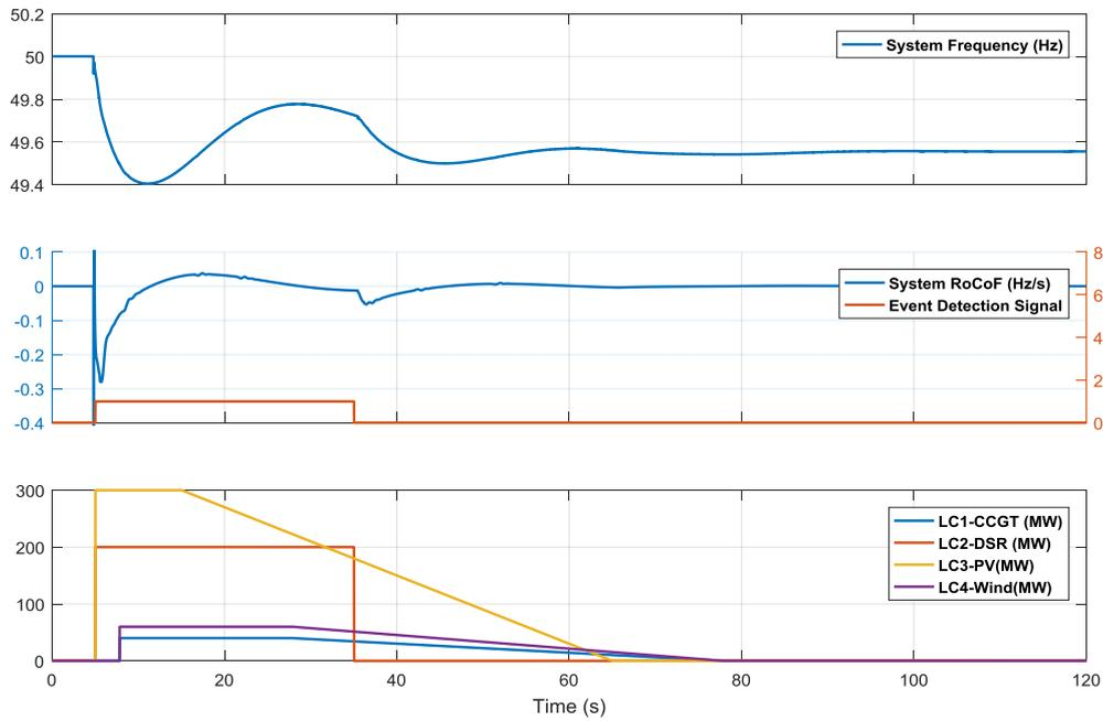
Figure 4-12 Simulation results of 1500 MW load increase at bus 9 zone 1 with limited resources
