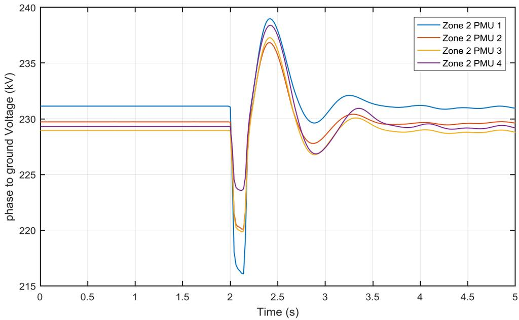
Figure 4-23 Zone 2 PMU voltages of 140 ms two phase ground fault at Bus 3 Zone 1
