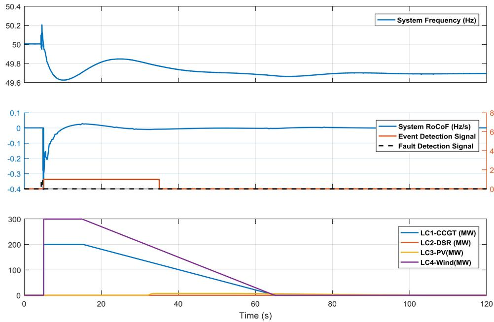
Figure 4-33 Simulation results of load increase after fault at bus 22 in zone 2
