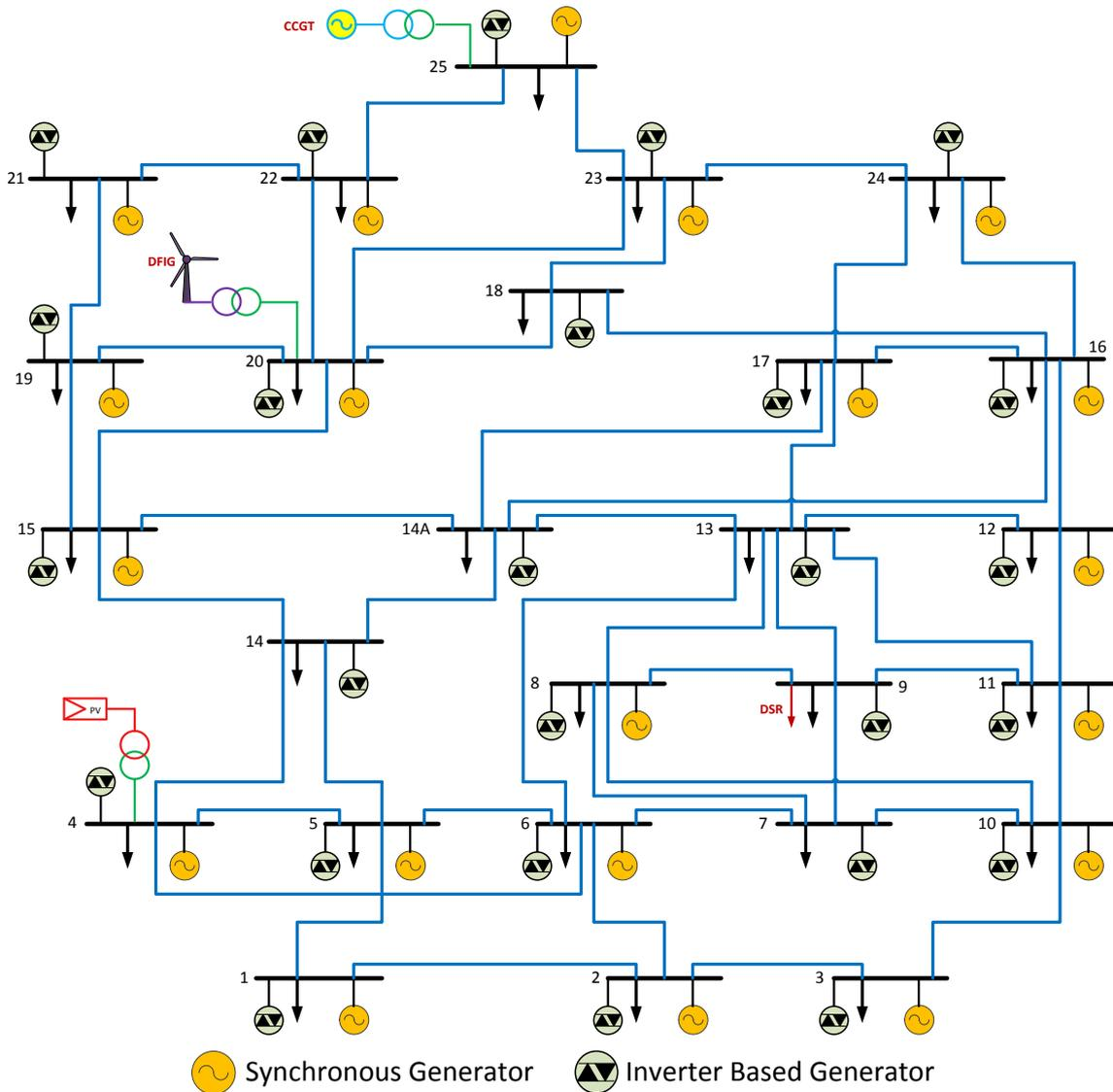
Figure 2-2: Single line diagram model of GB network test system
