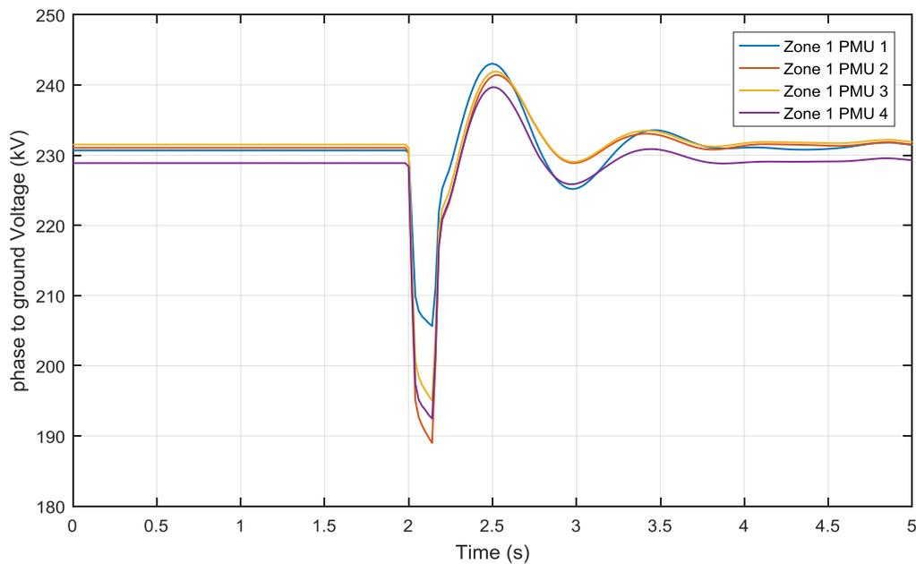
Figure 4-28 Zone 1 PMU voltages of 140 ms three phase ground fault at Bus 16 Zone 2
