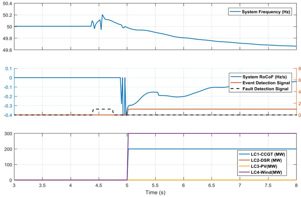
Figure 4-34 Simulation results (Zoomed) of load increase after fault at bus 22
