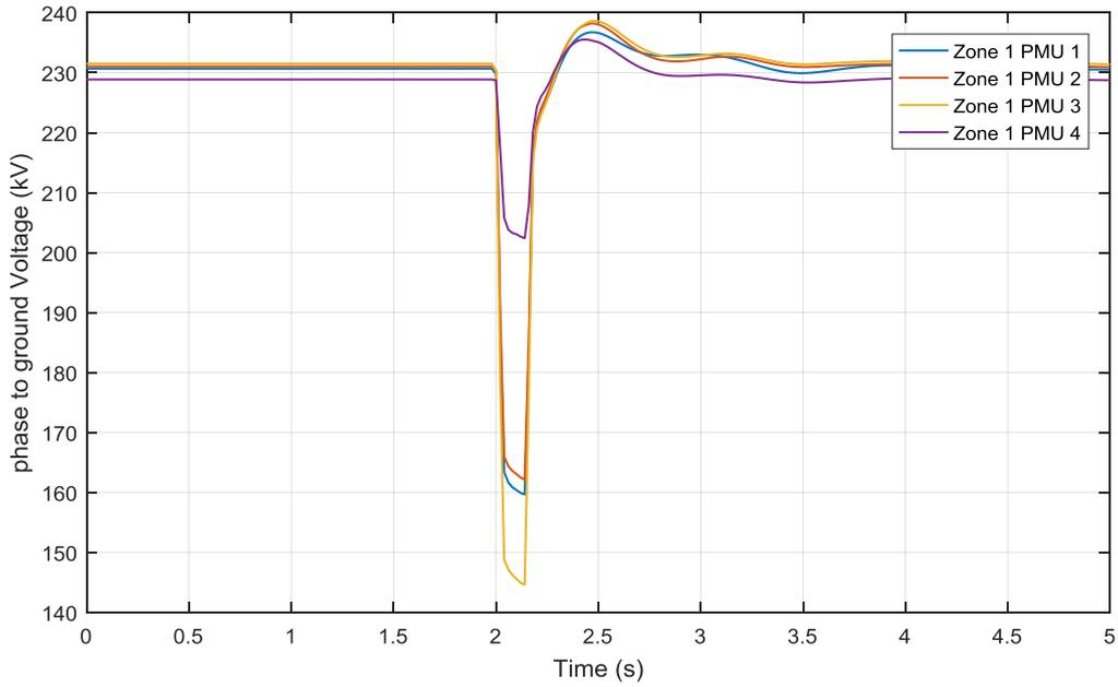
Figure 4-22 Zone 1 PMU voltages of 140 ms two ground fault at Bus 3 Zone 1
