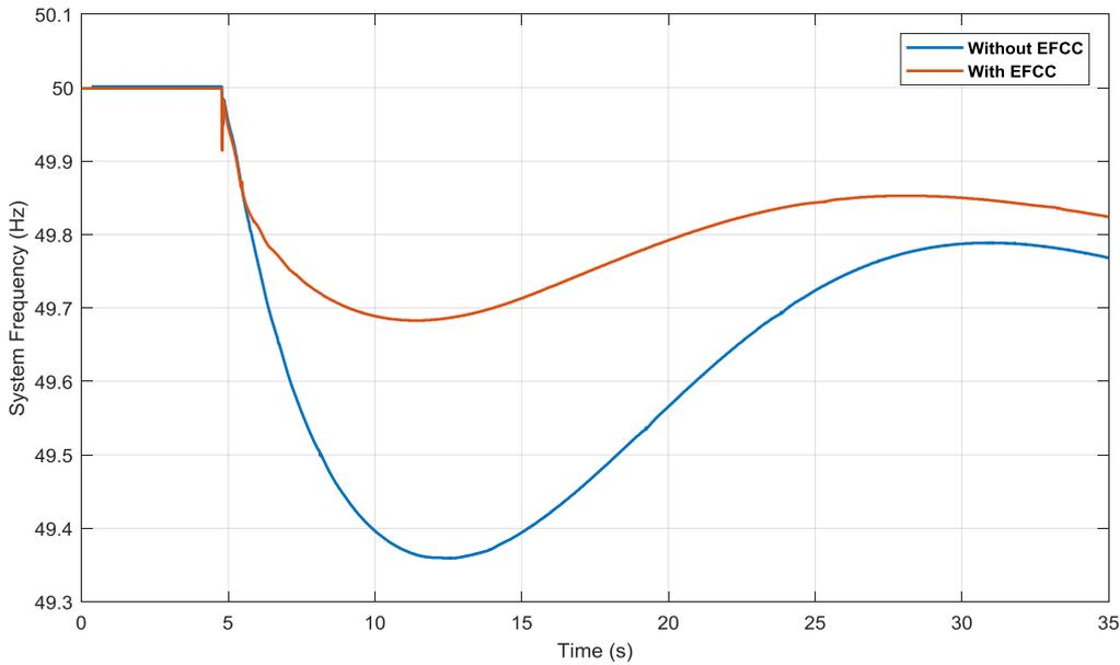
Figure 4-5 System frequency of 1000 MW load increase at bus 9 zone 1 with limited resources
