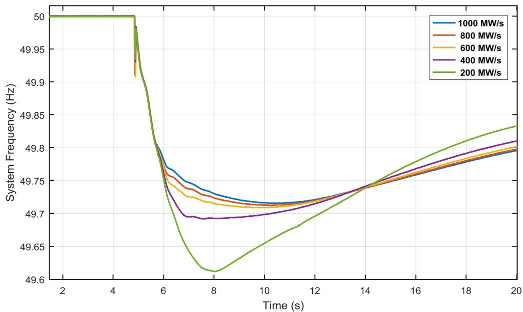
Figure 4-46 Frequency response (zoomed) of different service provider response ramping rates
