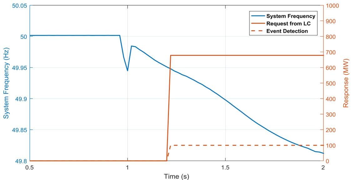
Figure 4-4 Simulation results of 1000 MW load increase at bus 9 zone 1
