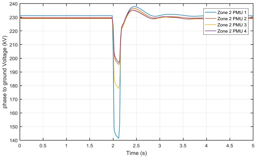
Figure 4-20 Zone 2 PMU voltages of 140 ms Single line ground fault at Bus 16 Zone 1
