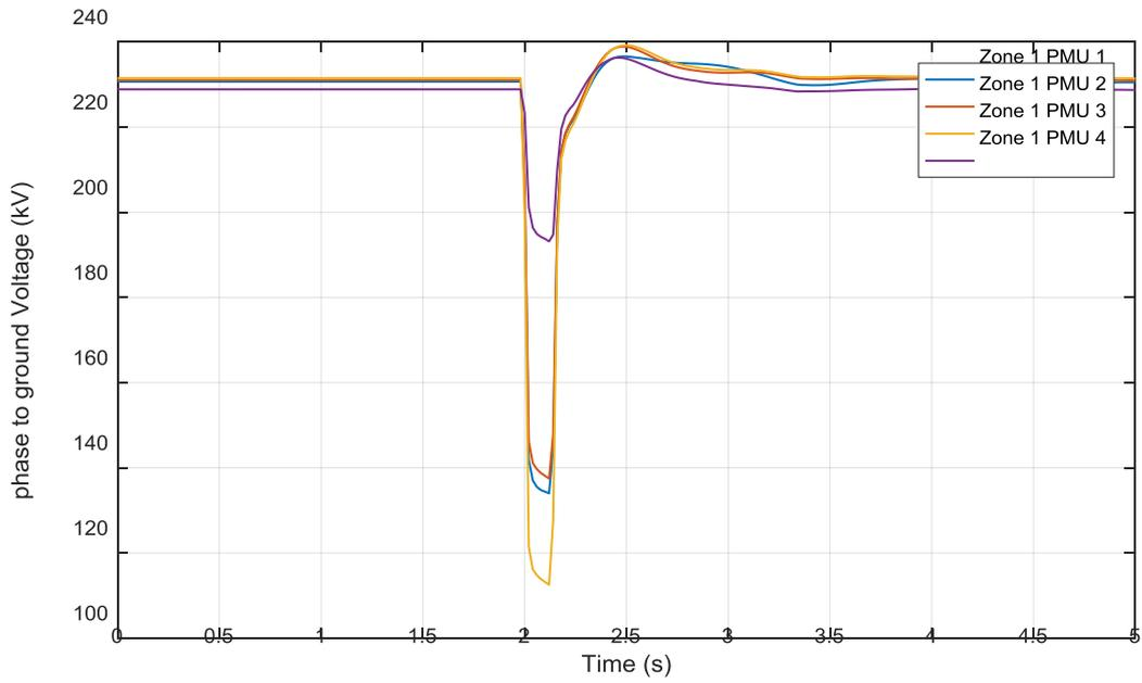
Figure 4-25 Zone 1 PMU voltages of 140 ms three phase ground fault at Bus 3 Zone 1
