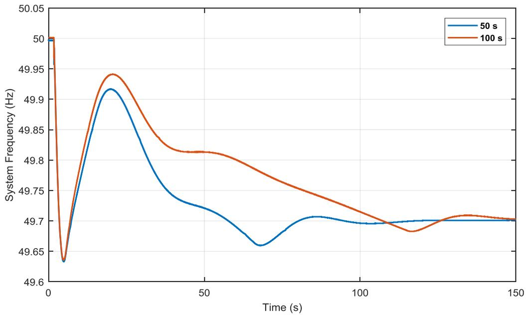
Figure 4-3 Simulation results of 1000 MW load increase at bus 9 zone 1 with two different resource pulling off speed
