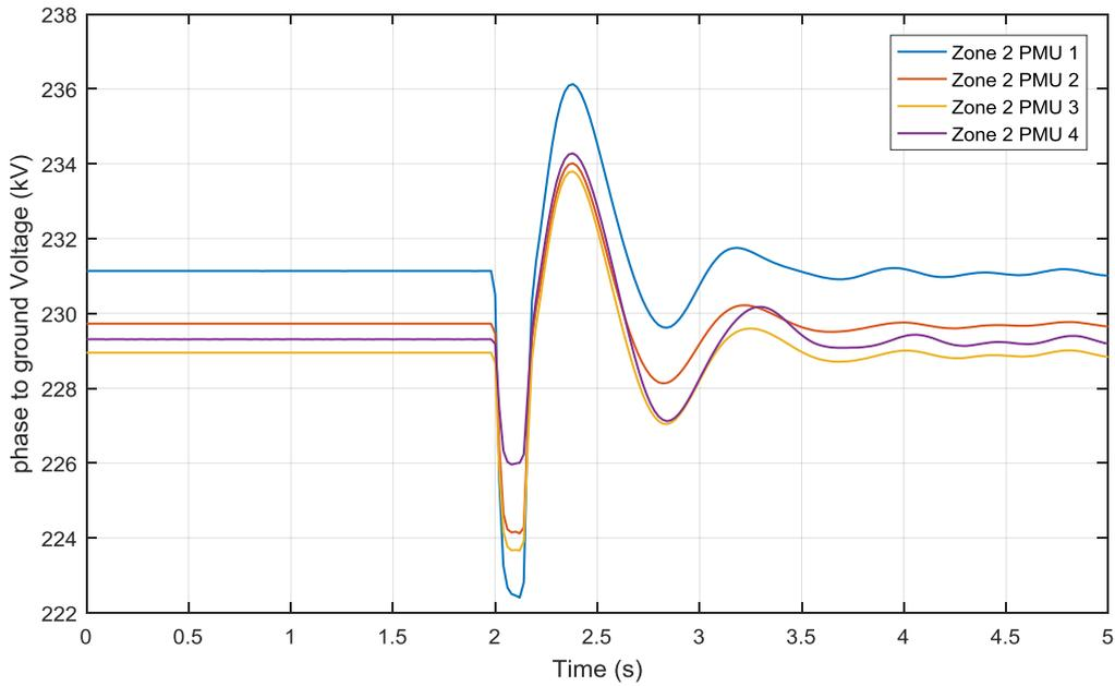
Figure 4-17 Zone 2 PMU voltages of 140 ms Single line ground fault at Bus 3 Zone 1
