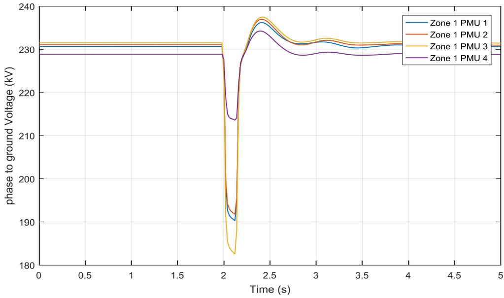
Figure 4-16 Zone 1 PMU voltages of 140 ms Single line ground fault at Bus 3 Zone 1
