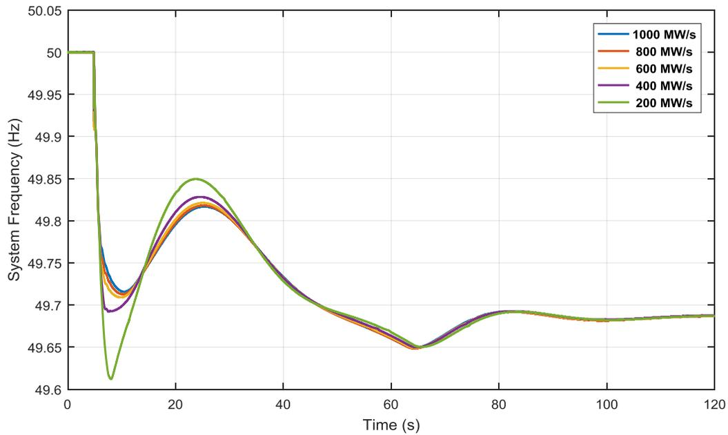
Figure 4-45 Frequency response of different service provider response ramping rates
