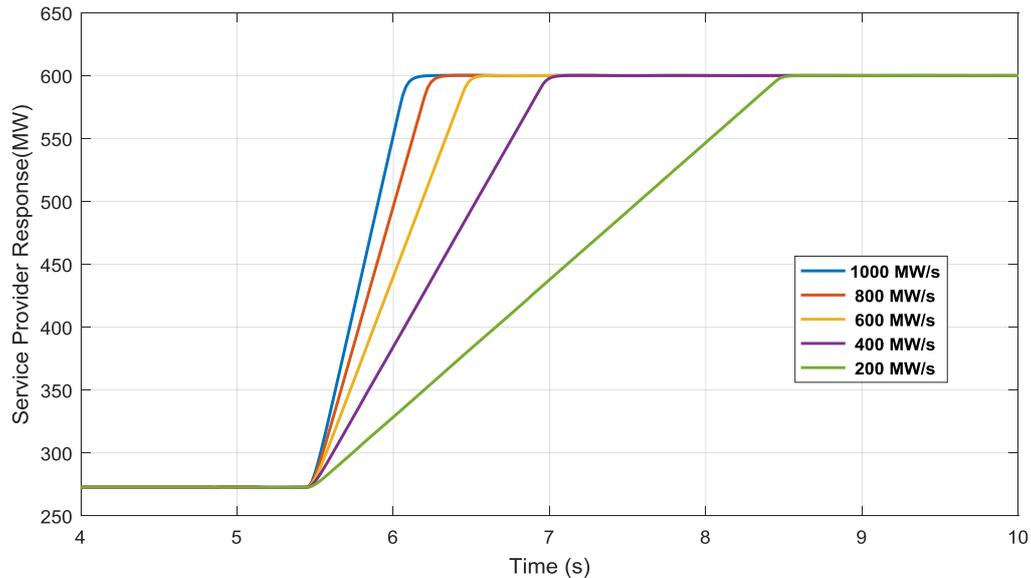
Figure 4-47 Actual service provider response with different ramping rates
