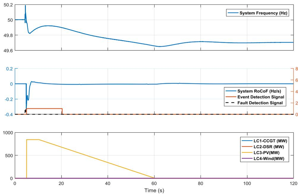
Figure 4-37 System frequency of generator tripping (Asyn at bus 5) after fault at bus 5 in zone 1
