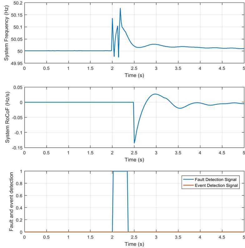
Figure 4-15 Simulation result of 140 ms Single line ground fault at Bus 3 Zone 1
