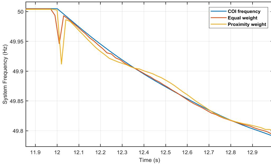
Figure 4-40 System frequency of different PMU weight configuration (zoomed)
