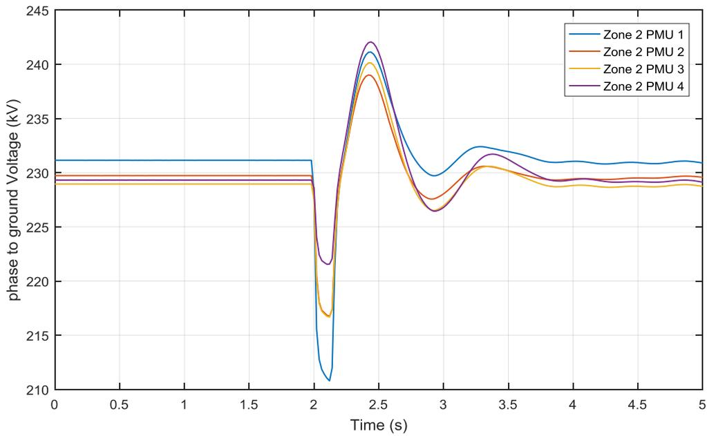
Figure 4-26 Zone 2 PMU voltages of 140 ms three phase ground fault at Bus 3 Zone 1
