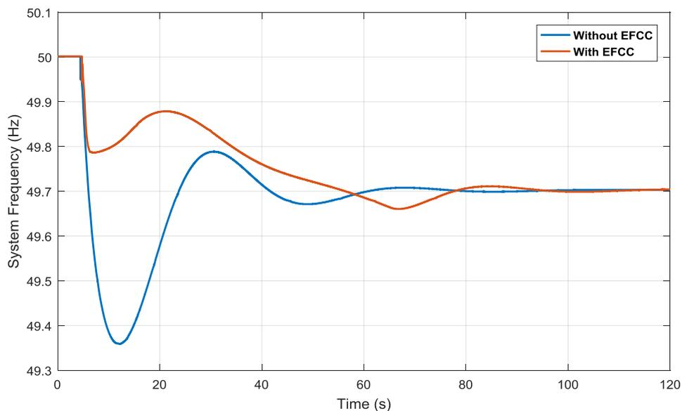
Figure 4-1 System frequency of 1000 MW load increase event at bus 9 zone 1
