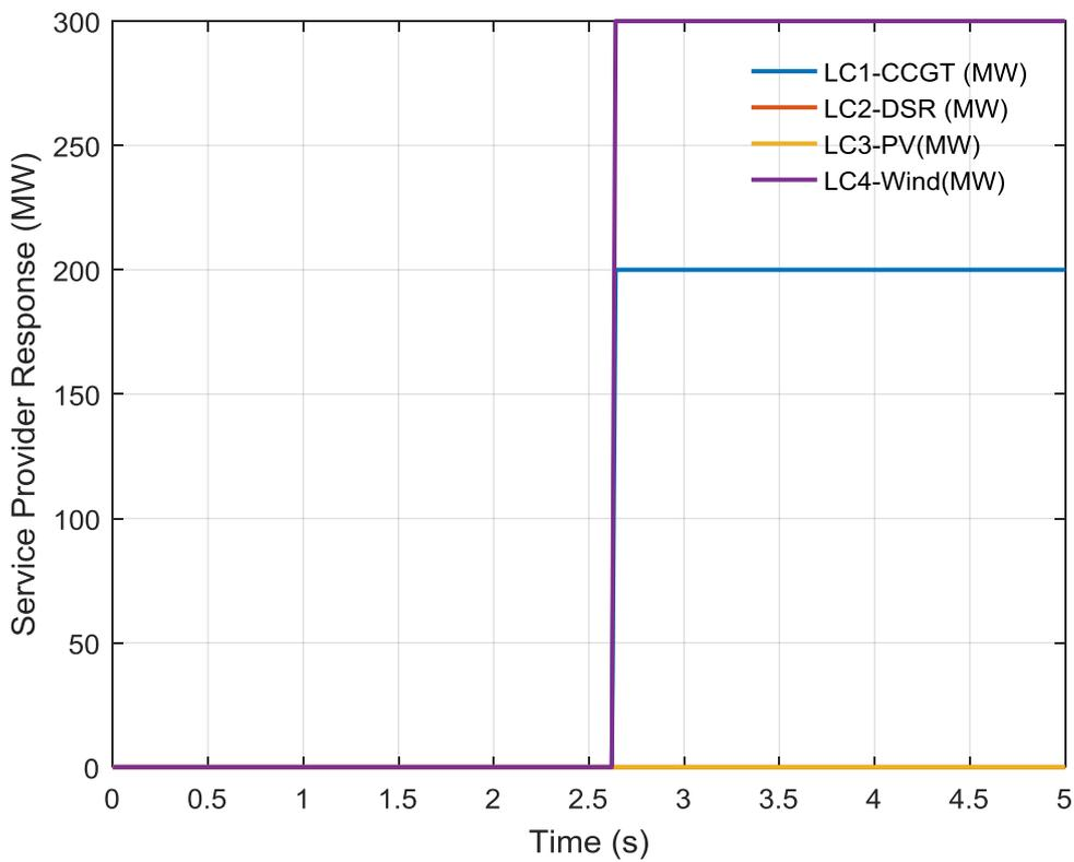
Figure 4-30 Event detection of 140 ms three phase ground fault of 1500 MW load increase at Bus 16 Zone 2
