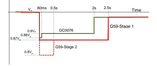
Fig 1: Stage 1 and Stage 2 Protection Requirement in ER G59 for Under-Voltage Protection and GC0076 Requirement for Pre-Event Voltage at Nominal Level
