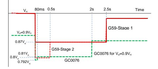
Fig 2: Stage 1 and Stage 2 Protection Requirement in ER G59 for Under-Voltage Protection and GC0076 Requirement for Pre-Event Voltage at 90% of Nominal
