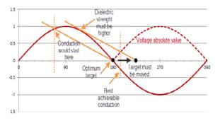
Figure 10 : Effects of the RDDS on the switching point
