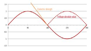
Figure 9 : Importance of the RDDS for capacitor banks
