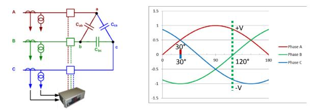
Figure 3 : Effects of the CB repeatability on the inrush current
