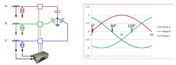
Figure 1 : Energization of a Yg capacitor bank
