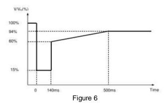
V/VN is the ratio of the actual voltage on one or more phases at the LV Side of the Offshore Platform to the nominal voltage of the LV Side of the Offshore Platform.
