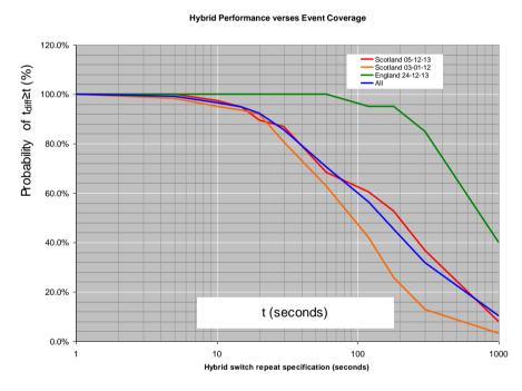
Figure 6: Probability of time difference between two successive events during a storm being greater than a specific value
