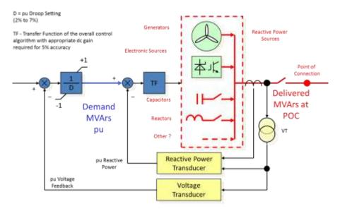
Figure 1: Typical Voltage Control Methodology
