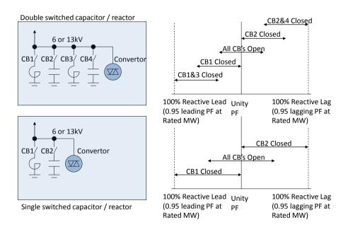
Figure 2: Typical SVC Steady State Operating Methodology
