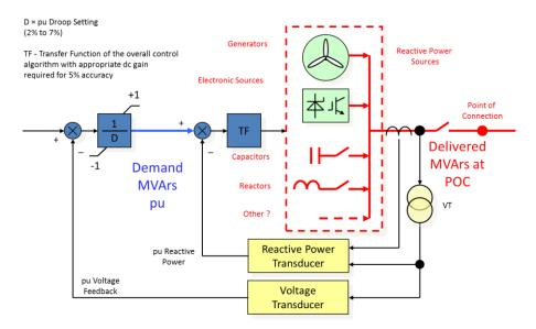
Figure 1: Typical Voltage Control Methodology
