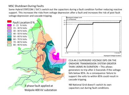
Figure 15: Voltage Depression and MSC Shutdown during Faults
