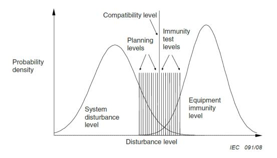
Figure 1 — Illustration of EMC concepts relevant to system
