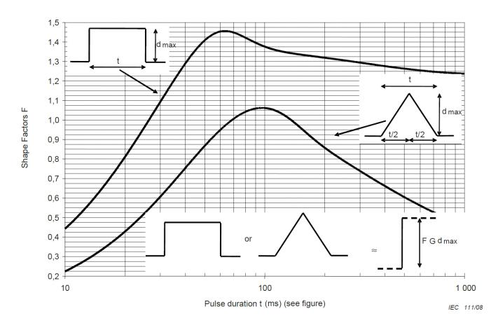
Figure B.2.1 — Shape factor curve for pulse and ramp changes
