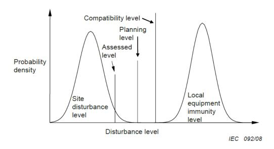
Figure 2 — Illustration of EMC concepts relevant to local site
