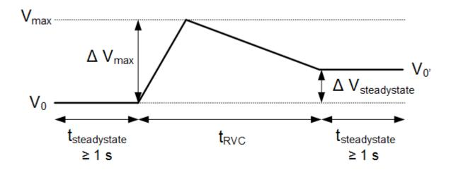
Figure 4 — Illustration of RVC characteristic for voltage swell
