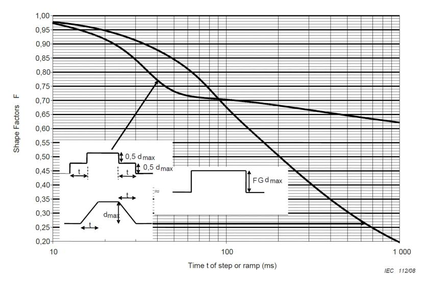
Figure B.2.2 — Shape factor curve for double-step and double-ramp changes
