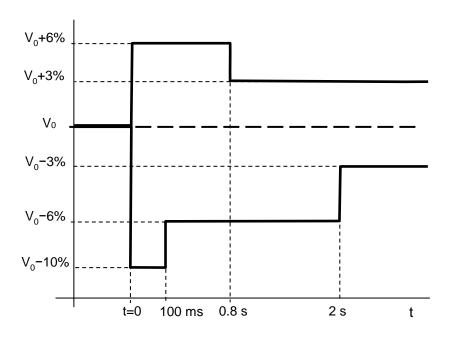
Figure 6 — Voltage characteristic for infrequent events
