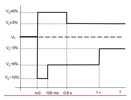
Figure ECC.6.1.7 (2) — Voltage characteristic for infrequent events
