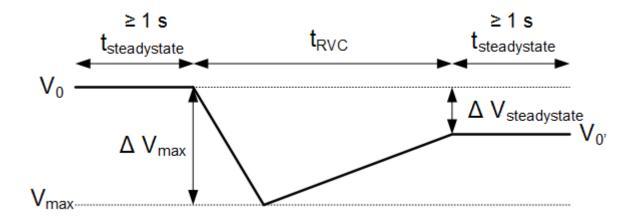
Figure 3 — Illustration of RVC characteristic for voltage dip
