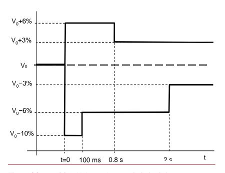
Figure CC.6.1.7 (2) — Voltage characteristic for infrequent events
