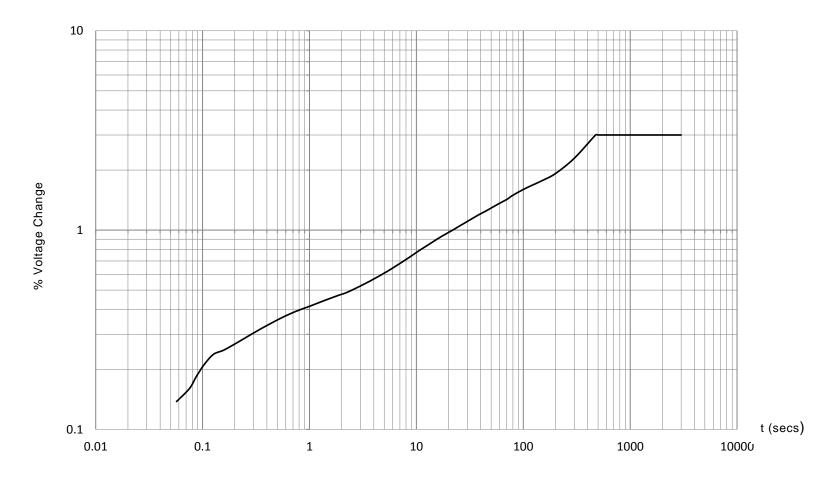
a) Minimum time interval between voltage changes
