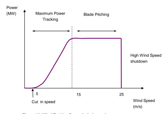
Figure 10: Wind Turbine Power / wind speed curve
