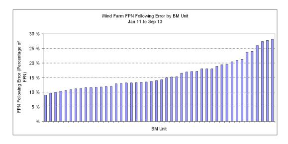
Figure 6: PN following accuracy by Wind BM Unit (Jan 2011 – Sept 2013)
