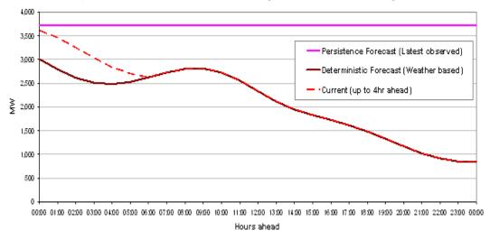
Figure 8: Wind Power forecast combining deterministic and persistence methodologies
