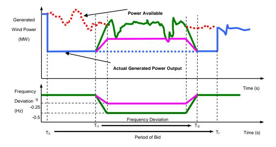
Figure 3: Example of low frequency response from wind generation
