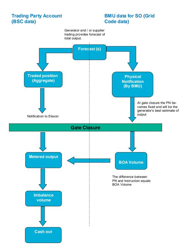
Figure 9: High Level Illustration of BSC and Grid Code data flows
