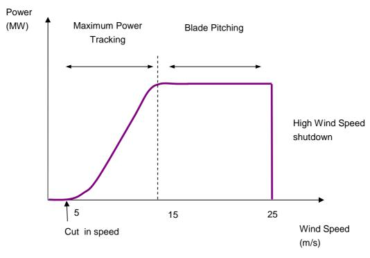
Figure 10: Wind Turbine Power / wind speed curve
