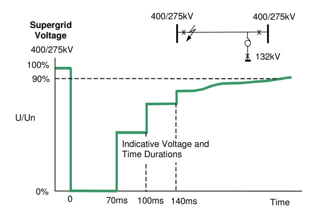
Typical fault cleared in 140ms:- 3 ended circuit
