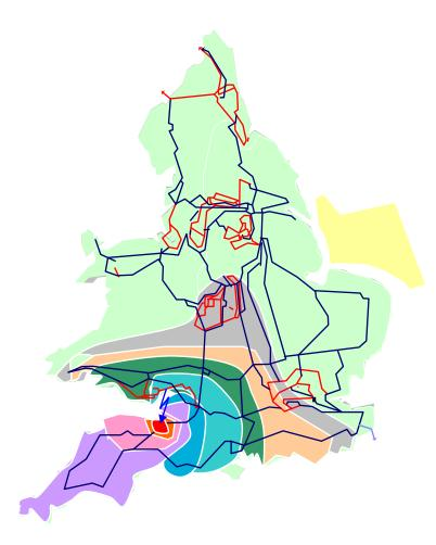
Example - 3 phase fault at Shurton 400 kV substation
