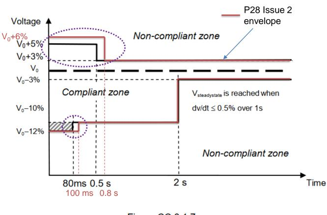
Figure CC.6.1.7 -Time and magnitude limits for a category 3 Rapid Voltage Change Key differences with Grid Code CC 6.1.7
