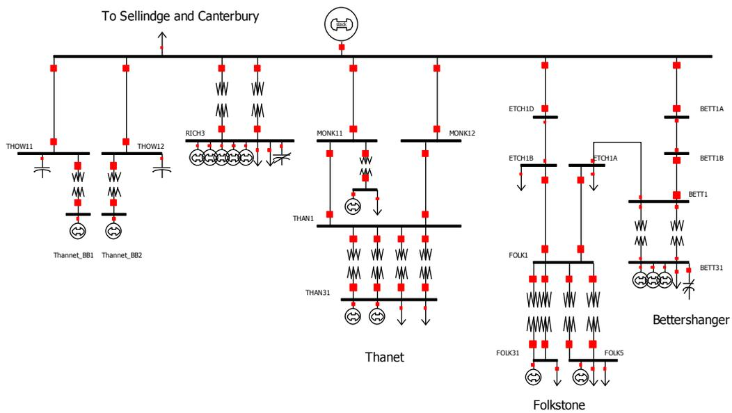
Figure 3-14 132 kV and part of 33 kV distribution network in Richborough
