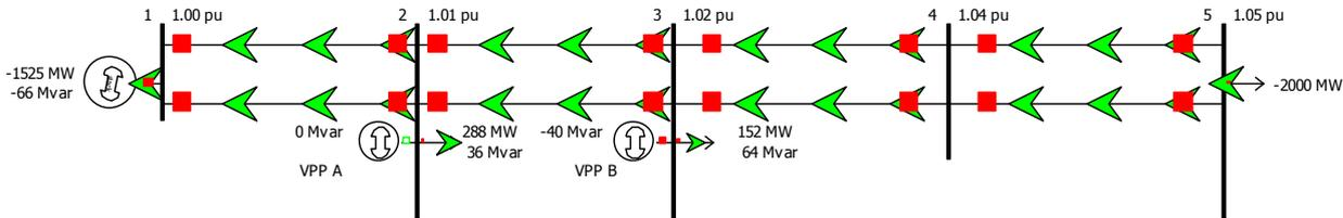
Figure 2-13 Solving the over-voltage problem using 40 Mvar absorption from VPP B
