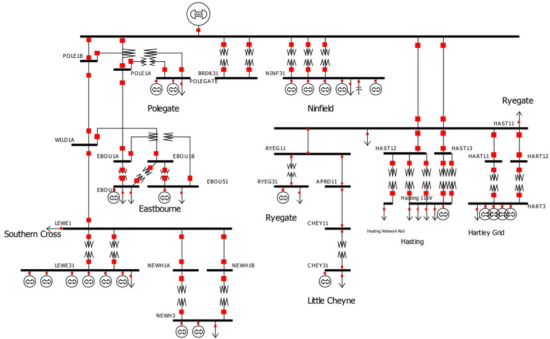
Figure 3-5 Reduced model of the Ninfield distribution network
