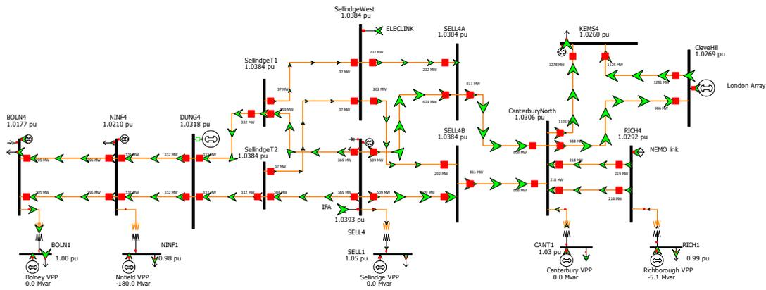
**Figure 4-8 Solving network congestion problem using a combination of the transmission connected generators and VPPs**
