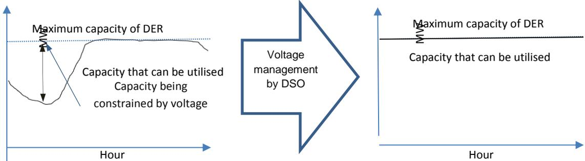
**Figure 1-1. An illustrative example of the increased role of DSO to enable full access to DER capacity to provide transmission services**
