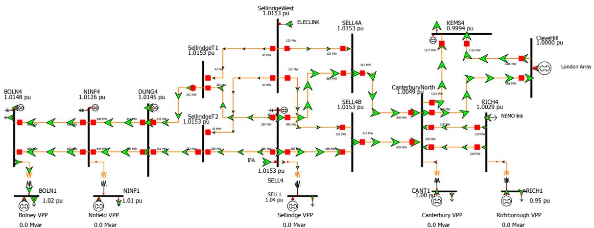
Figure 4-1 South-East GB transmission test system
