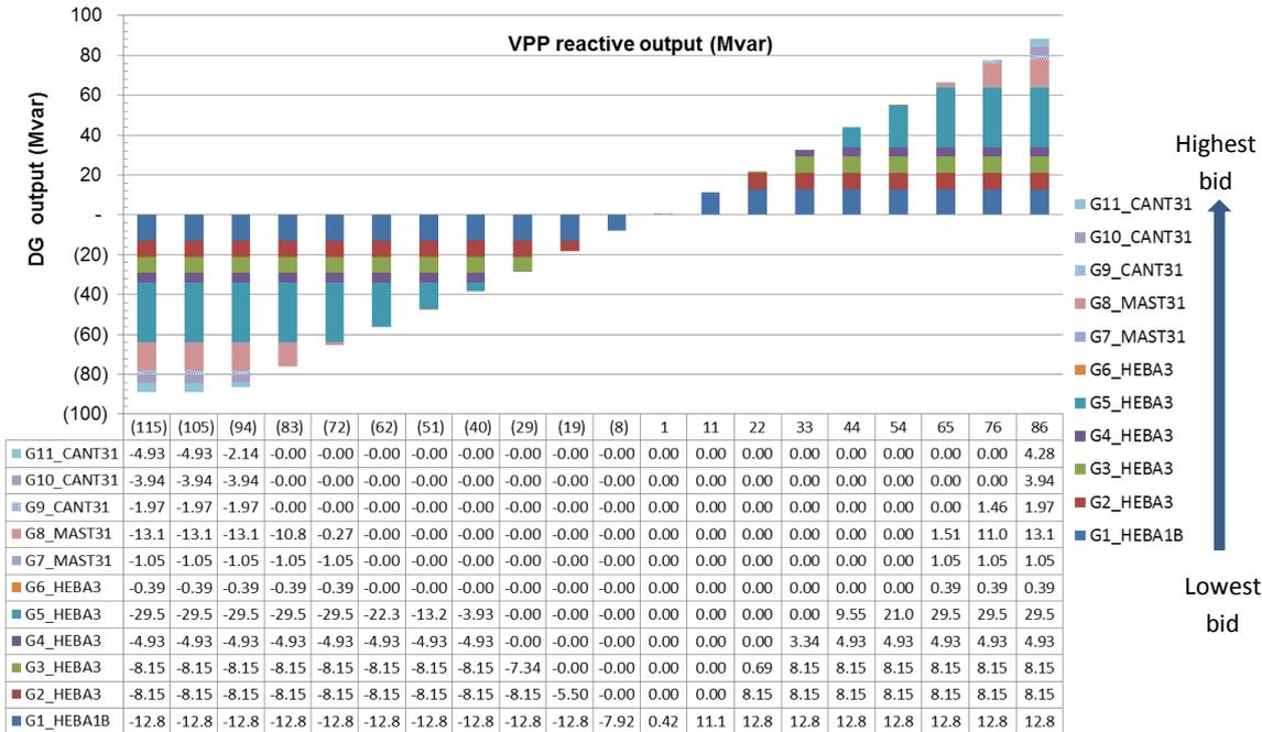
Figure E. 12 Reactive power dispatch of each DER in Canterbury VPP
