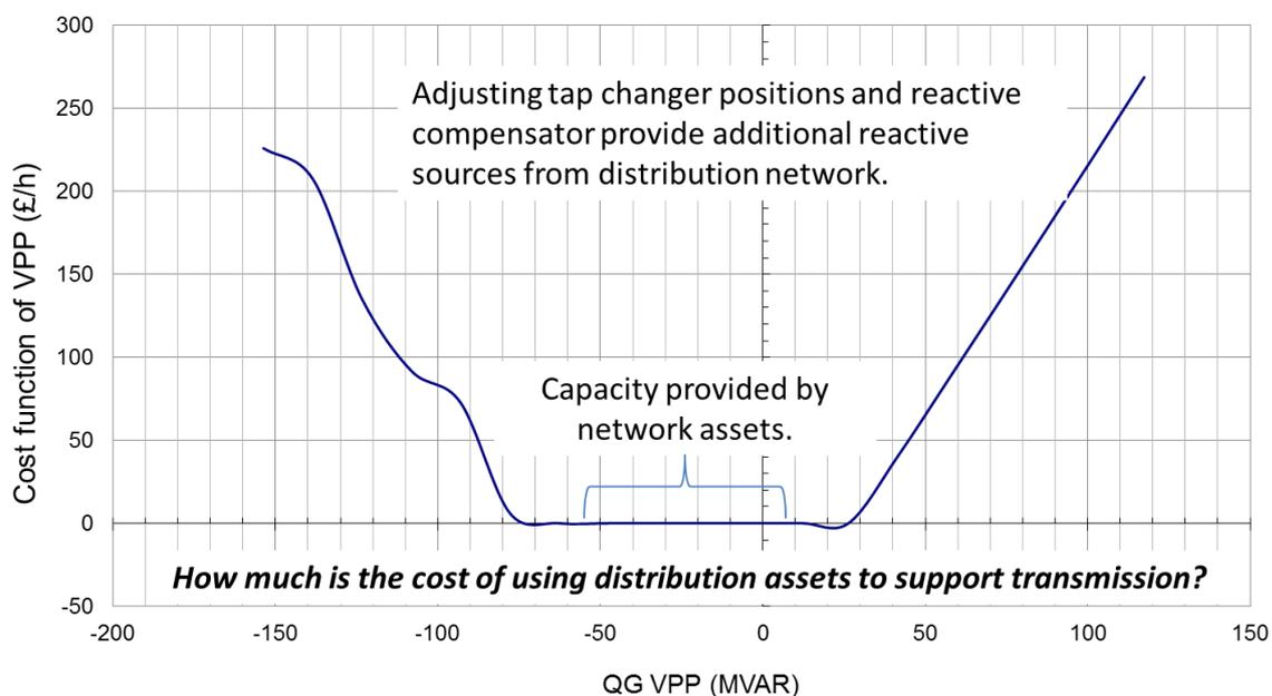
**Figure 3-17 Mvar cost function [Bolney VPP] with optimised tap changers and distribution reactive assets**
