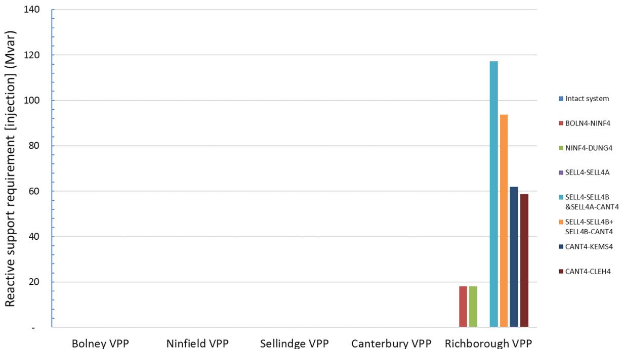
**Figure 5-5 Reactive power requirement in different system conditions**
