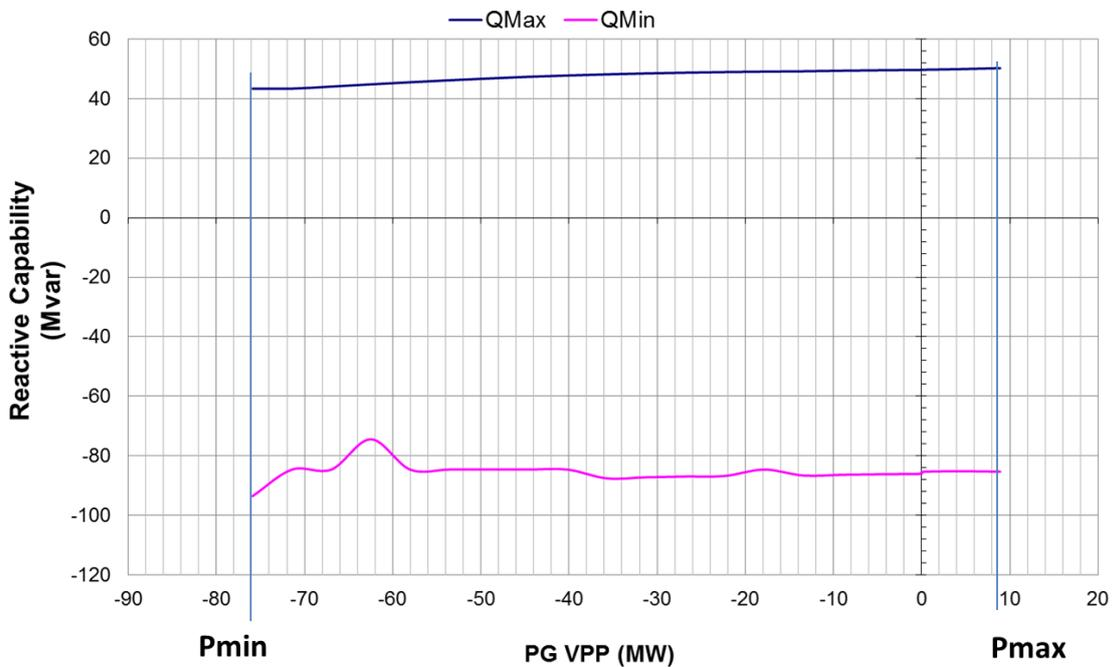
**Figure 3-9 PQ curve of the Sellindge VPP**
