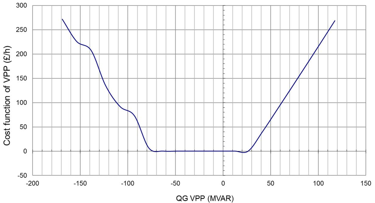
**Figure 3-4 Reactive power cost function of Bolney VPP**
