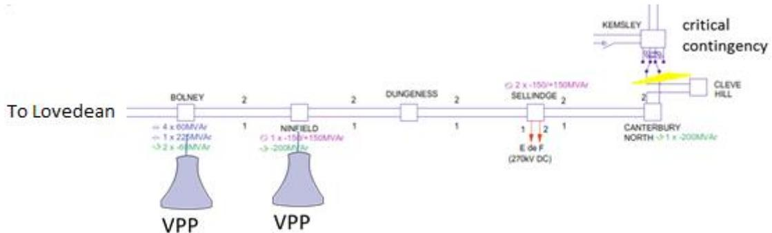
Figure 2-5 South-East transmission system model
