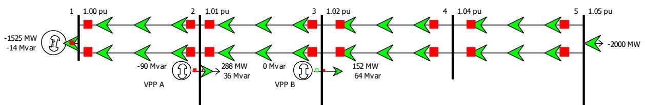
Figure 2-12 Solving the over-voltage problem using 90 Mvar absorption from VPP A
