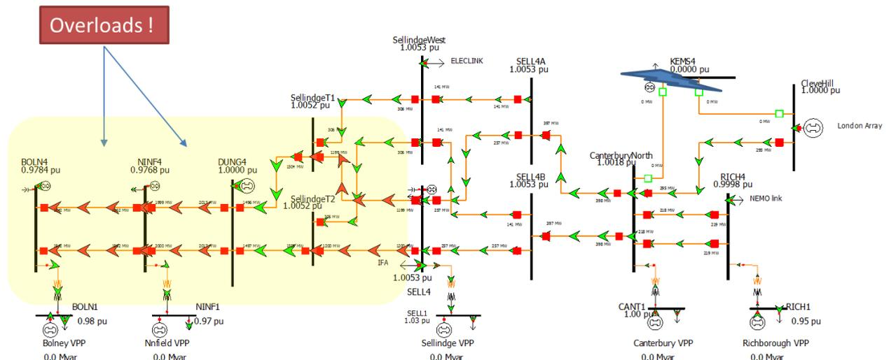
**Figure 4-2 Network congestion problem caused by a double circuit outages**
