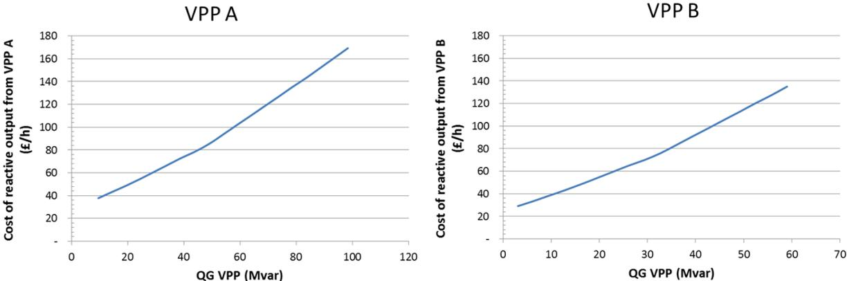
Figure 2-14 Cost function of reactive power services (injection) from VPP A and VPP B during peak demand<sup>7</sup>
