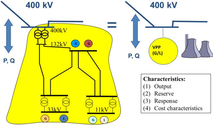
**Figure E. 6 VPP as a flexible representation of the aggregated DER and networks**
