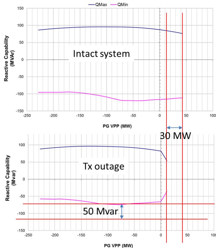
**Figure E. 11 Impact of a transformer outage on the PQ curve capability of Canterbury VPP**
