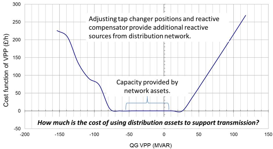
**Figure E. 8 Mvar cost function [Bolney VPP] with optimised tap changers and distribution reactive assets**
