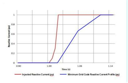
Figure ECC4.4 – Injected Reactive Current from Power Park Module
