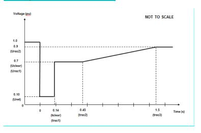
Figure ECC.6.3.15.3 - Voltage against time curve applicable to **Type C** and **D Synchronous Power Generating Modules** connected below 110kV
