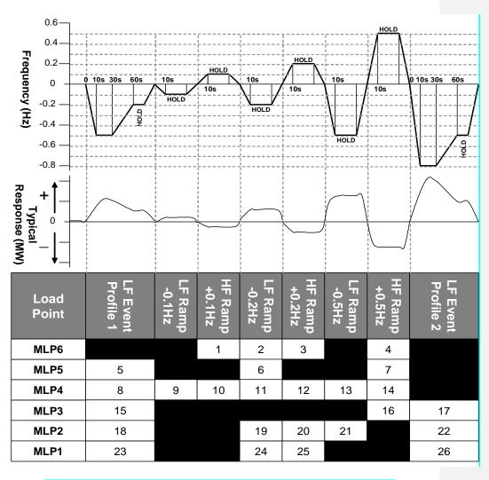
Figure 1: Frequency Response Capability FSM Ramp Response Tests
