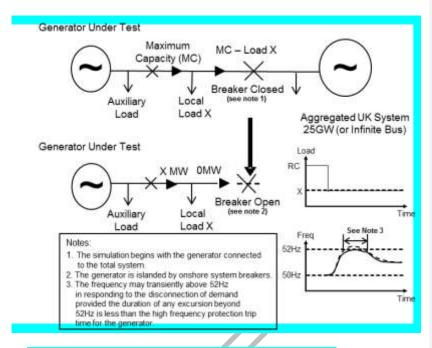
Figure ECP.A.3.6.1 - Diagram of Load Rejection Study
