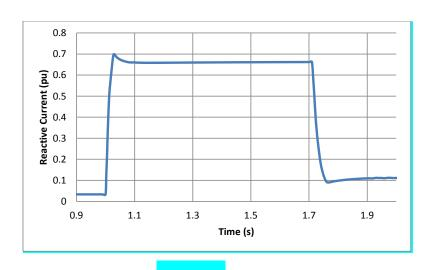
Figure ECC4.5 Reactive Current Injected for a 50% voltage dip for a period of 710ms
