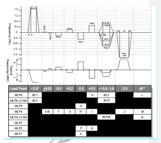
Figure 2: Frequency Response Capability LFSM-O, LFSM-U and FSM Step
