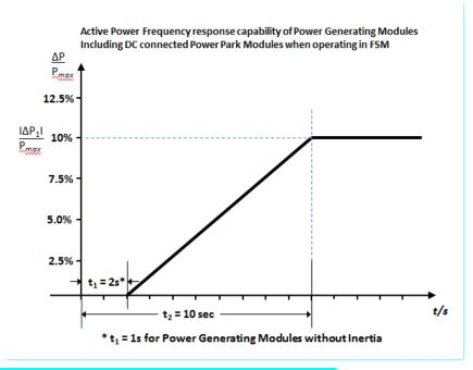
Figure 6.3.7.3.3(b) Active Power Frequency Response capability.
