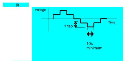
ECP.A.6.5 Figure 1 – Transformer tap sequence for voltage control tests
