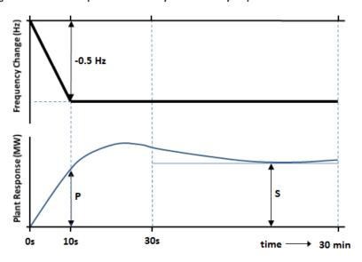
Figure ECC.A.3.3 - Interpretation of High Frequency Response Service Values
