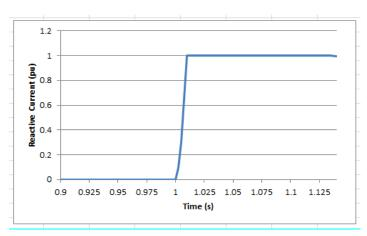
Figure ECC4.2(b) – Reactive Current Injected from the Power Park Module connected to Substation C
