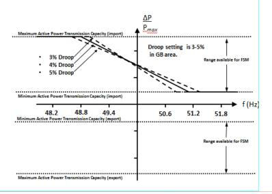
Figure 6.3.7.3.4(a) – **Active Power** frequency response capability of a **HVDC System** operating in **Frequency Sensitive Mode** (FSM). ΔP is the change in active power output from the **HVDC System**..
