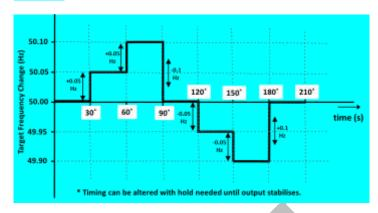
ECP.A.6.6. Figure 3 - Target Frequency setting changes
