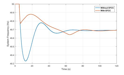
• The lowest frequency is improved from 49.33 Hz to 49.64 Hz
