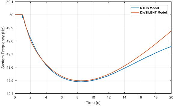
Validation of the 26 Zone GB network represented in RTDS against the GB 36 Zone network simulated using PowerFactory (model based on scenario year 2020)
