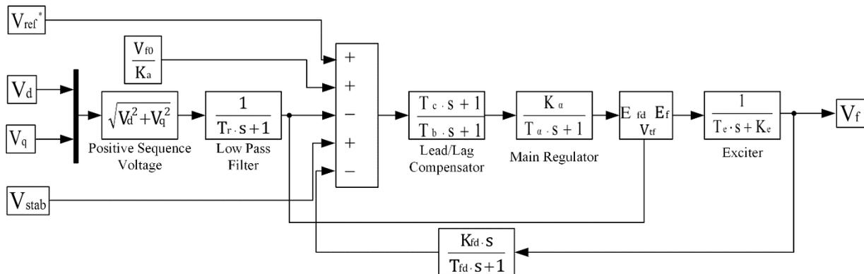
Figure 4. IEEE Type 1 Excitation System Block Diagram
