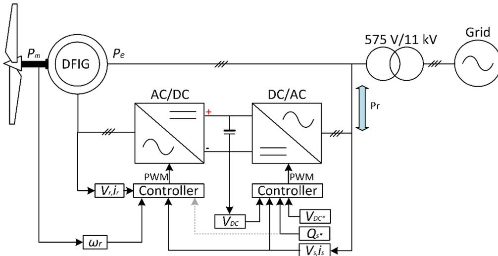
Figure 6. DFIG Model connected to 11kV Network
