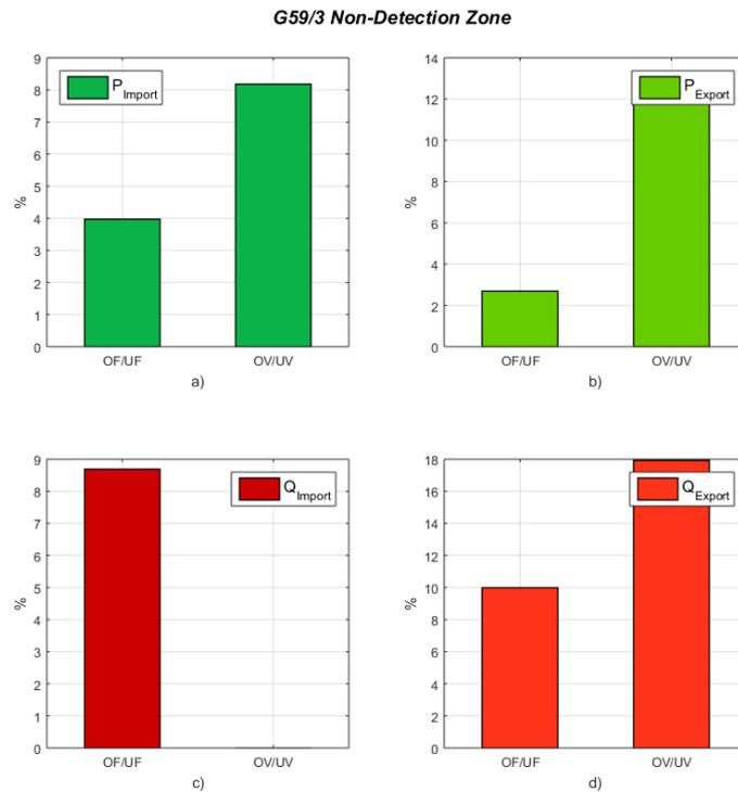
**Figure 31. OF,UF,OV,UV NDZs for Generation Mix 3, a) Active power import, b) Active power export, c) Reactive power import, d) reactive power export**
