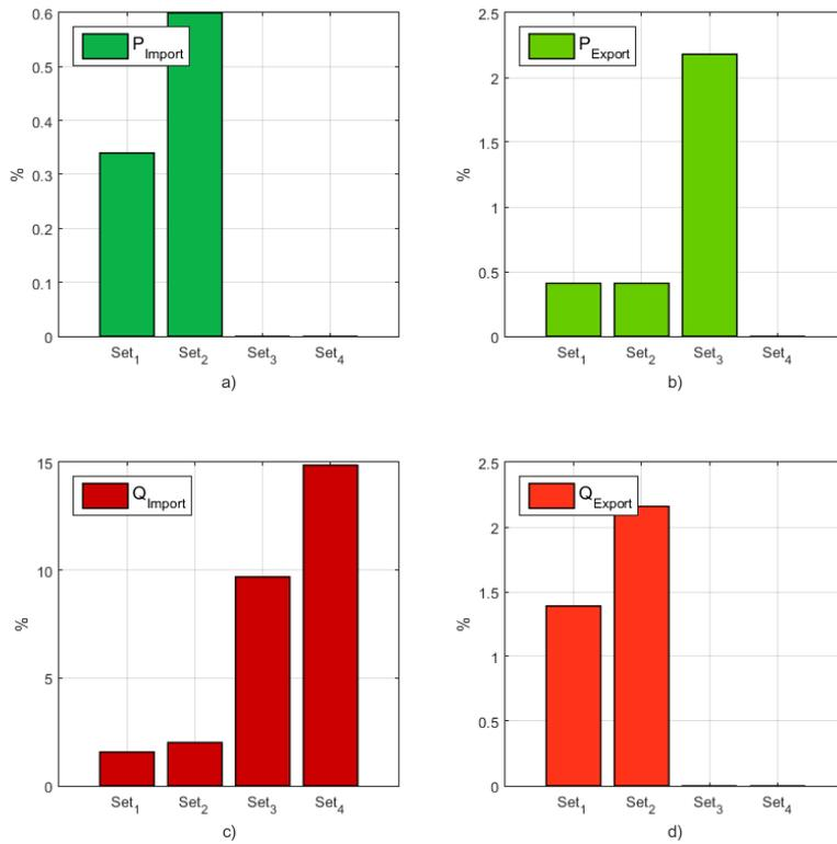
**Figure 44. ROCOF NDZs for Generation Mix 10, a) Active power import, b) Active power export, c) Reactive power import, d) reactive power export**
