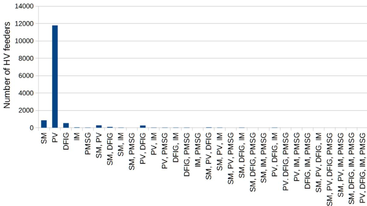
Figure 14. Islanding groups at the HV feeder level (Scenario 2)
