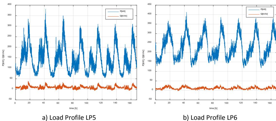
**Figure 21. Two LV switchboard recorded profiles (ENW) – February 2015**
