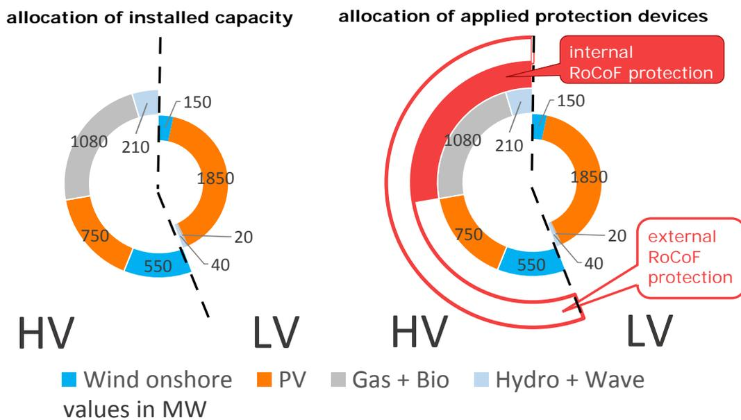
**Figure 17. Indicative illustration of technology shares (<5 MWe) per voltage level (left) and potential application of ROCOF protection (right), HV: high voltage level, LV: low voltage level, internal ROCOF: protection is part of the genuine plant control, external ROCOF: protection by separate devices at the point of common coupling, year: end of 2013 [10]**
