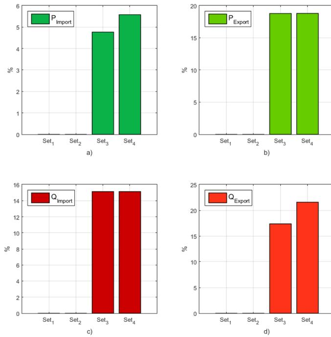
**Figure 36.ROCOF NDZs for Generation Mix 6, a) Active power import, b) Active power export, c) Reactive power import, d) reactive power export**
