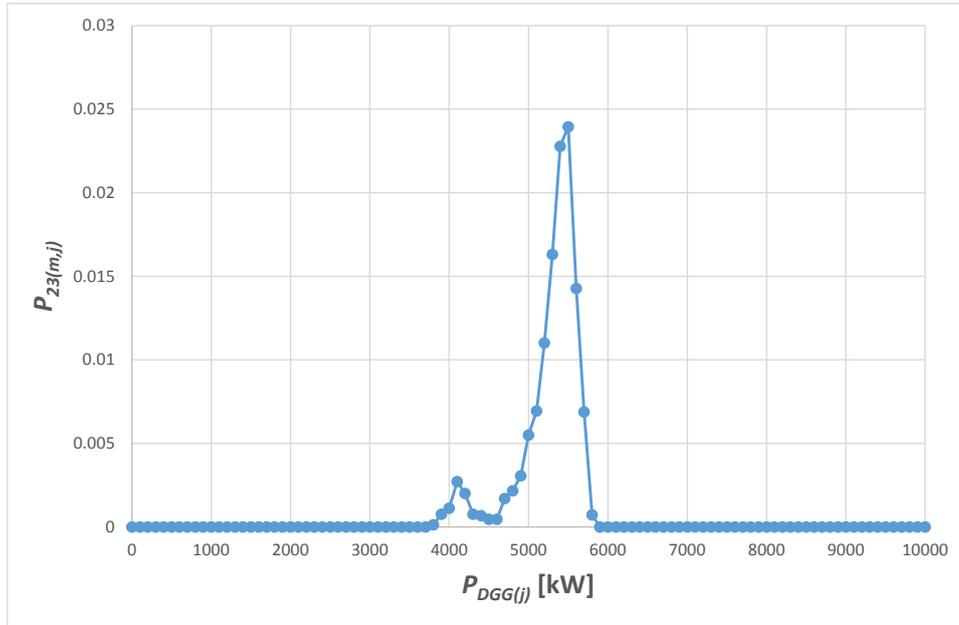
**Figure 11. Non-detection zone probability at varying DG group capacity**
