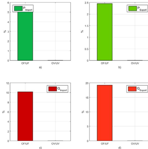
**Figure 45. OF,UF,OV,UV NDZs for Generation Mix 10, a) Active power import, b) Active power export, c) Reactive power import, d) reactive power export**
