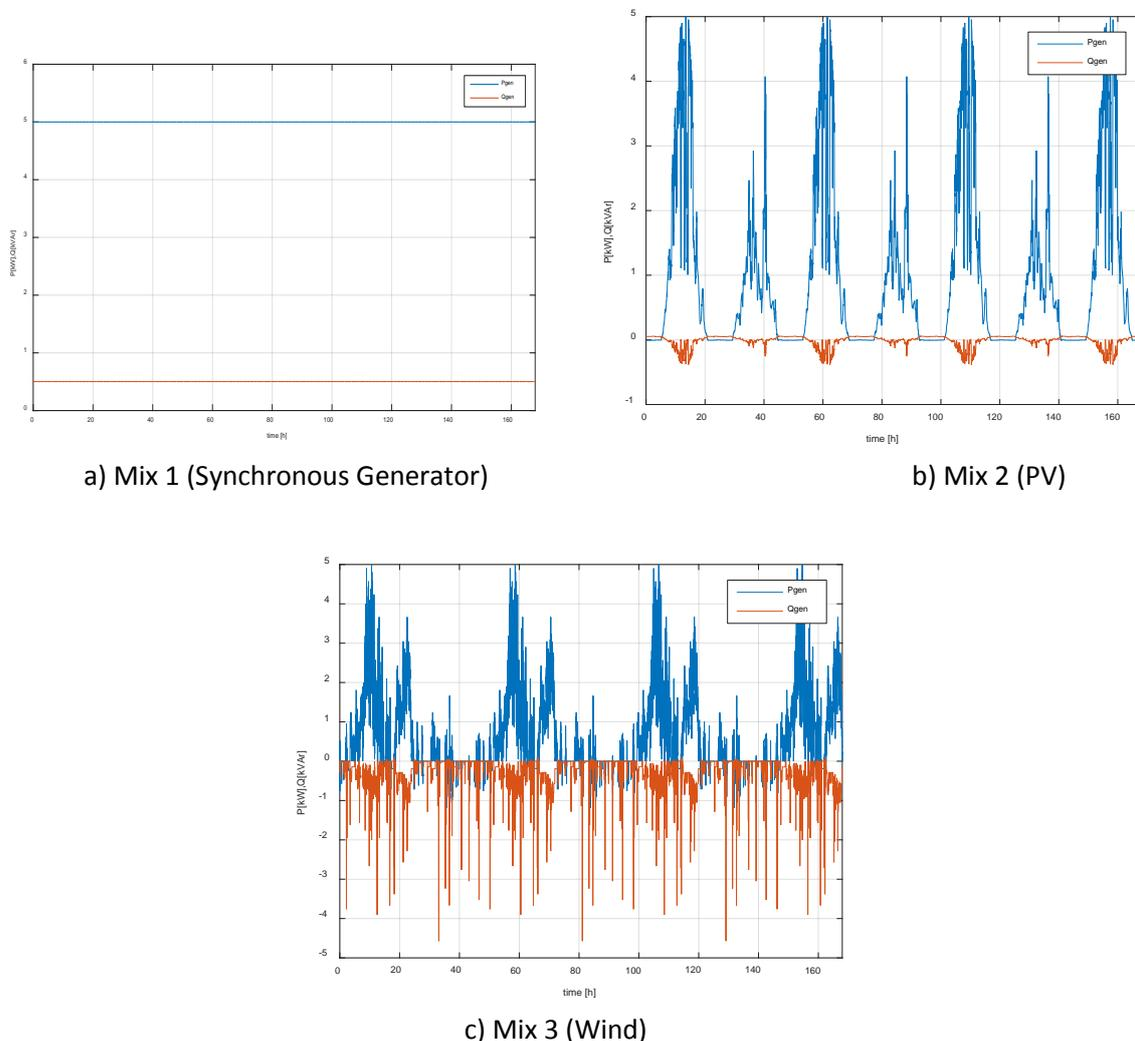
**Figure 22. Example load profiles from individual DG technologies**
