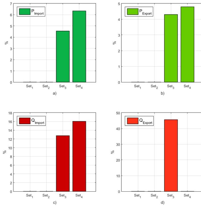
**Figure 34. ROCOF NDZs for Generation Mix 5, a) Active power import, b) Active power export, c) Reactive power import, d) reactive power export**
