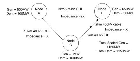
Assuming Node A is the reference node<sup>†</sup>,, each 400kV circuit has impedance X, the 275kV circuit has impedance 2X, the 400kV cable circuit expansion factor is 10 and the 275kV overhead line circuit expansion factor is 2, the DCLF transport algorithm calculates the base case power flows for Peak Security background as follows:
