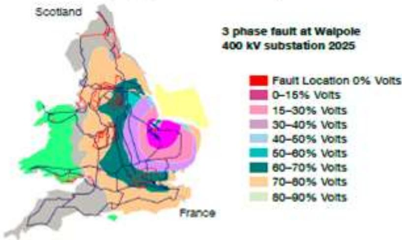
Figure 4.2(b) Effect on Voltage Profile of a solid three phase short circuit fault at Walpole 400kV substation under a high Converter Generation background
