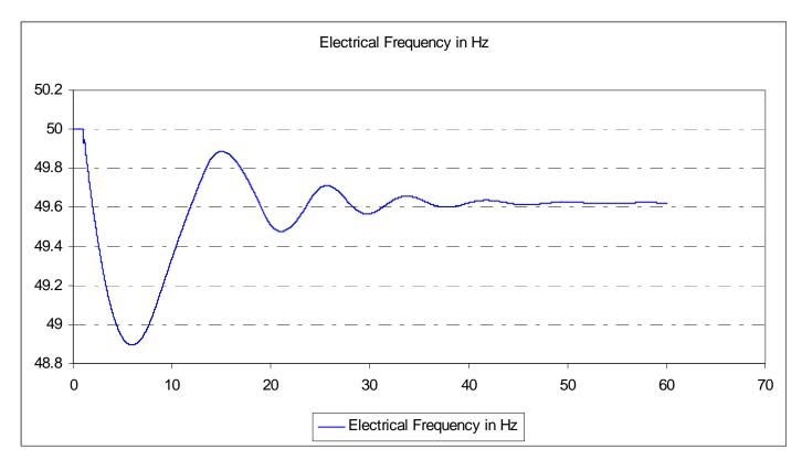
650MW of dynamic response from synchronous gens, 1200MW from wind turbines and 200MW static delivered
