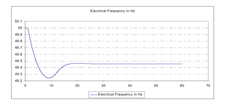
Approximately 1400MW of dynamic response and 200MW of static response delivered
