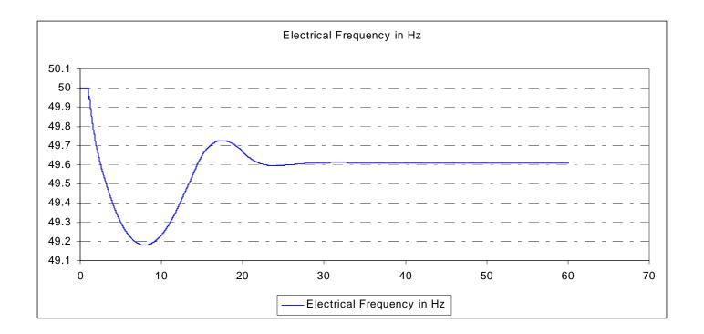
450MW of dynamic response from synchronous Gens, 1200MW from wind turbines, 200MW static response and 800MW of synthetic inertia delivered
