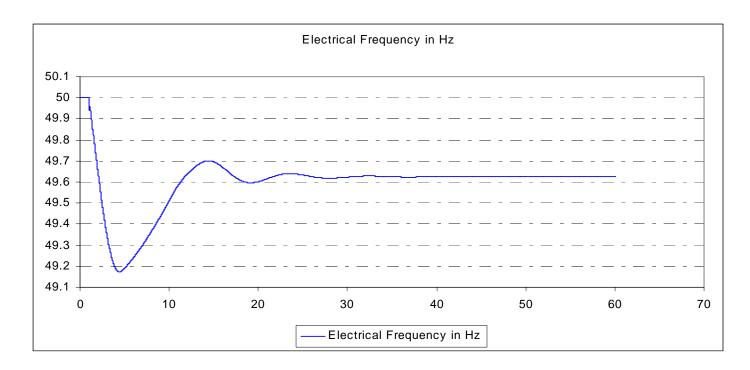
400MW of dynamic response from sync gen, 1200MW of dynamic response from wind turbines within 4 seconds and 200MW of static response.
