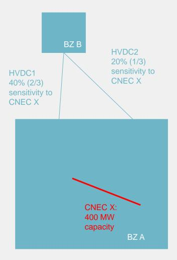
Suppose two 1000 MW HVDC interconnectors on the bidding zone border between BZ A and BZ B
