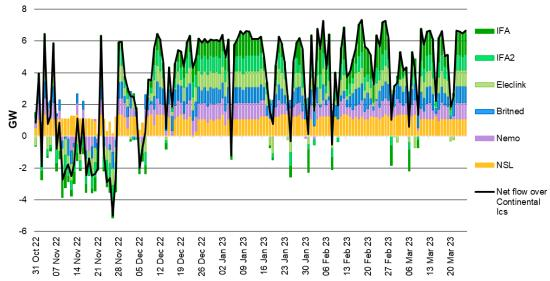
Figure 9: IFA, IFA2, BritNed, Nemo Link and NSL flow at peak times
