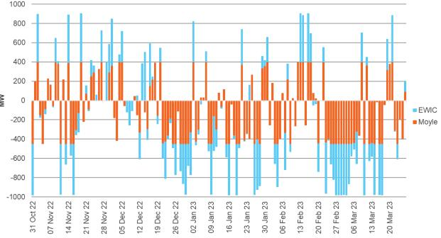
Figure 13: Stacked bar chart showing Moyle and EWIC flows at peak times (positive MW values mean flows into GB)
