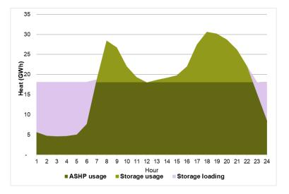
Figure 1: Thermal storage use on a peak day: hourly dispatch profiles for Air Source heat pump in Leading the Way
