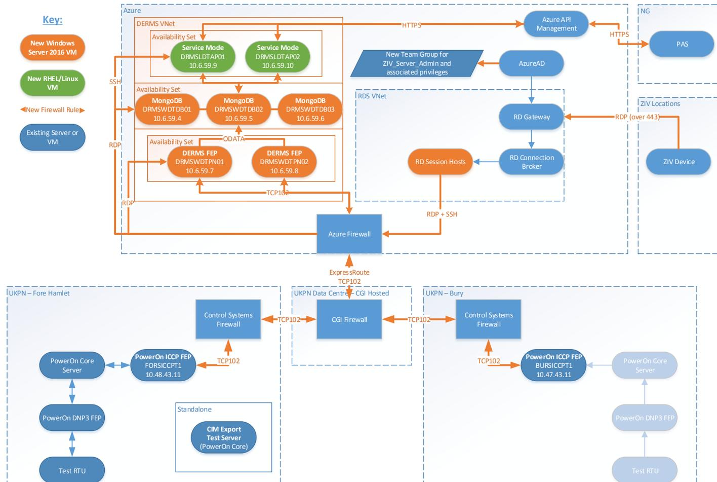
Figure 4: Azure hosting to support the pre-prod and prod environments
