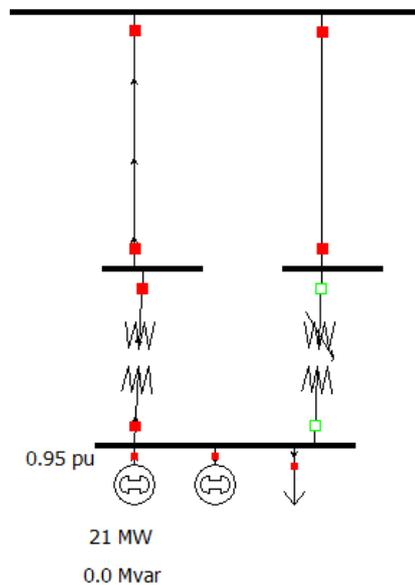
**Figure 6 A transformer circuit outage in Ninfield distribution area**
