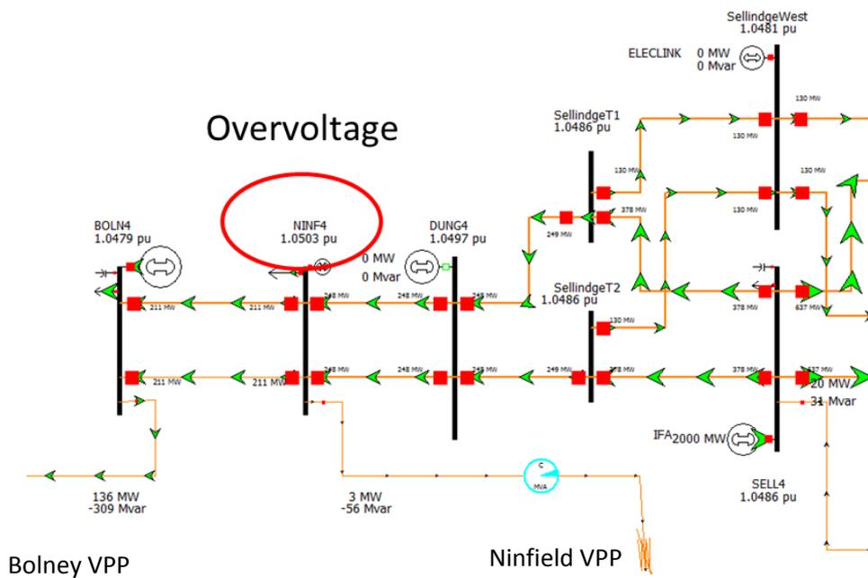
Figure 16 Overvoltage at Ninfield 400kV
