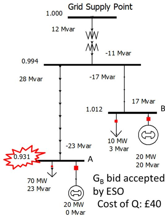
Figure 11 ESO solution to get the least-cost reactive source
