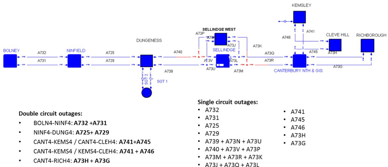
**Figure 30 Transmission system model and the list of critical single and double circuit contingencies**
