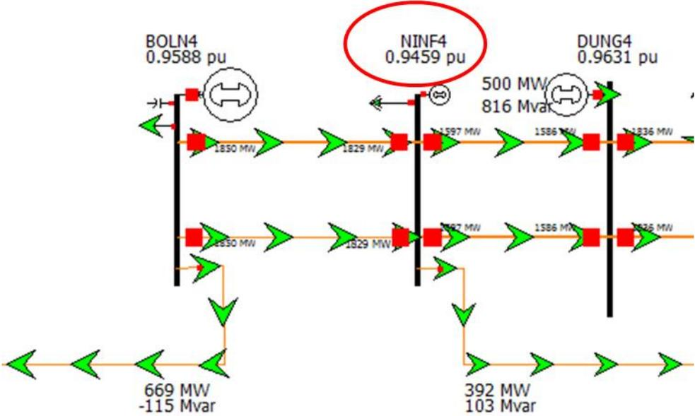
Figure 27 Undervoltage problem at the transmission
