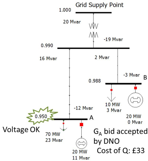
Figure 10 DSO solution for the undervoltage problem at the distribution
