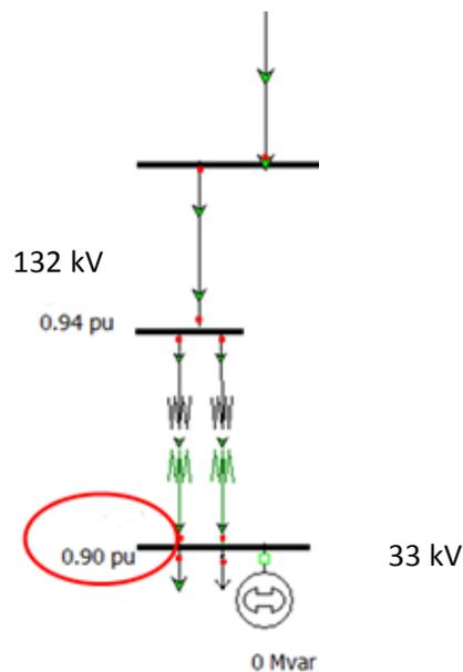
Figure 26 Undervoltage problem in Power Potential distribution grid
