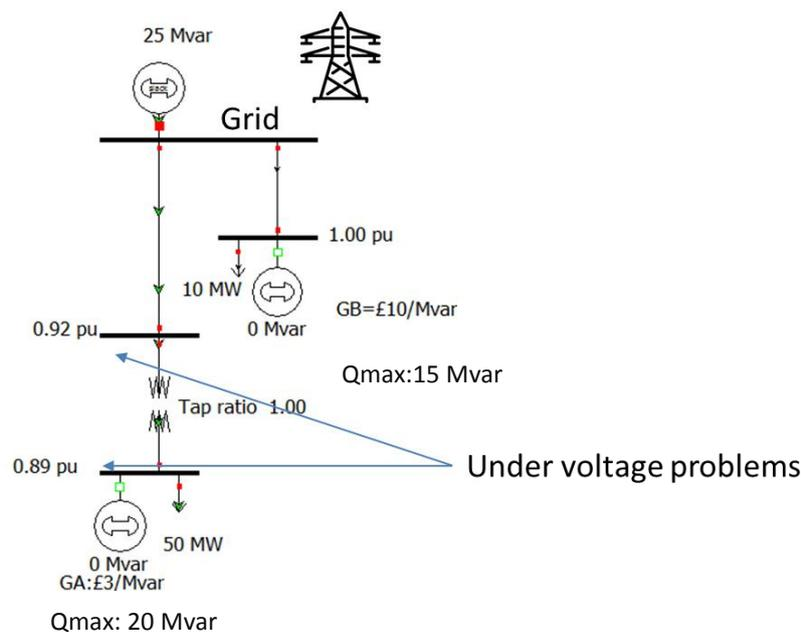
Figure 21 A simple distribution system with undervoltage problems
