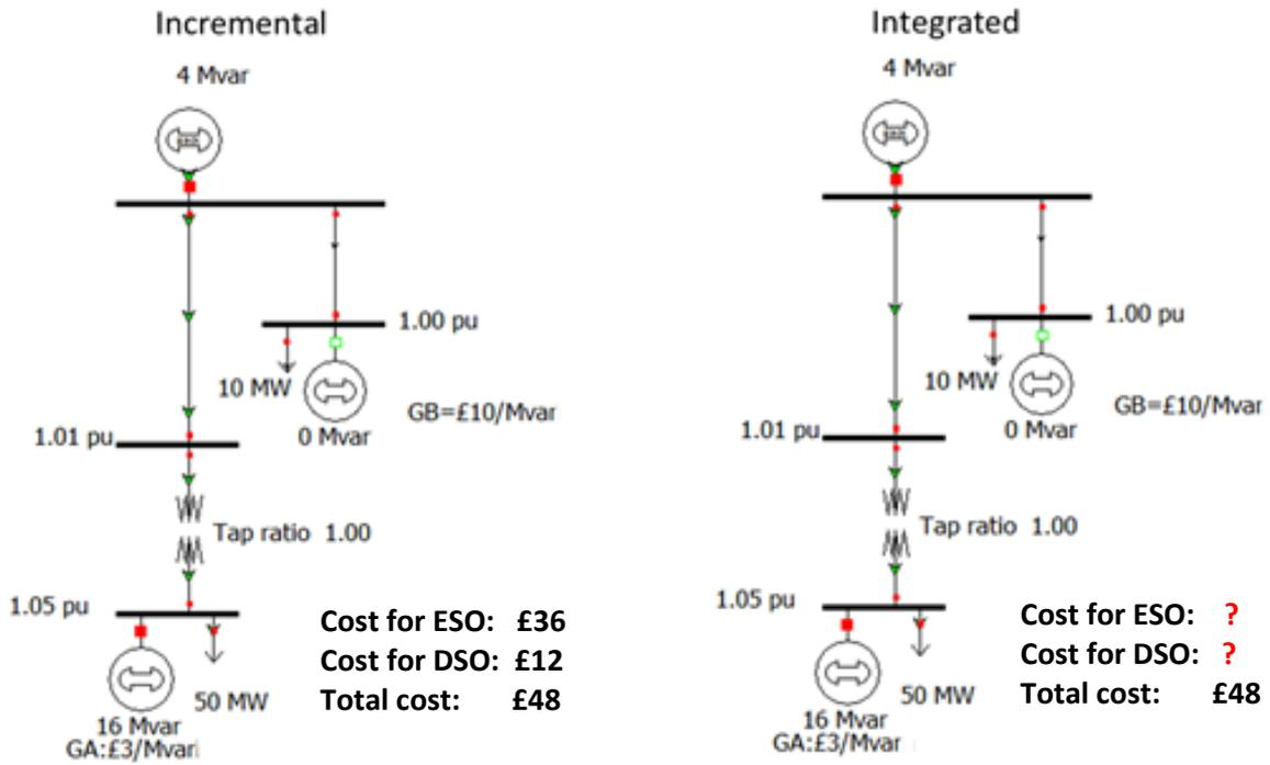
Figure 25 Comparison between the incremental and integrated solution with smart (corrective) control
