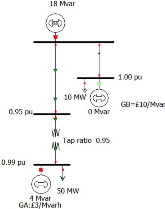
**Figure 22 The state of the distribution system after the implementation of the DSO’s solution**
