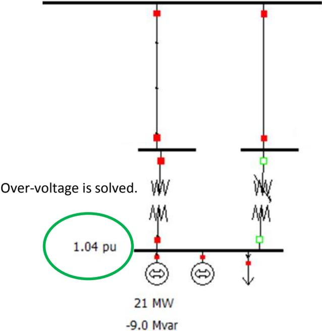
**Figure 20 Synergy of using a Power Potential unit to solve the overvoltage at the transmission and the local distribution grid**
