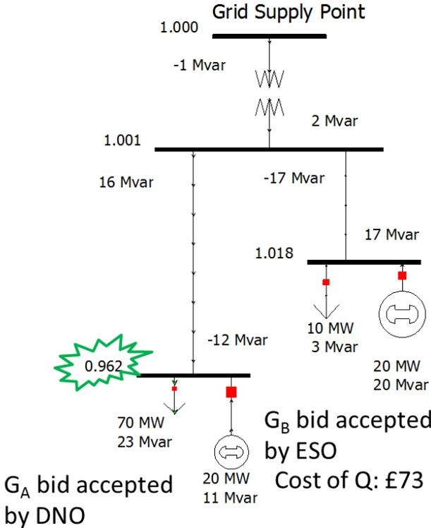
Figure 12 ESO-DSO’s no coordinated solution
