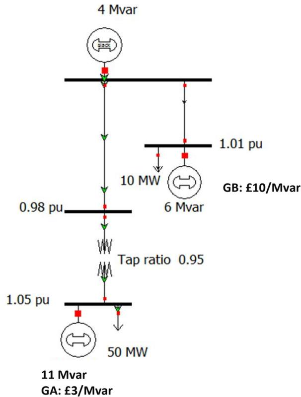
**Figure 23 DSO-ESO incremental approach solution with preventive mode**
