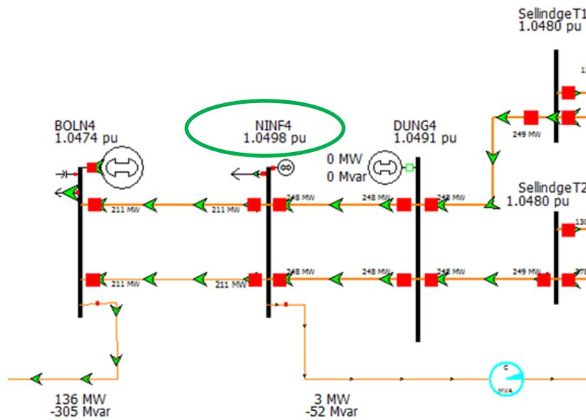
**Figure 18 A power Potential unit in Ninfield VPP is used to correct the overvoltage problem at Ninfield 400 kV**
