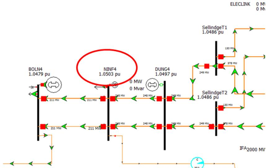
**Figure 5 An overvoltage problem at the transmission**
