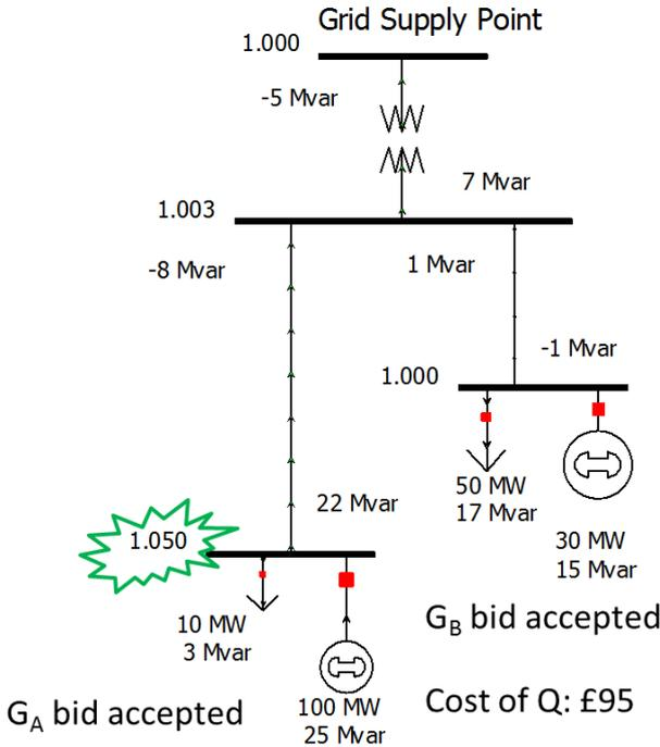
Figure 4 A solution from the Power Potential approach
