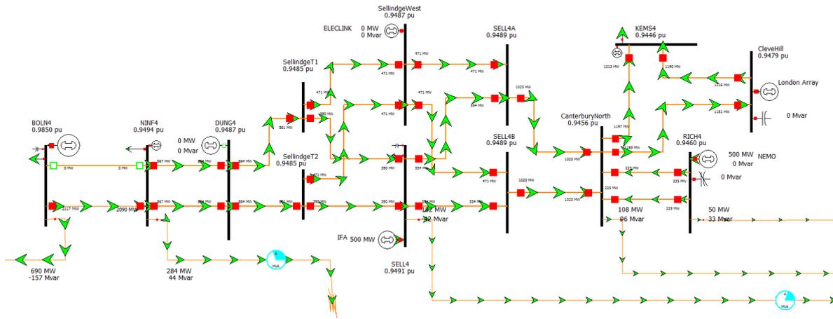
**Figure 37 A system with high demand (winter), low import, and a 400 kV circuit outage between Bolney and Ninfield**
