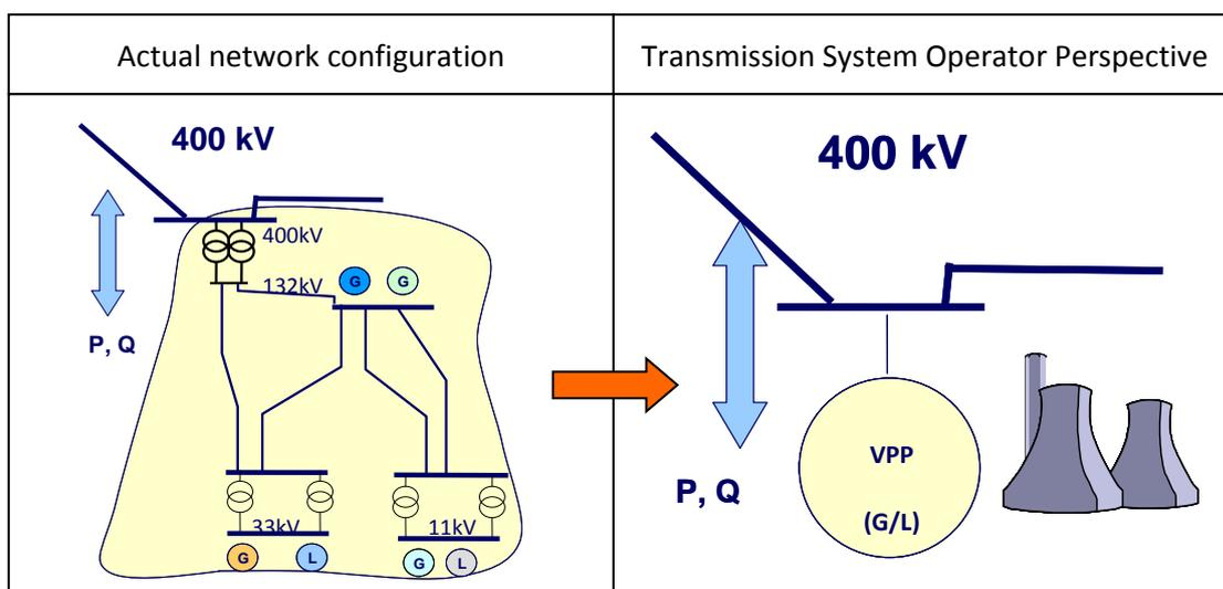
Figure 2-4 Characterisation of DER as a Virtual Power Plant
