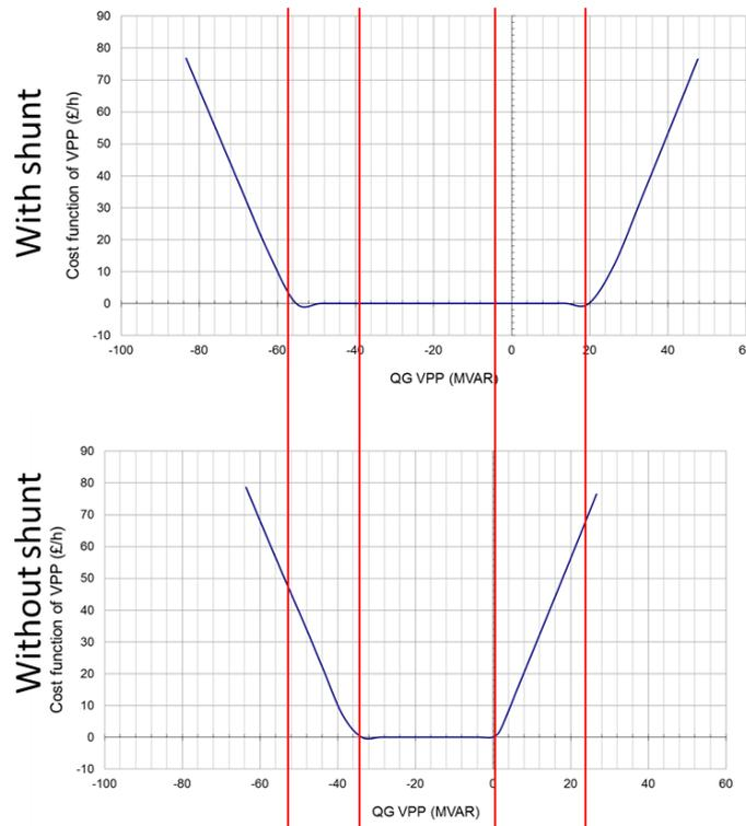
**Figure E. 9 Mvar cost function [Sellidge VPP] with and without shunt reactive compensator**
