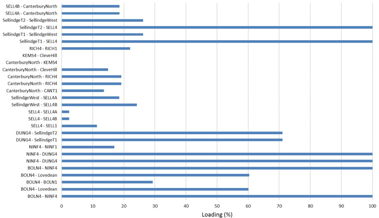
**Figure 4-4 Loading of each circuit after redispaching the output of VPP and transmission connected generators**
