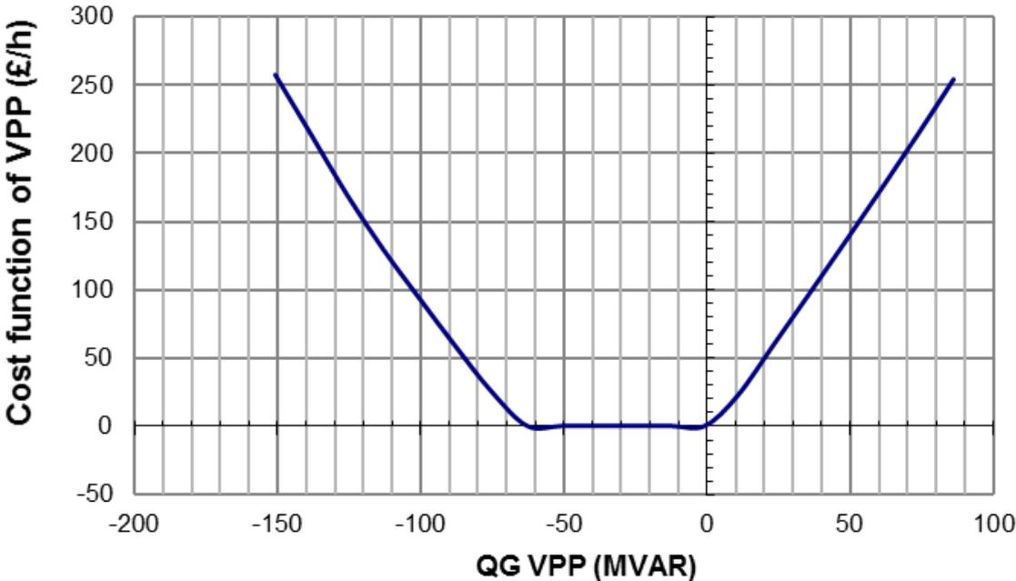
Figure 3-7 Reactive power cost function of Ninfield VPP
