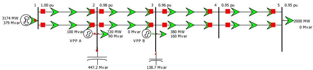
Figure 2-10 Solving the under-voltage problem using 100 Mvar from VPP A
