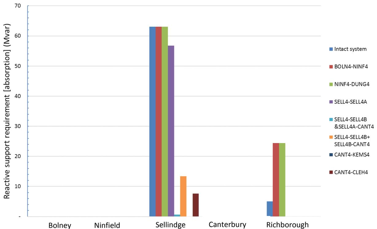
Figure 5-2 Reactive power requirement in different system conditions
