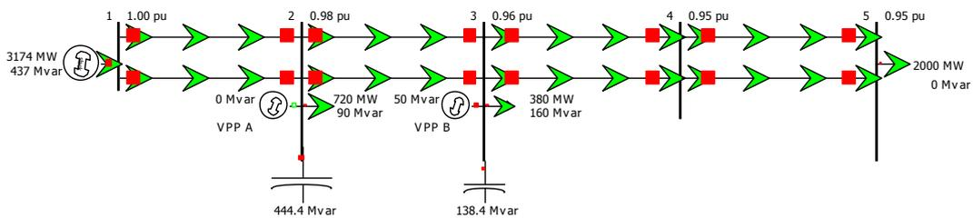
Figure 2-11 Solving the under-voltage problem using 50 Mvar from VPP B
