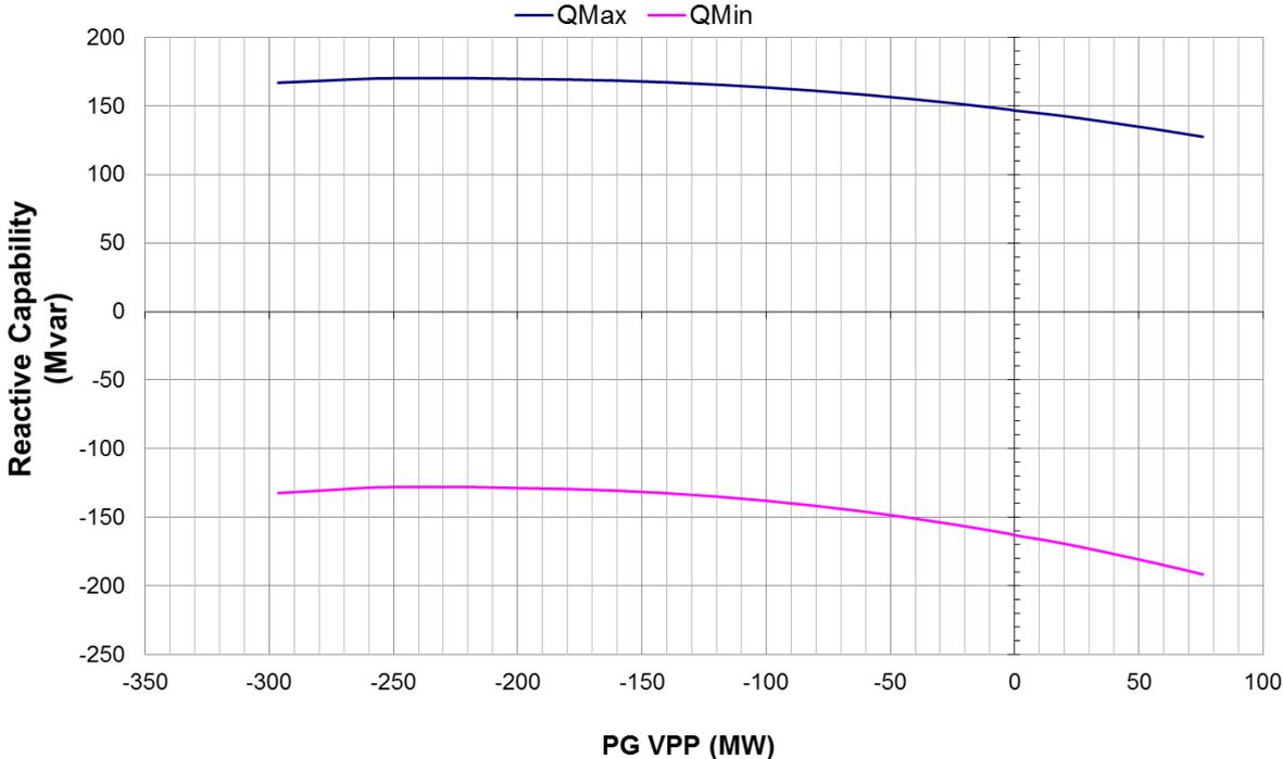
Figure 3-15 PQ curve of the Richborough VPP
