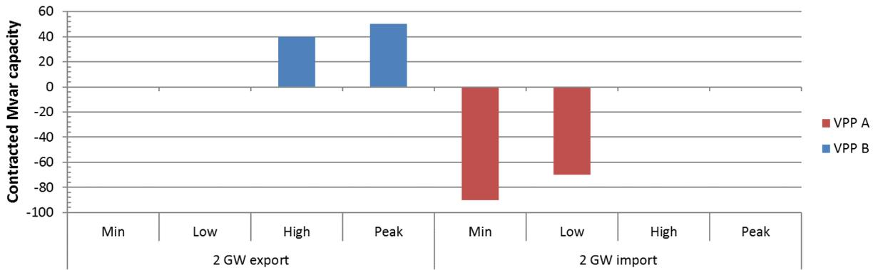
**Figure 2-16 Allocation of reactive power contract to VPP A and VPP B depending on the system conditions forecasted a day ahead**
