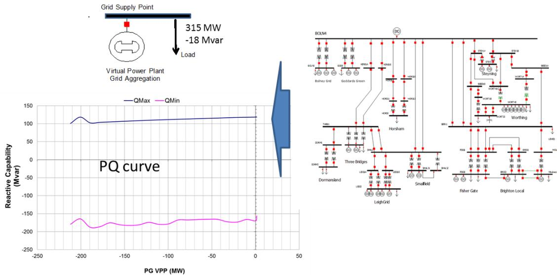
**Figure E. 7 Reactive power capability and its cost function of Bolney VPP**
