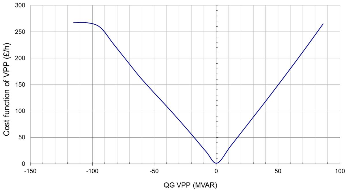
Figure 3-13 PQ curve of the Canterbury VPP
