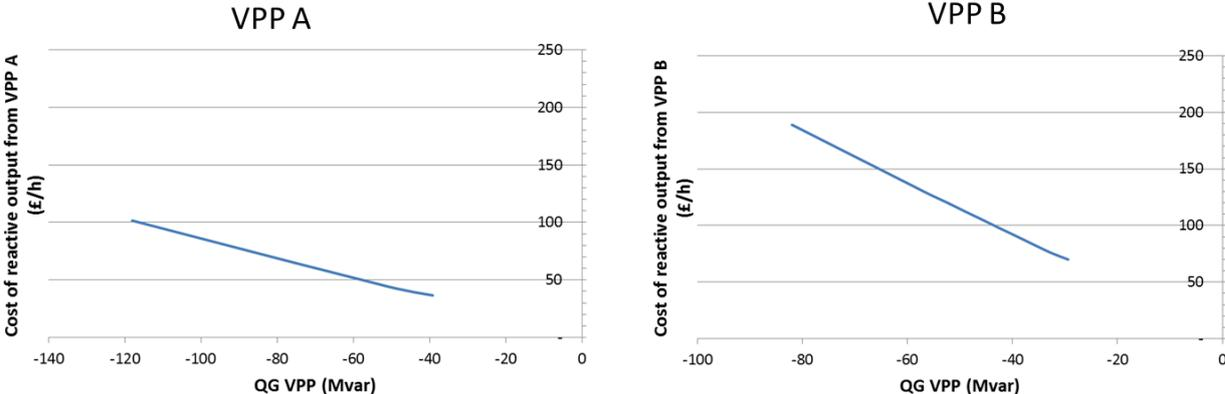
**Figure 2-15 Cost function of reactive power services (absorption) from VPP A and VPP B during minimum demand**
