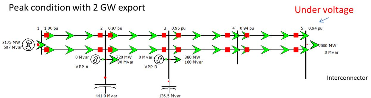
Figure 2-6 An illustrative example showing an under voltage problem during peak load condition with 2 GW export
