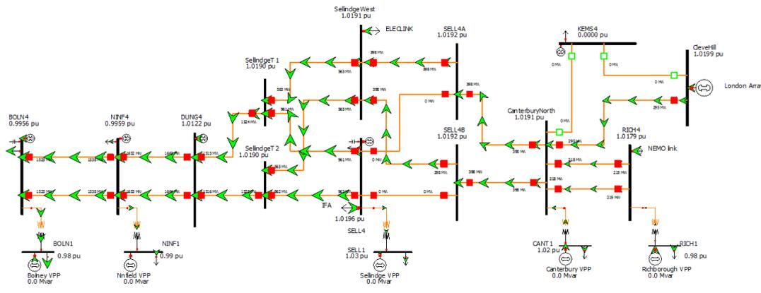
**Figure 4-3 Solving network congestion problem using a combination of the transmission connected generators and VPP**
