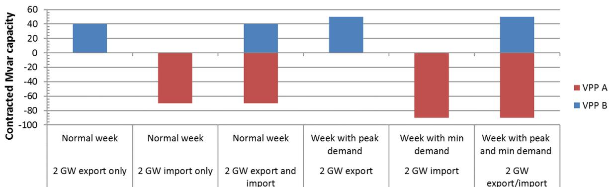
**Figure 2-17 Allocation of reactive power contract to VPP A and VPP B depending on the system conditions forecasted a week ahead**
