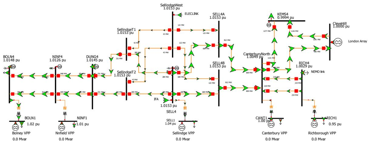
Figure 4-1 South-East GB transmission test system
