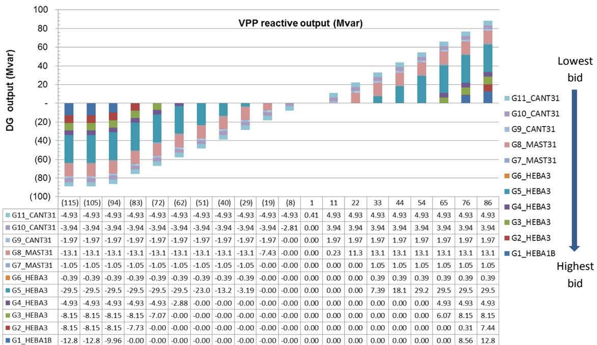
Figure 3-22 Reactive power dispatch of each DER in Canterbury VPP
