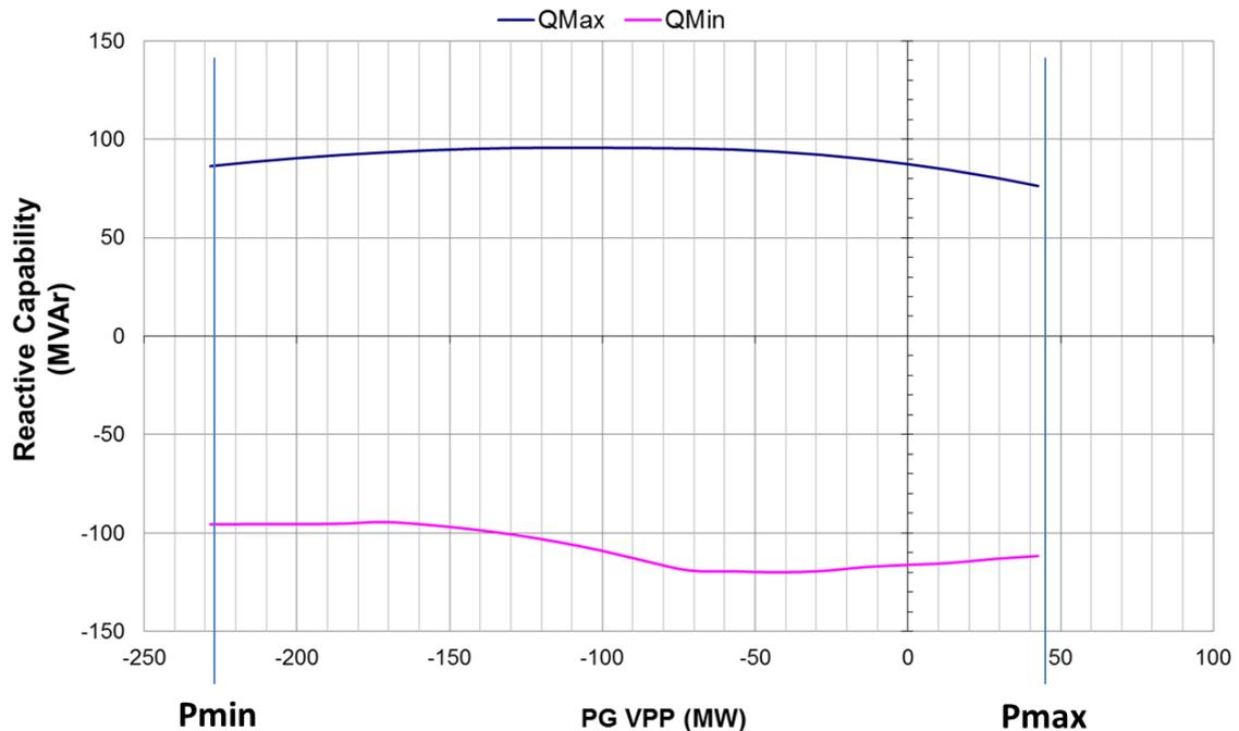
**Figure 3-12 PQ curve of the Canterbury VPP**
