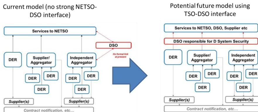
Figure 2-2 A potential future model of TSO-DSO interface<sup>6</sup>
