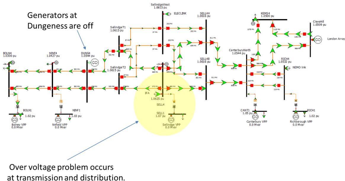
**Figure 4-5 Illustrative case study simulating an over-voltage problem on the test system**
