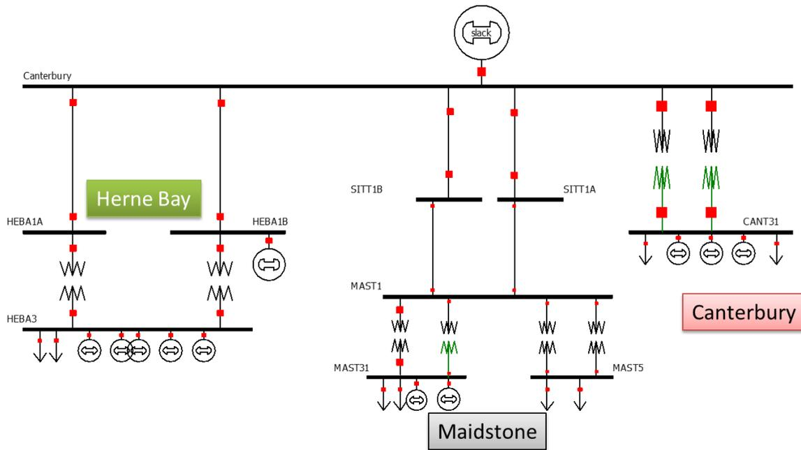
**Figure 3-11 Reduced Canterbury distribution network model**
