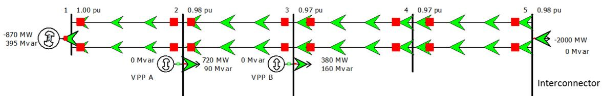
Figure 2-8 An illustrative example showing a normal peak condition with 2 GW import
