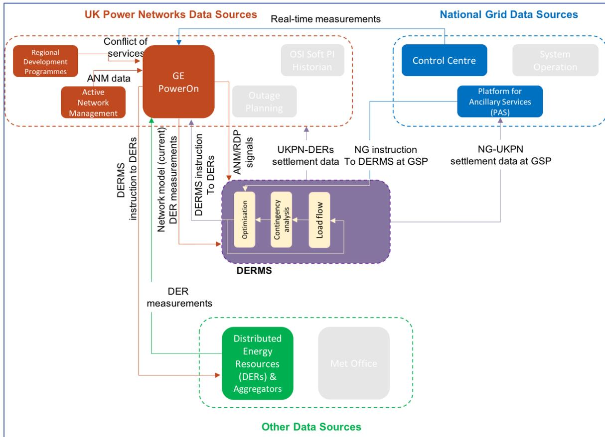
Figure 6: Data exchange in the 'Real time' (Service Mode)
