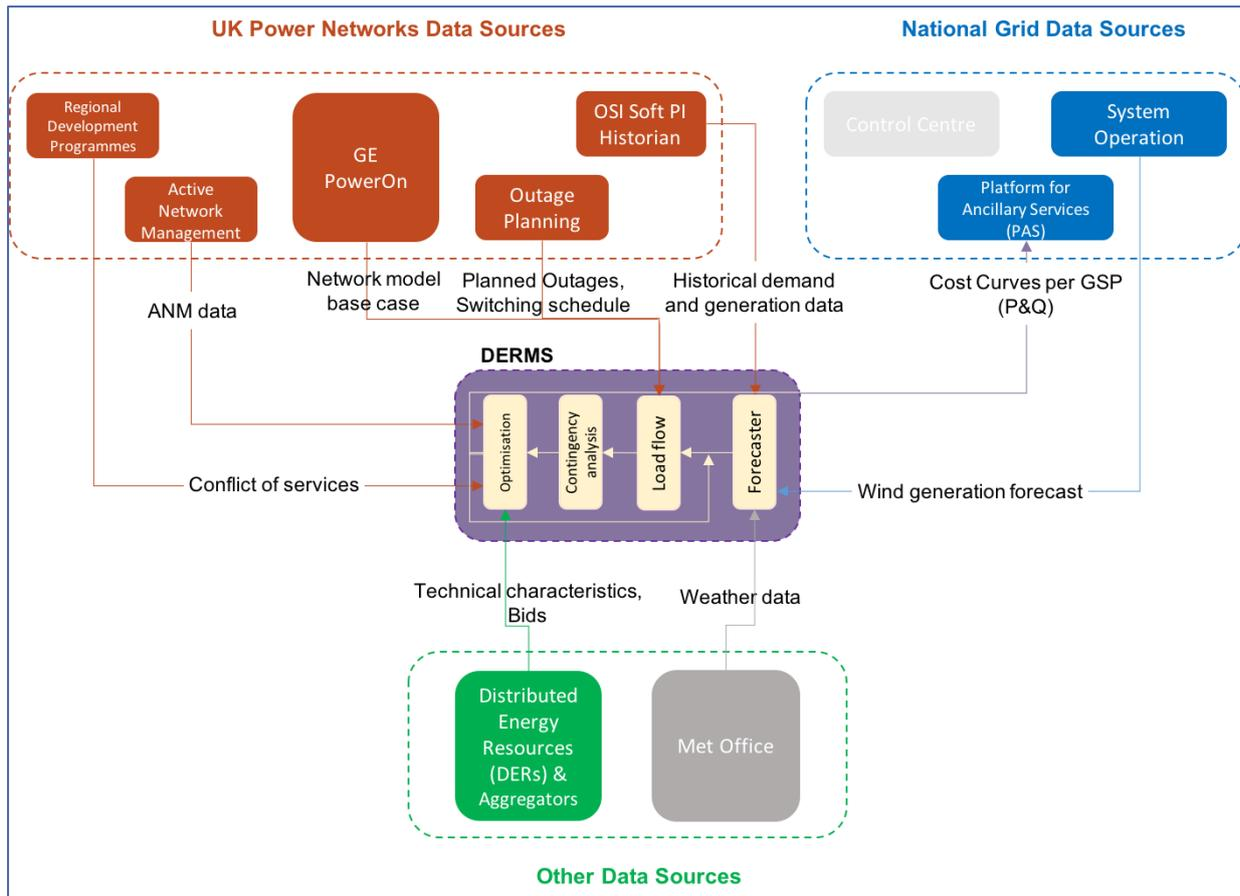
Figure 5: Data exchange in the Future Availability operational horizon (Forecasting and Future Availability modules)
