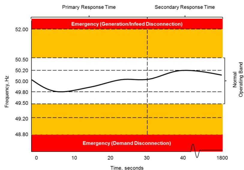
Figure A2 GB System Frequency Limits
