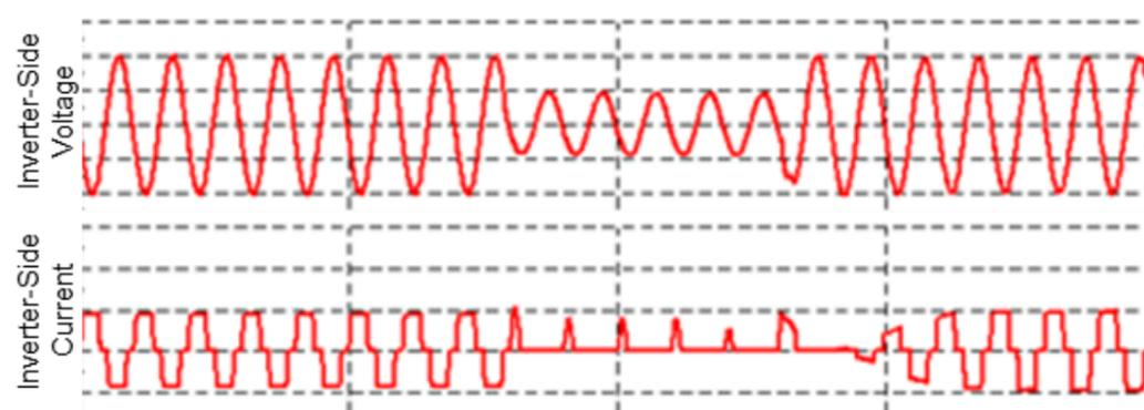
Figure 33 Commutation Failure
