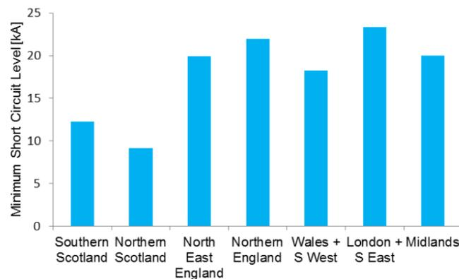
Figure 20 Minimum Short Circuit Level (2014/15)
