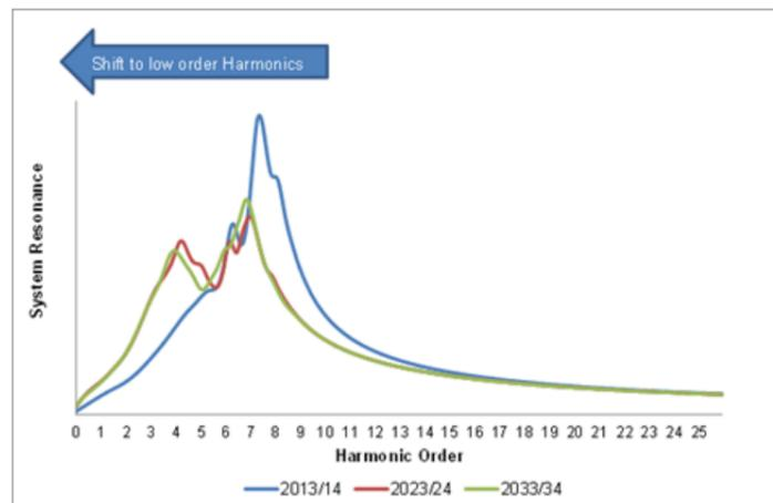
Figure 29 System Resonance Shift to Lower Order Harmonics
