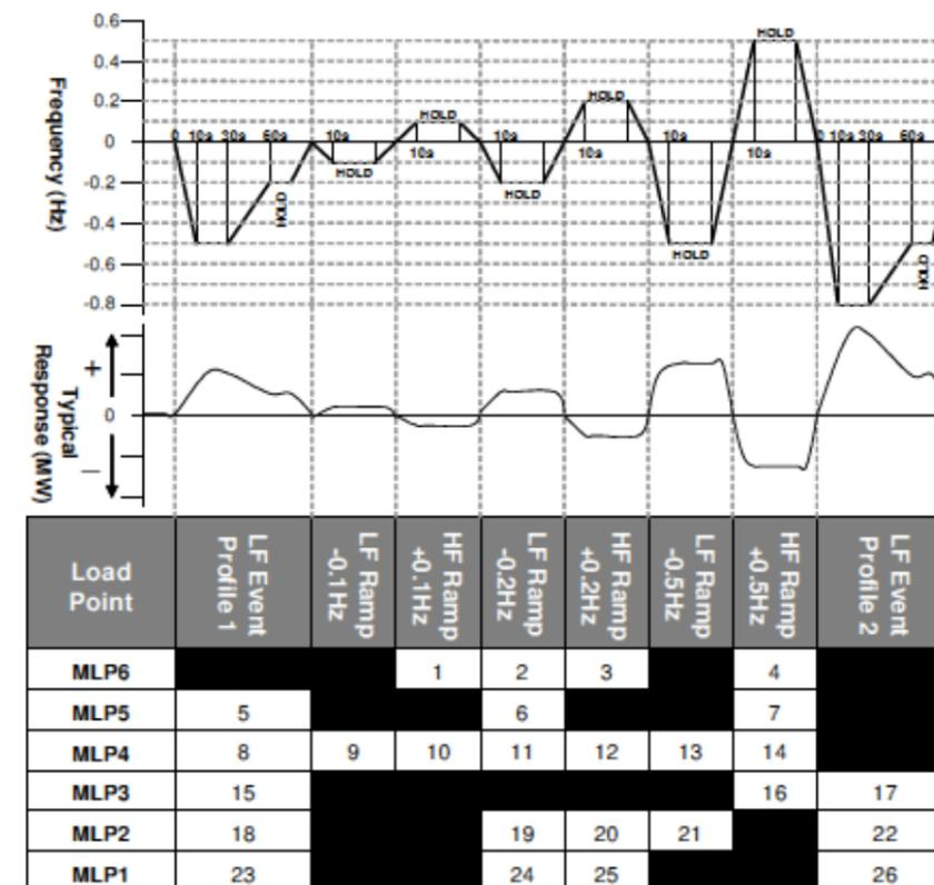
**Figure 18 Frequency Response Capability Test Criteria**
