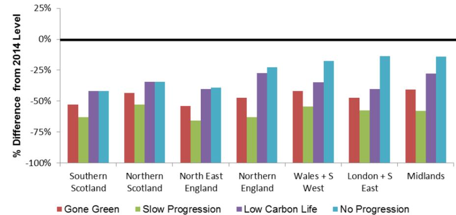
Figure 22 Minimum Short Circuit Level Relative to 2014/15 Level (2034/35)
