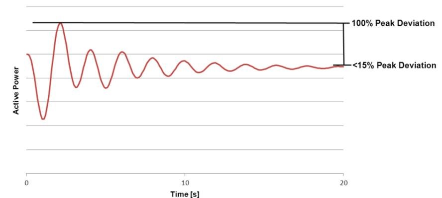
**Figure 16** NETS SQSS Power Oscillation Damping Requirement
