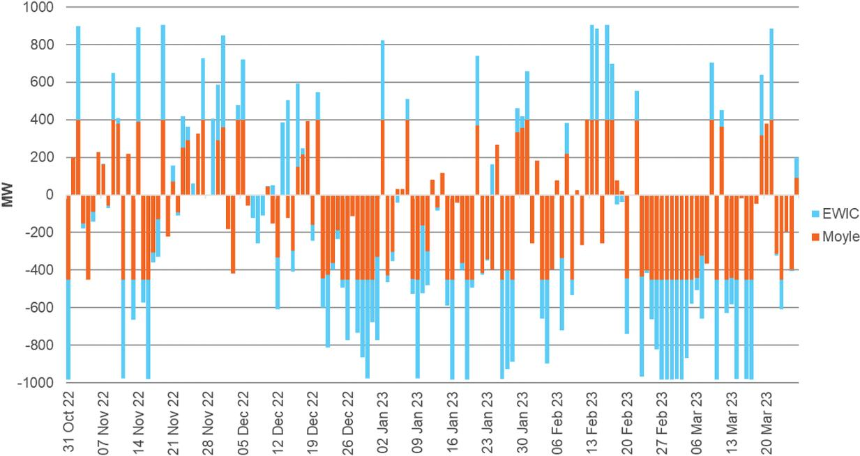
Figure 13: Stacked bar chart showing Moyle and EWIC flows at peak times (positive MW values mean flows into GB)
