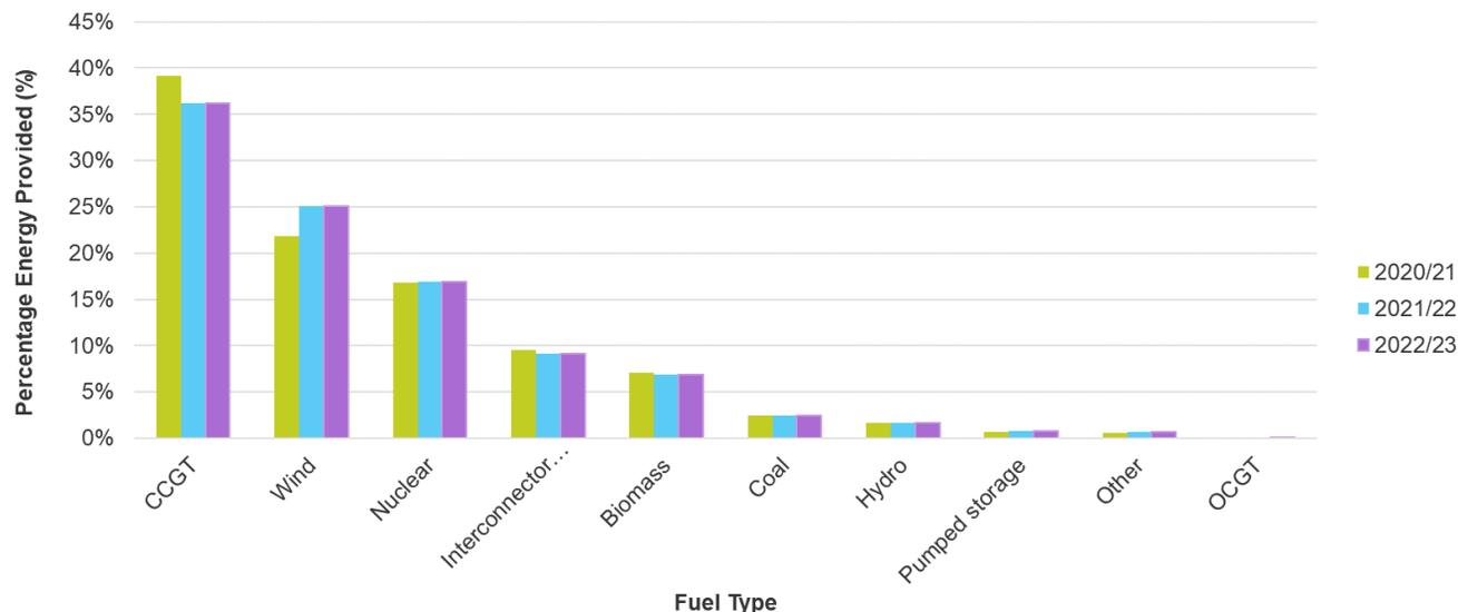
Figure 6: Percentage of electricity provided by each fuel type over Winters 2020/21, 2021/22 and 2022/23 (transmission connected generation only)
