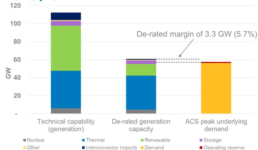
Figure 5. Supply margin in relation to generation capacity and demand for Scenario 1
