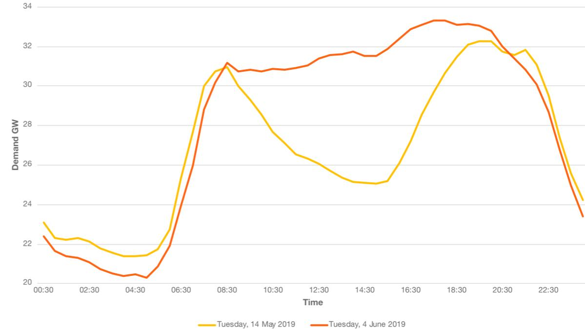
**Figure 4: Impact of embedded solar generation on transmission system demand between two days 3 weeks apart in summer 2019.**
